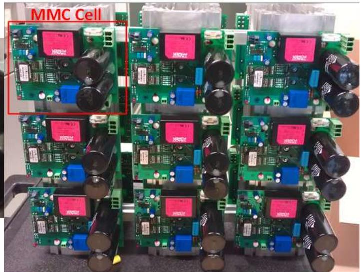
Figure A - 6: Cells on the heatsinks
