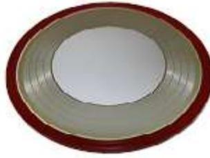
Figure I-31: 4" IGCT (5.5 kA/4.5 kV) (ABB)
