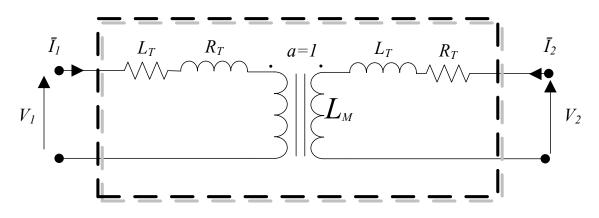
Figure II-15: 2-port model of a transformer
