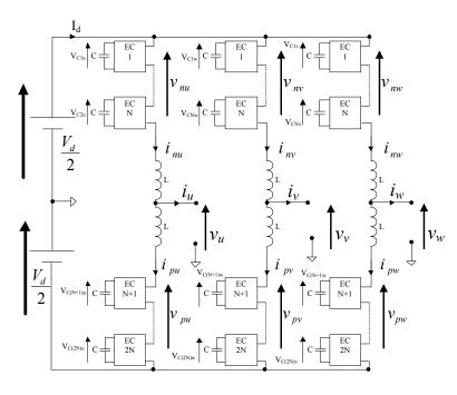
Figure II-1: Modular Multilevel Converter in three-phase configuration
