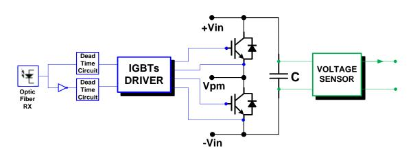
Figure A - 1: Scheme of the elementary switching cell
