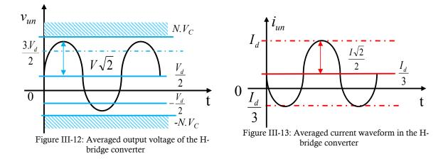
In (74), the current condition's waveform is highlighted in Figure III-12.
