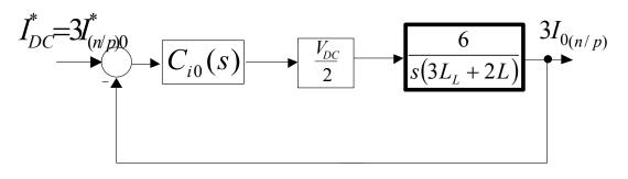
Figure IV-15: Control loop for the 0 component
