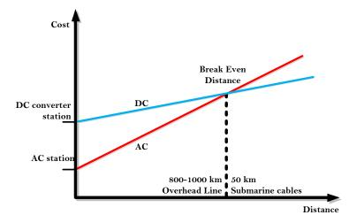
Figure I-1 - Estimation of the coasts for AC and DC transmission
