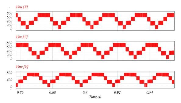
Figure V-10: Voltage imposed by each branch
