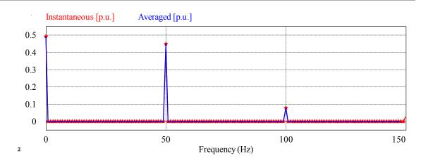
Figure II-7: Spectral content comparison for the output cell voltage
