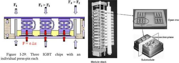
Figure I-30: Pictures of a module stack, an open individual module, and a sub-module inside the module
