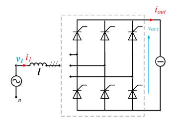
Figure I-36: Rectifier bridge based on phase-controlled thyristors
