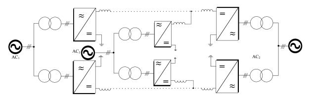
Figure I-13: Multi-terminal connection
