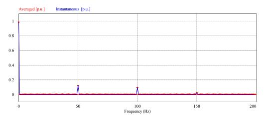
Figure II-5: Spectral content comparison of a capacitor voltage for a cell
