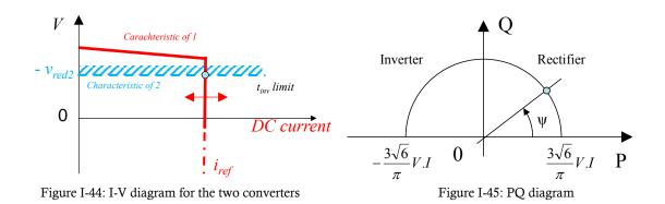
The converter which gets the power and works in inverter mode is depicted in Figure I-46. The converter must regulate the voltage phase angle  $\psi_2$  to operate at the minimum turn-off time  $t_{inv}$  and then limit the reactive power received. As shown in Figure I-44, the operating point is given by the intersection of characteristics for the first converter (in red) and the receiver converter (in blue).
