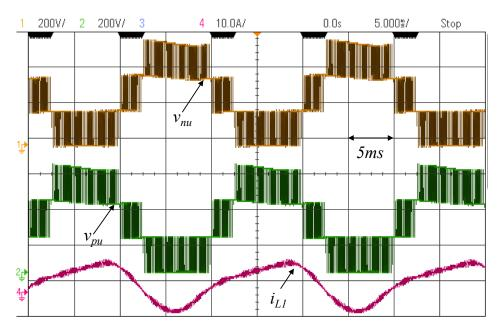
Figure V-25: Negative and positive branch voltages, branch current
