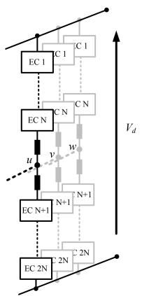
Figure I-62 : Modular Multilevel Converter base schema
