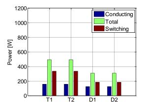
Figure III-19:Cell power losses for MMC in reactive operating mode
