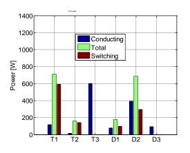
Figure III-20: Cell power losses for MMC in Inverter operating mode
