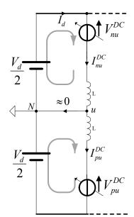
Figure III-3: AC circuit of the MMC structure
