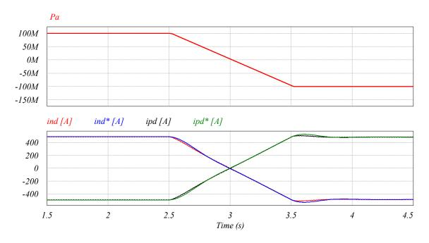
Figure IV-21: Output of the energy balancing controller and direct component of the current for the negative and positive part; power flow
