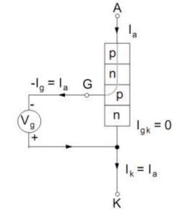
Figure I-33: Lay out in conduction mode for the IGCT
