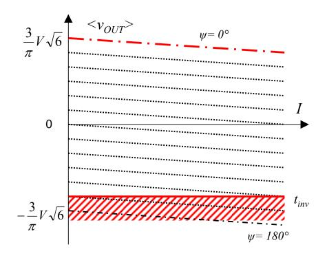
Figure I-41: DC voltage capability vs AC current
