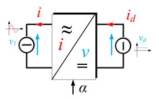
Figure I-47: basic structure for the AC/DC conversion based on VSC systems
