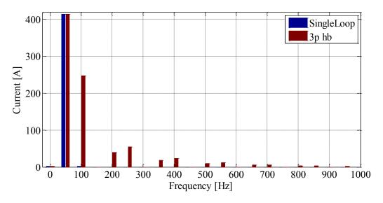
Figure III-34: comparison spectral content of the phase current
