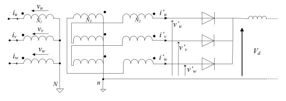
Figure III-30: Three phasehalf bridge rectifier with zigzag transformer.
