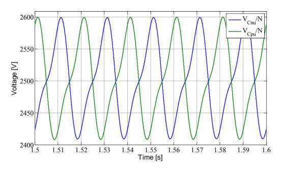
Figure II-29: Voltage capacitor normalized on the number of cells
