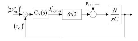
By considering the instantaneous model, the same strategy already described in the previous chapter was adopted to keep a constant voltage of  $2V_{DC}/N$  on each cell capacitor. This because the cell voltage balancing is a parallel loop which depends neither from the current nor from the branch energy balancing loops but it directly interferes on the modulation index. One more time each cell capacitor has 200V voltage.
