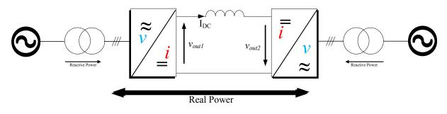
Figure I-3 - CSC-HVDC system base lay out
