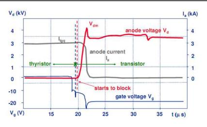
Figure I-35: Typical currents and voltages for a IGCT in turn off mode
