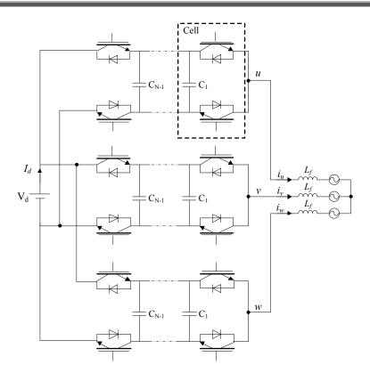
Figure I-59: Three-phase flying capacitor converter
