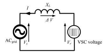
Figure I-50: Single phase Equivalent circuit VSC-HVDC connection
