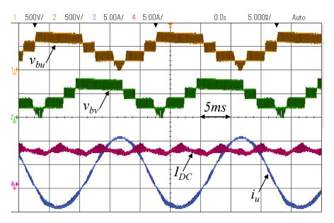
Figure V-13: Branch voltages and currents on DC side and phase u.
