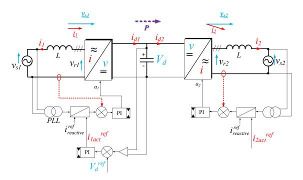
Figure I-55: simple control strategy for a VSC based HVDC connection
