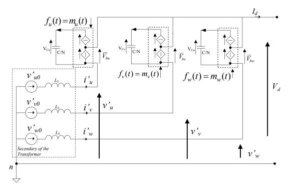
Figure III-29 - Simplified circuit on the AC side with averaged model of the Half Wave multilevel converter
