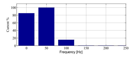
Figure II-26: Spectral content of the branch current in percentage with respect to the fundamental component
