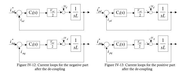
In the dq0 reference frame, the control of the fundamental component means controlling a constant variable in the time domain. Moreover, a second harmonic component due to the circulating currents, treated in the second chapter, has to be suppressed (Figure II-9). In dq0 this component becomes the fundamental one.
