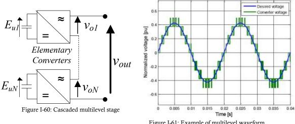
Figure I-61: Example of multilevel waveform
