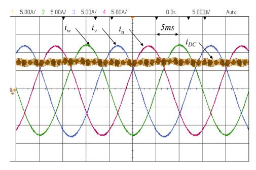
Figure V-23: Output AC currents and DC current
