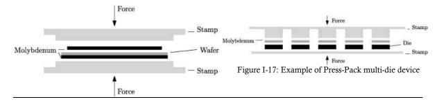
Figure I-16:Cross section of a press-pack single wafer (monolithic)
