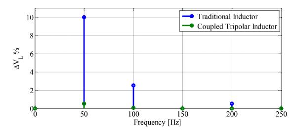
Figure II-27: Comparison of the harmonic content of the voltage drop on the traditional branch inductor of the previous case and the series inductor  $L_T$
