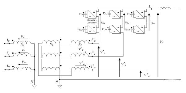
Figure III-28 - Upgraded AC/DC converter
