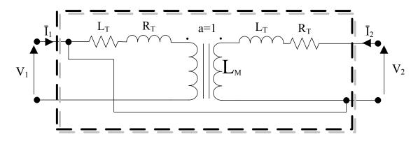
Figure II-16: transformer model in tripolar configuration
