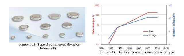
Thyristors can reach very high voltage levels, they are very fast during turn-on and they don't show overvoltage problems in series connection [28]-[22].
