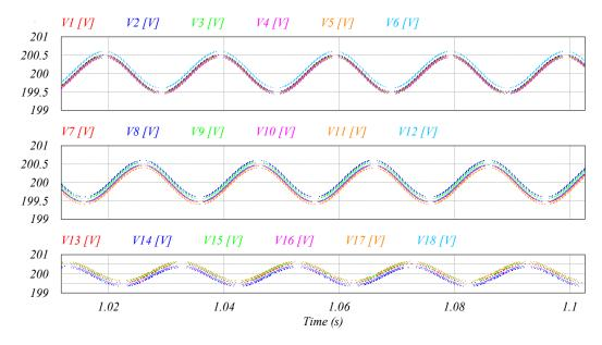
Figure V-12: Voltages on the cell capacitors
