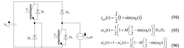
Figure III-25: Asymmetrical H-Bridge employed for the negative branch
