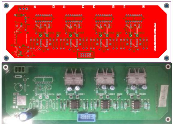
Figure A - 13: Optical emitter layout
