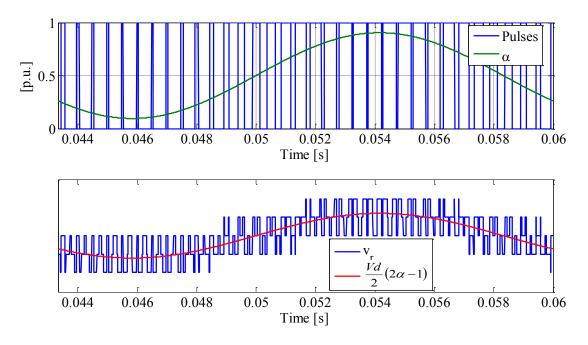
Figure I-49: switch pulses and duty cycle; phase voltage imposed by the converter and its fundamental component waveform
