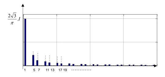
Figure I-40: Harmonic content for a 6 pulse thyristor rectifier
