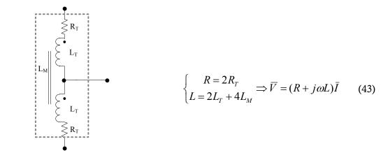
Figure II-17: Equivalent tripolar element of the coupled transformer
