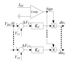
Figure IV-23: Capacitor voltage balancing diagram in a branch
