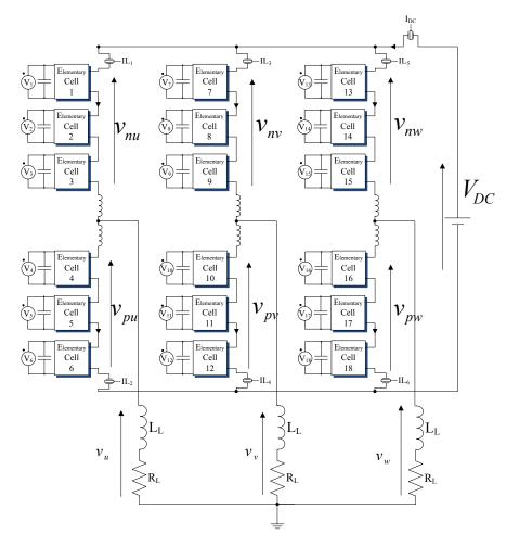
Figure V-20: MMC system configured for the experimental tests
