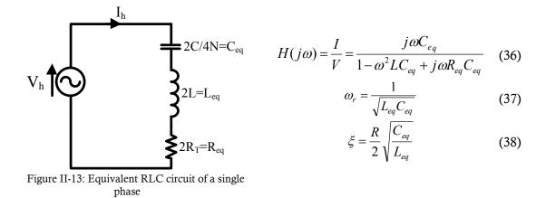
The RLC circuit includes the capacitor, which represents the equivalent capacitance in the phase; then there are the negative and the positive inductors and the resistance, which resumes the dissipative part of the semiconductors and the copper losses. The system is studied like a typical second-order circuit of which the transfer function is (36).
