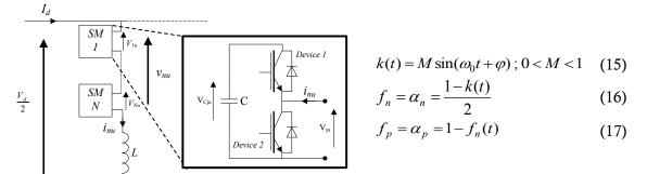
Figure II-8: Simple cell adopted for the MMC structure
