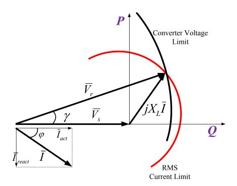
Figure I-54: Fresnel diagram for a AC/DC VSC structure
