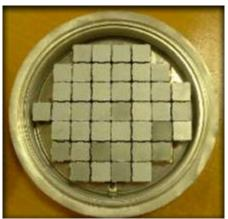
Figure I-27: Westcode internal disposition of a IGBT
