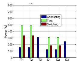
Figure III-22: Cell power losses for MMC in reactive operating mode
