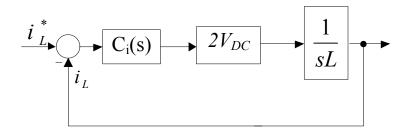
Figure V-9: Current control loop
