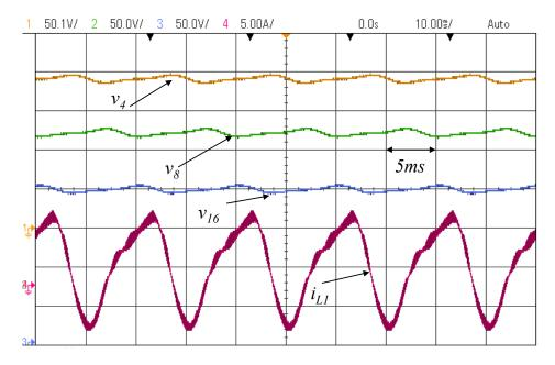
Figure V-27: Capacitor voltages and branch current
