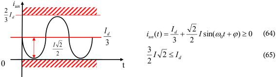
Figure III-9: Averaged current waveform if Asymmetrical H-converter is considered
