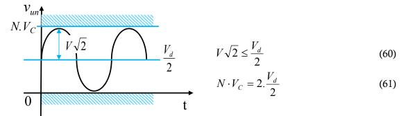
Figure III-6: Averaged voltage waveform if the single cell is considered
