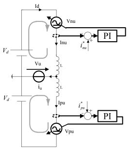
Figure II-11: MMC elementary by imposing each branch current
