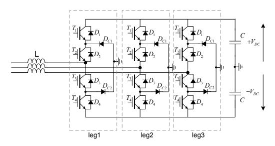
Figure I-58: Three-level three-phase NPC topology
