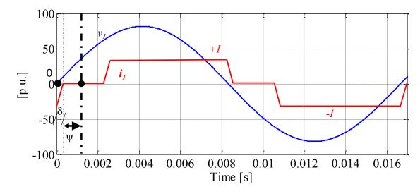
Figure I-39: Typical input current waveform for a 6-pulse rectifier compared with the AC phase voltage
