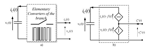
Figure II-2: Low-frequency model b) of an elementary switching cell a)
