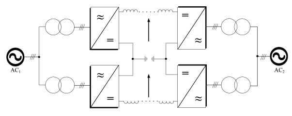
Figure I-12: Bipolar system
