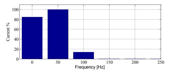
Figure II-21: Spectral content of the branch current in percentage with respect to the fundamental component
