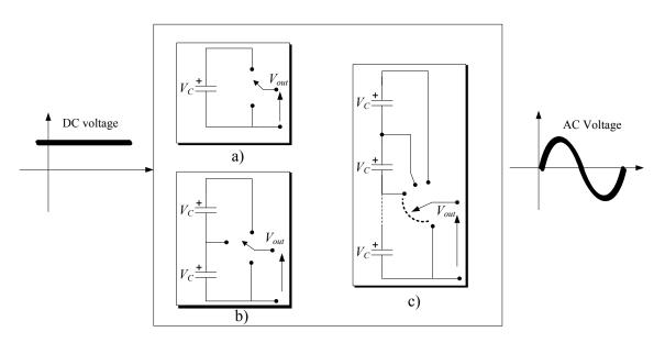
Figure I-56: Basic schema of VSC topologies for a simple one a), 2-VSI b), and a multilevel topology c)
