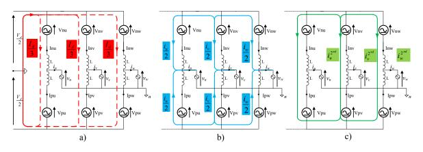
Figure II-9: Current flow in the MMC structure
