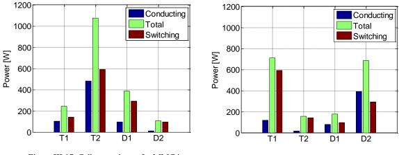
Figure III-17: Cell power losses for MMC in Inverter operating mode
