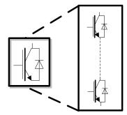
Figure I-8: IGBTs Series connected lay-out
