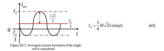
This balance is also necessary to ensure a constant dc voltage across the capacitor. The right power balance also indicates a constant voltage capacitor in the cell and therefore the right energy balance in the branch.
