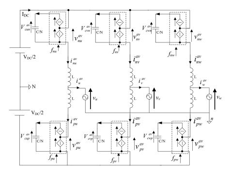
Figure IV-2: Averaged model for a MMC structure
