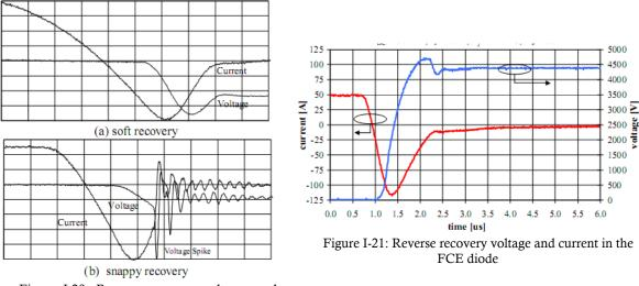
Figure I-20: Reverse recovery voltages and current in the diodes (ABB®)
