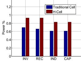
Figure III-23: Increase of the losses for a 3-Phase system by using full H bridge cells respect to a classical system
