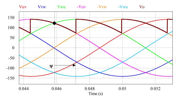
Figure I-37: Line to line voltage waveforms for the 6-pulse converter
