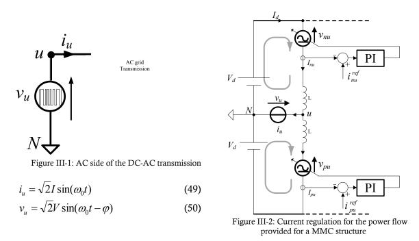
Considerations regarding voltages and currents are given by splitting the circuit in the AC and DC part (principle of superposition). The study is performed only for one phase.
