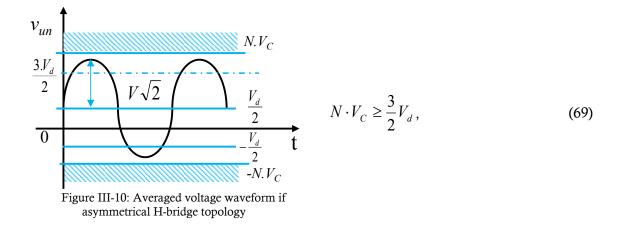
In this case, the voltage level  $NV_c$ , which enables the system to reach the maximum amplitude of the branch voltage, is 1.5 times that of the DC voltage. This means a 50% increase for the number of elementary converters per branch with respect to the employment of the simple cell. On the other hand, considerations on the sizing capacitor make this topology more attractive.
