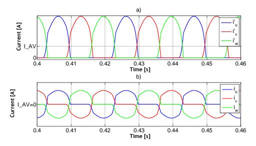
Figure III-31 - AC Current waveforms at secondary side (a) and primary side (b) of the transformer
