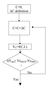
Figure II-12: Iteration method for the capacitor evaluation
