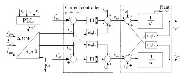
Figure IV-11: Current controller plant in dq0 reference frame for the positive part of the structure
