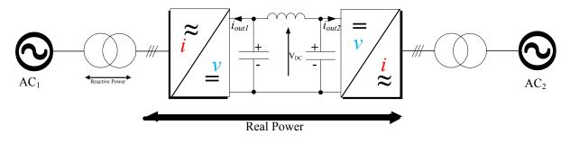
Figure I-6 - VSC-HVDC system base layout
