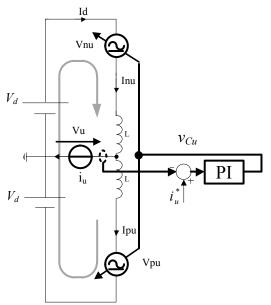
Figure II-10: MMC elementary circuit by imposing the AC output current
