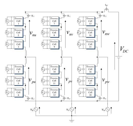
Figure V-16: MMC system configured for the simulations
