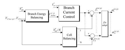
Figure IV-3: SPWM Control approach for a multicellular structure
