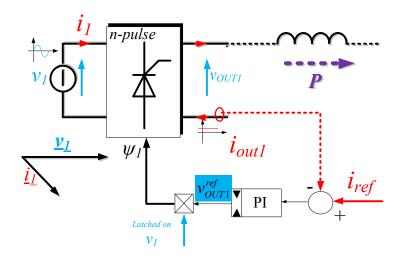
Figure I-43: Basic HVDC connection based on CSC systems
