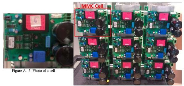
Figure A - 6: Cells on the heatsinks
