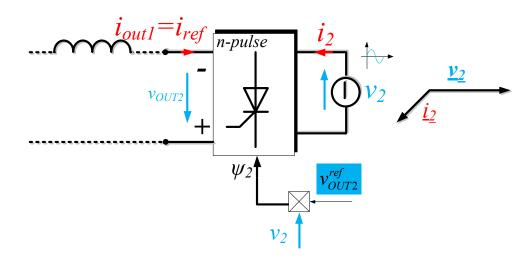
Figure I-46: thyristor converter in inverter operation
