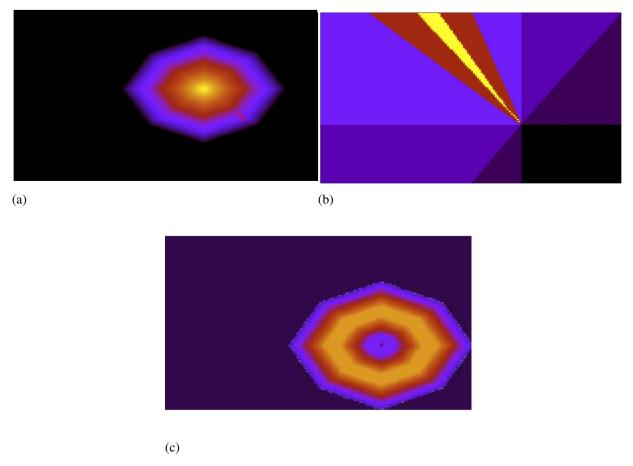
Figure 3.6-(a). Illustration of the target model at a given depth. The colors here indicate the temperature. (b) and (c): application of the bearing only and the range only target detection models. The colors represent here the probability of the target presence (The detection models are represented in a grid structure, see section 3.4).
