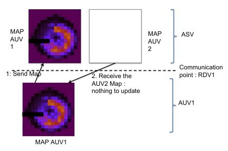
Figure 3.13 – Evolution of the cell probability to contain a source, derived from a map fusion between the AUV1 and the ASV. At the first communication point with the AUV1, AUV1 sends its new map to the ASV, receives the latest map of the AUV2 and updates its map.
