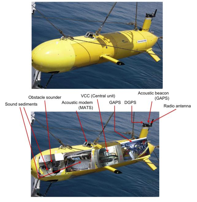
Figure 2.2 – The AUV Asterix used at IFREMER and its components.
