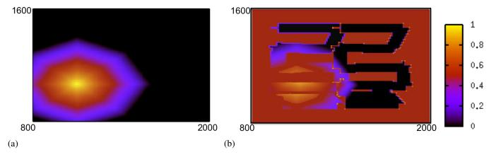
Figure 6.4 – Illustration of a map that results from an exploration strategy of two underwater vehicles using the predefined mission described in figure 6.3. (a) shows the real world. (b) shows the resulting trajectory and the obtained map at the end of the mission execution of both vehicles.
