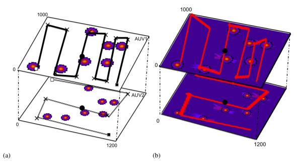
Figure 6.7 – Illustration of the obtained results using two AUVs. Each AUV has a common exploration area and communication points. Figure 6.7a is the predefined path for AUV1 and AUV2. Figure 6.7b represents the obtained path and the constructed map, after execution, for both AUVs.
