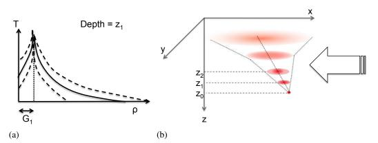
Figure 3.5 – (a). Evolution of the temperature as a function of the horizontal distance  $\rho$  for one depth  $z_1$ .  $G_1$  represents the gap between the hottest temperature and the real position of the target. (b) Illustration of the real target properties propagation at different depths with a steady current.
