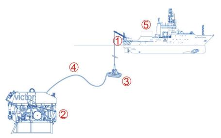
Figure 2.1 – Victor6000, a Remotely Operated Vehicle used at IFREMER. (1) 8500 meters long umbilical of 20 mm diameter a 30 tons weight, (2) the 4 tons vehicle, (3) and (4) a jetsam located within 100 to 300 meters depth, and (5) the 20 feet container that fuels the vehicle with energy.
