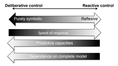
Figure 5.5 – *Illustration of the differences between reactive and delibrative control architectures.*
