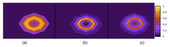
Figure 3.9 – Evolution of the cell probability to contain a source, derived from 3 measures made at the same depth in the environment shown in figure 3.8 – the positions where the measures are taken are denoted by a cross. (a) is the map using one measure and (b) and (c) are the resulting map using two and three measures in order.
