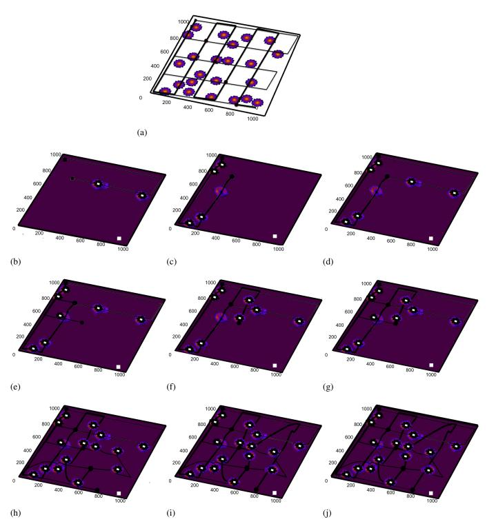
Figure 4.5 – Illustration of two vehicles sharing data for the same area. For the other figures: the left column represents the target detected by the first UAV, the middle column the target detected by the second UAV, and right column the targets detected when merging both maps. Times goes downwards, each line corresponds to a communication point.
