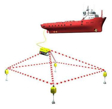
Figure 2.5 – Illustration of the use of LBL with a ROV.
