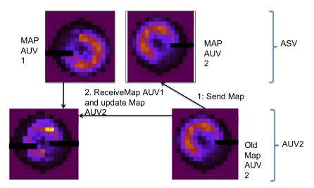
Figure 3.14 – Evolution of the cell probability to contain a source, derived from a map fusion between the AUV2 and the ASV. At the first communication point with the AUV2, AUV2 sends its new map to the ASV, receives the latest map of the AUV1 and updates its map.
