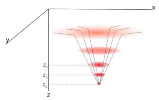
Figure 3.3 – Illustration of the temperature evolution within a thermal plume in stationary waters: the temperature, here represented in red (the redder the hotter), decreases with the elevation and with the distance to the vertical of the emitting vent.
