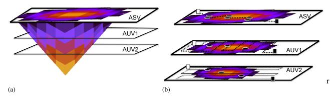
Figure 6.10 – Illustration of the predefined exploration strategy for each underwater vehicle to shape one target. Communication points are represented with black circles and the beginning and end point with white and black rectangle in oder.
