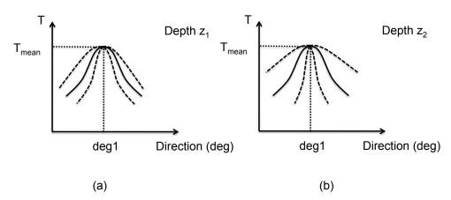
Figure 3.7 – Evolution of the temperature as a function of degrees "deg" for two depths  $z_1$  and  $z_2$  (defined in the figure 3.3).
