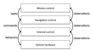
Figure 2.6 – *Illustration of different levels of underwater vehicles' autonomy.*
