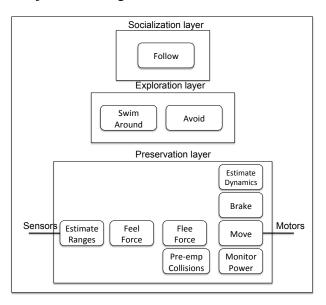
Figure 5.3 – *Illustration of the Eric AUV control architecture*
