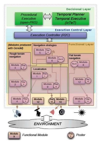
Figure 5.4 – *Illustration of the LAAS architecture [Ingrand07].*
