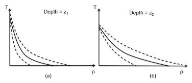
Figure 3.4 – Evolution of the temperature as a function of the horizontal distance  $\rho$  for the two depths  $z_1$  and  $z_2$  defined in figure 3.3. Dashed line represent the dispersion of the temperature.
