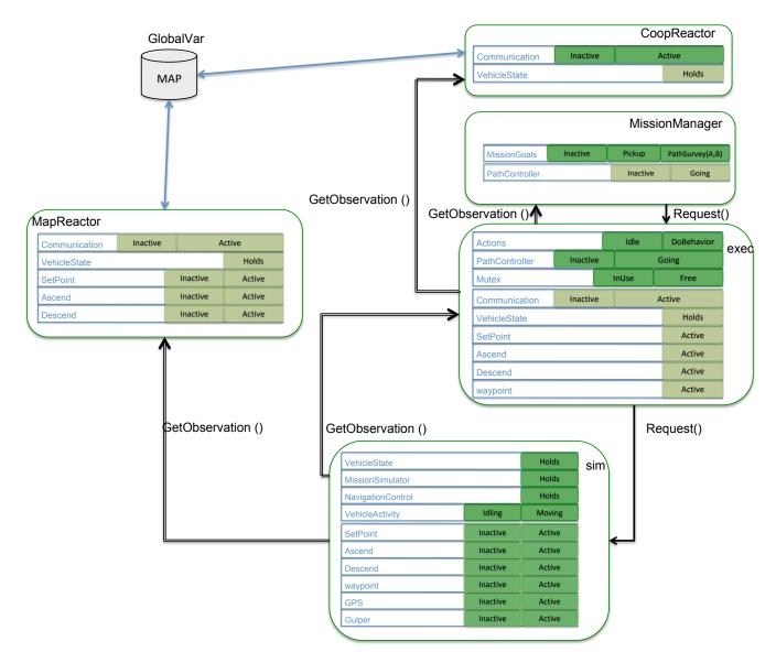
Figure 5.18 – Illustration of different timelines used at each reactor in the T-ReX architecture
