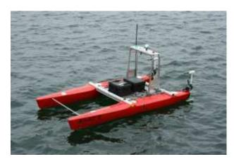
Figure 2.3 – ROAZ II: an autonomous surface vehicle used at LSA's lab
