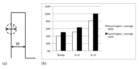
Figure 4.7 – figure 4.7a: Definition of the vehicle sensor range r and the transect width W. figure 4.7b: Illustration of the various strategies percentage of found targets for two different values of coverage percentage.
