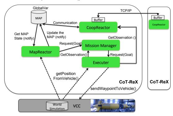
Figure 6.14 – Illustration of the used architecture to link between our implemented T-ReX architecture and the used architecture at IFREMER.
