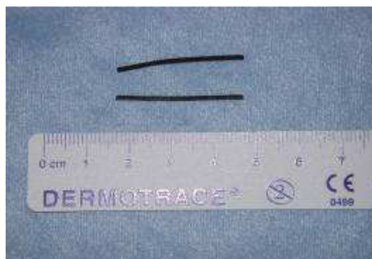
Figure III-26 : Bande fine de plasto-aimants ferrite
