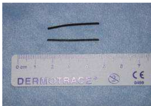
Figure III-26 : Bande fine de plasto-aimants ferrite
