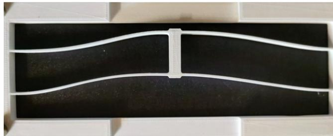
Figure 5.11 – Illustration of the alteration of the initial shape of the beams due to the relaxation of the material three weeks after printing for one of the mechanism used.
