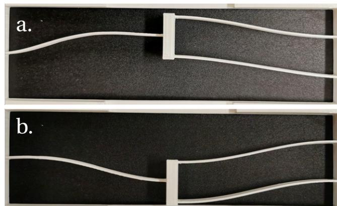
Figure 5.12 – Photograph of an *enhanced* mechanism made with 3D printing in its two stable configurations: a. Fabricated and b. Deformed
