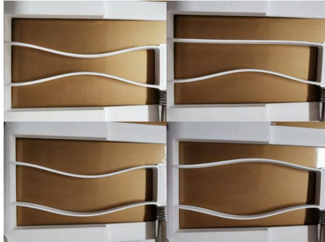
Figure 5.10 – Illustrations of half-mechanisms showing the beams of *classic* bistable mechanisms in various buckling mode.
