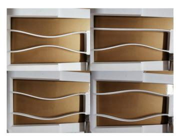
Figure 5.10 – Illustrations of half-mechanisms showing the beams of *classic* bistable mechanisms in various buckling mode.
