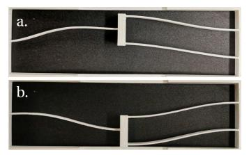
Figure 5.12 – Photograph of an *enhanced* mechanism made with 3D printing in its two stable configurations: a. Fabricated and b. Deformed
