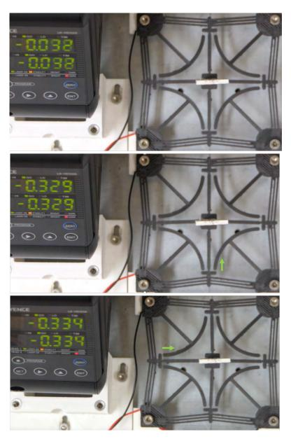
Figure 5.38 – Experimental characterisation of the XY positioning system. The numbers on the dials of the Keyence sensor show the displacement in centimetres. The top image (a.) represents the initial state and the middle (b.) and bottom (c.) images show the amount of displacement in the direction of the arrows in response to an actuation.
