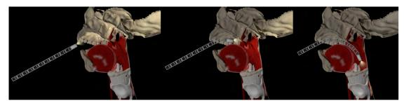
Figure 2.5 - Example rendering of a hyper-redundant robot based on multistable modules.
