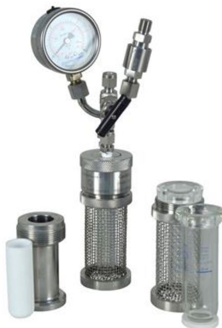
Figure 4. Typical Büchi autoclave used for catalytic experiments under pressure. Left: Teflon cuve. Right: glass cuve. Photo reproduced from the Büchi website ( www.buchiglas.fr )
