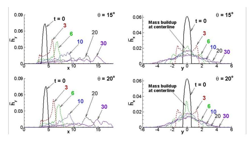
Figure 7-10. Streamwise  $(\bar{h}_x)$  and spanwise  $(\bar{h}_y)$  averages of the mean height  $(\bar{h})$  at t=0,3,6,10,20,30 for  $\theta=5^\circ,10^\circ,15^\circ,20^\circ$ .  $\bar{h}_x$  reveals a mass buildup near the centerline.
