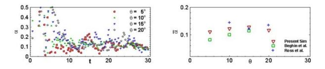
Figure 7-20. (Left) Temporal evolution of the entrainment coefficient  $\alpha$ . (Right) Mean value of  $\alpha$  beyond t=10 as a function of bottom slope  $\theta$ .
