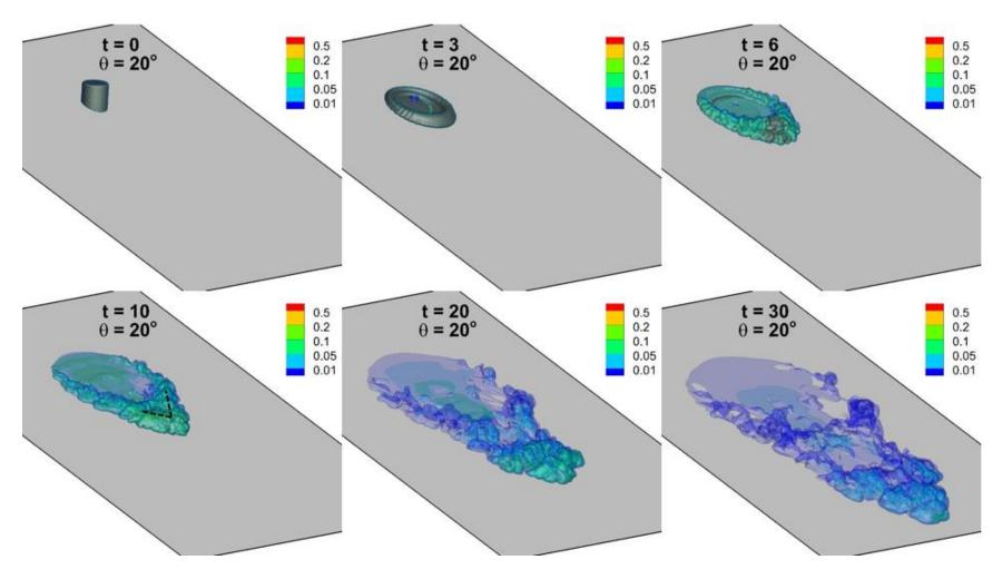
Figure 7-4. Snapshots of the current at various times (t=0,3,6,10,20,30) for various slopes  $\theta=(5^\circ,10^\circ,15^\circ,20^\circ)$ . The current is visualized with multiple semi-transparent iso-surfaces of density with a value of  $\rho=(0.01,0.05,0.1,0.2,0.5)$ .
