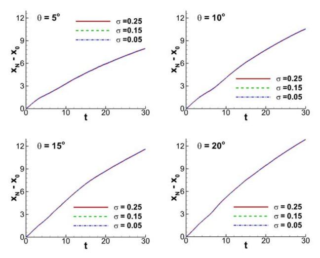
Figure 7-7. Sensitivity of the calculated front position to the segment length  $\sigma$  for a fixed  $\epsilon=10^{-3}$ .
