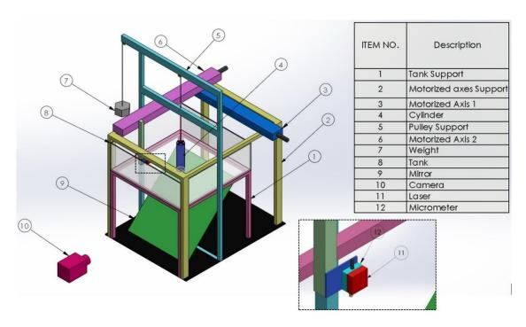
Figure 2-1. Isometric view of experimental setup. For the enlarged view at the bottom right, the tank and the motorized axes support have been hidden to allow for an unobstructed view of the laser.
