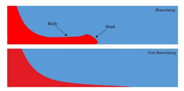
Figure 1-2. Schematic of a Boussinesq (top) and a non Boussinesq (bottom) current.
