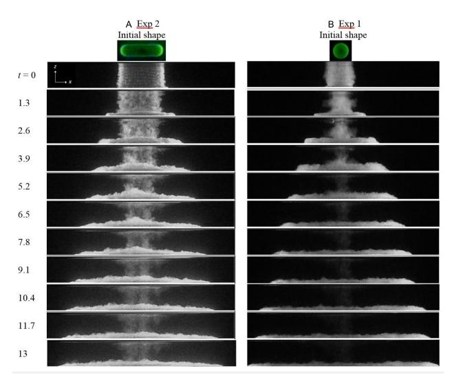
Figure 5-5. Side view of the A) rounded rectangle and B) circular gravity currents.
