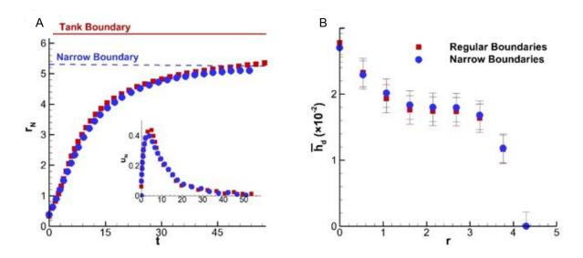
Figure 6-13. A) Front position versus time for Exp 6-1 (squares) and Exp 6-2 (circles) along the minor x-axis. The solid and dashed lines represent the location of the tank lateral wall in Exp 6-1 and 6-2, respectively. Inset: time evolution of the front velocity. B) Corresponding mean final deposition thickness  $\bar{h}_d$ .
