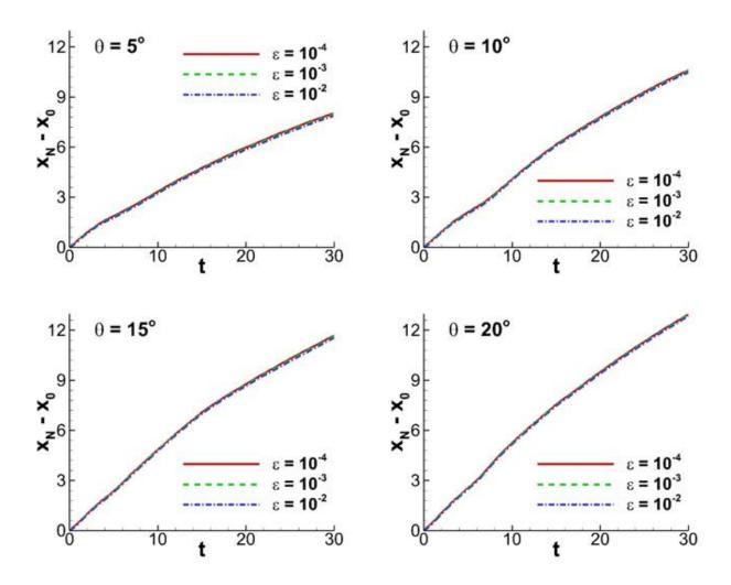
Figure 7-6. Sensitivity of the calculated front position to the small threshold value  $\epsilon$  for a fixed  $\sigma=0.15$ .
