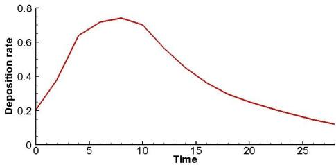
Figure 4-8. Deposition rate versus time at the bottom wall of the domain for Re=10000. The sedimentation rate increases from the time of release, attains a maximum value around t=8 then monotonically diminishes up to the end of the simulation.
