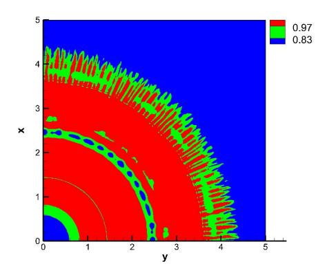
Figure 4-9. Contours of concentration at the bottom wall for Re=10000 in one quadrant of the computational domain at t=6. The large scale vortex tubes transport low concentration fluid (particle-laden fluid mixed with the ambient) from the top of the current towards the bottom wall resulting in a local minimum around r=2.5.
