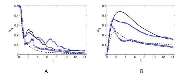
Figure 3-5. Temporal evolution of the local front's height A) and speed B) in the vertical mid-plane of x-direction (dashed lines) and y-direction (solid lines) of the current of initial rounded-rectangle cross section for two initial depth ratios, namely a partial-depth release  $h_0 = H/2$  (blue lines with symbols) and a full-depth release  $h_0 = H$  (black lines without symbols). These results are obtained from fully-resolved simulations with  $H/R_0 = 2$  and Re = 8950.
