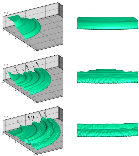
Figure 4-3. Iso-surfaces of density in one quadrant of the computational domain for Re=10000. The structure of the current exhibits multiple rolled-vortices with the lobe and cleft instability pattern identifiable at later times (t=6). An isovalue of  $\rho=0.25$  is employed for all cases. A close up view of the front (on the right) shows its transition from a nearly two-dimensional surface at early times (t=2) to a more complex structure at later times(t=6)
