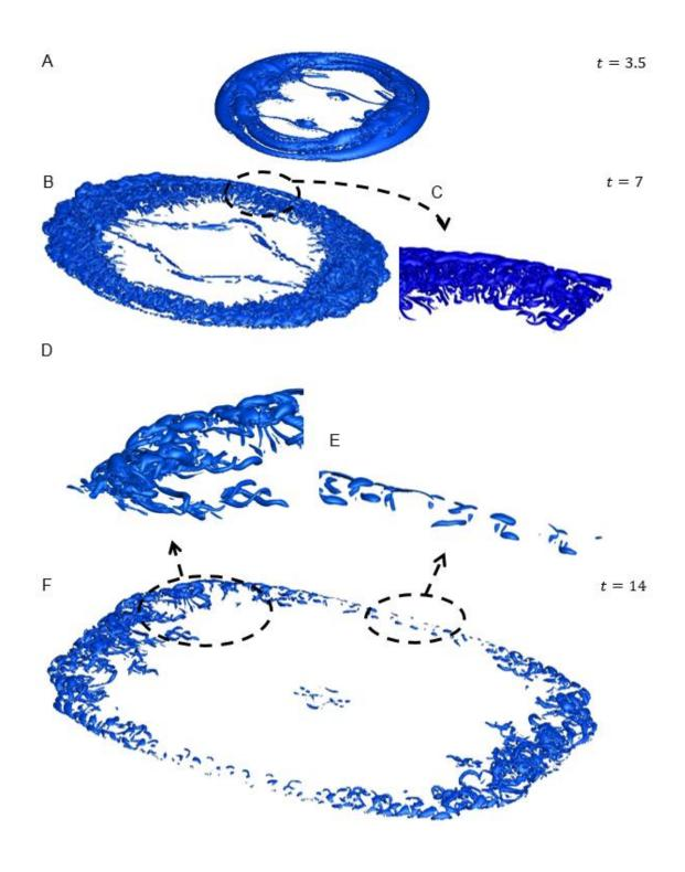
Figure 5-16. Isosurfaces of  $\lambda_{ci}=2$  for the RR release (Sim 5-1) for t=3.5,7, and 14. The vortical tubes are stretched and twisted before eventually breaking down into smaller structures.
