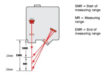
Figure 2-3. Measuring range of laser.
