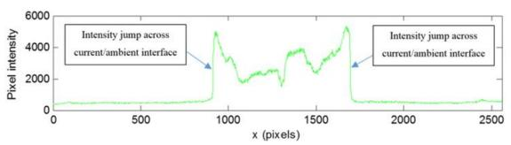
Figure 2-4. The large pixel intensity jump across the interface (close to an order of magnitude) allows the front to be easily identified.
