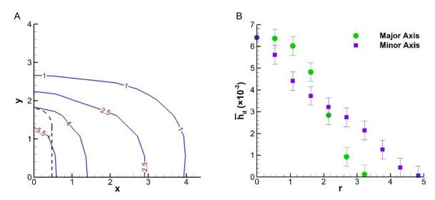
Figure 6-10. A) Iso-contours of the mean deposition thickness  $\bar{h}_d$  of the  $\phi_0=0.13$  -turbidity current (Exp 6-6). The dashed line represents the boundaries of the hollow cylinder. Values of  $\bar{h}_d$  are given in percent. B) Corresponding mean final deposition thickness versus radial distance along the major *y*-axis (circles) and minor *x*-axis (squares). The bars correspond to the measurement error.
