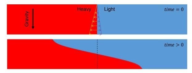
Figure 1-1. Conditions leading to the formation of a gravity current. At time = 0, a hydrostatic pressure difference is present at the vertical interface. It increases linearly with depth, reaching a maximum at the bottom surface.
