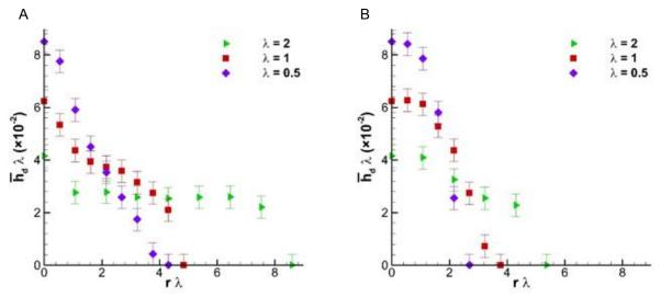
Figure 6-12. Mean final deposition thickness  $\bar{h}_d$  versus radial distance for various initial height aspect ratio  $\lambda$  along A) the minor x-axis and B) the major y-axis:  $\blacklozenge$ ,  $\lambda$ =0.5 (Exp 6-10);  $\blacksquare$ ,  $\lambda$ =1 (Exp 6-3);  $\blacktriangleright$ ,  $\lambda$ =2 (Exp 6-1). The bars correspond to the measurement error.
