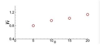
Figure 7-14. Mean Froude number as a function of bottom inclination. The Froude number is observed to increase linearly with bottom slope.
