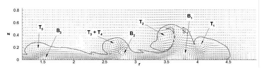
Figure 4-12. Velocity field in a plane passing through the center of the domain at t=6 for Re=10000 case. The current layout is visualized by a density contour of  $\rho=0.05$ . The top (resp. bottom) vortices rotate with a counter-clockwise (resp. clockwise) direction.
