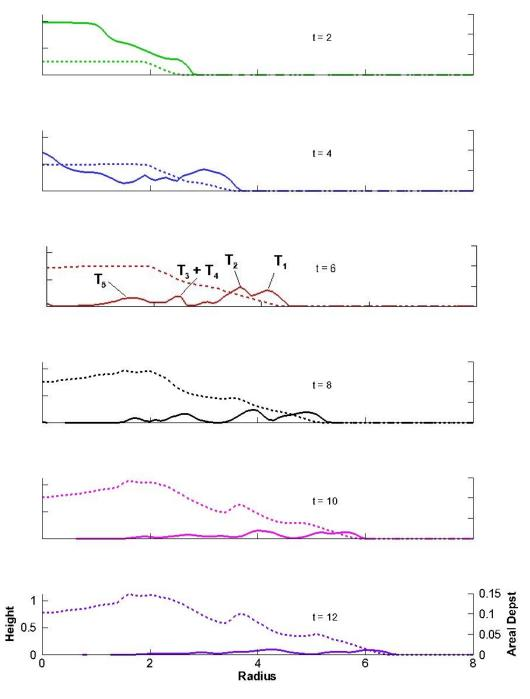
Figure 4-5. Height (solid line) and areal deposit (dashed line) as a function of radius for different times with Re=10000. The four peaks in the height profile at t=6 correspond to the Kelvin-Helmholtz vortices shown in Figure 4-3.
