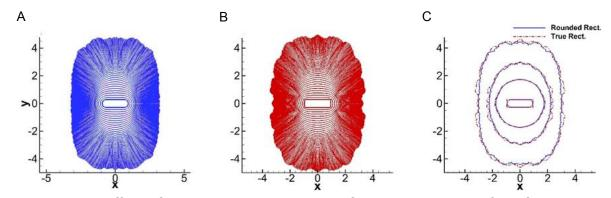
Figure 5-15. Effect of the local initial curvature. Composite picture of the front evolution obtained from simulations. Time separation between fronts is  $\Delta t = 0.35$  and the final run time is t = 16.1 A) rounded rectangle (Sim 5-1); B) true rectangle (same physical parameters as Sim 5-1); C) comparison between the two geometries at t = 0, 3.5, 7, and 14.
