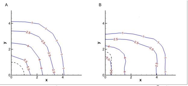
Figure 6-5. Iso-contours of the dimensionless mean deposition thickness  $\bar{h}_d$  of a turbidity current of initial A) circular cross-section (Exp 6-7) and B) non-circular cross-section (Exp 6-3). The dashed lines represent the boundaries of the hollow cylinders. Values of  $\bar{h}_d$  are given in percent.
