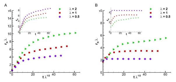
Figure 6-11. Front position versus time for currents of various initial height aspect ratio  $\lambda$  along A) the minor x-axis and B) the major y-axis:  $\bullet$ ,  $\lambda$ =0.5 (Exp 6-10);  $\blacksquare$ ,  $\lambda$ =1 (Exp 6-3);  $\triangleright$ ,  $\lambda$ =2 (Exp 6-1).
