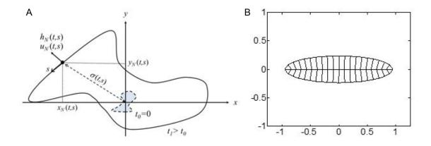
Figure 5-8. A), Notations used for the two-dimensional extended box model.  $\{x_N(s,t),y_N(s,t)\}$  denote the local position,  $h_N(s,t)$  the height,  $u_N(s,t)$  the outward normal velocity of the front and  $\sigma(s,t)$  the area per arc length. The independent variables s and t denote the curvilinear coordinate along the front and time, respectively. B), Example of initial partitioning of the initial elliptical body of a non-axisymmetric gravity current.
