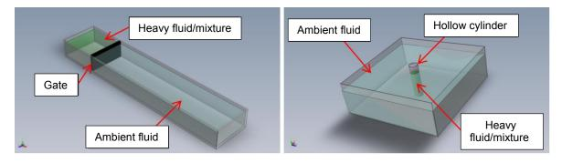
Figure 1-3. Canonical setups: Planar release (left), circular release (right).
