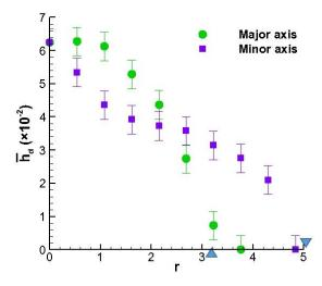
Figure 6-7. Mean final deposition thickness  $\bar{h}_d$  versus radial distance along the minor x-axis (squares) and major y-axis (circles) for the RR-turbidity current (Exp 6-3). The bars correspond to the measurement error. The upward (downward) triangles indicate the location of the critical radius of the front  $r_c$  along the minor (major) axis (Figure 6-5 for details).
