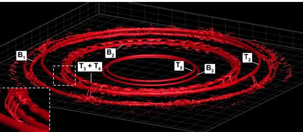
Figure 4-4. Iso-surfaces of  $\lambda_{ci}$  for Re=10000 with an isovalues of 6 and 8 for t=4 and t=6, respectively. The mean and rms values of  $\lambda_{ci}$  are (0.14, 0.79) for t=4, and (0.28, 1.62) for t=6. A close-up view at t=6 shows a set inclined hairpin vortical structures that have formed around the bottom clockwise rotating vortex  $B_2$  in the body of the current.
