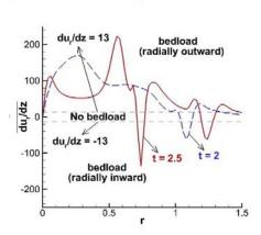
Figure 6-20. Snapshots of  $\overline{du_r/dz}$  from Sim 6-1 at t=2 (dashed line) and t=2.5 (solid line). The thin dashed horizontal lines corresponding to  $\overline{du_r/dz}=\pm 13$  separate three regions: (i) No bedload transport ( $|\overline{du_r/dz}| \le 13$ ), (ii) potential for radially outward bedload transport ( $\overline{du_r/dz} > 13$ ), (iii) potential for radially inward bedload transport ( $|\overline{du_r/dz}| < 13$ ).
