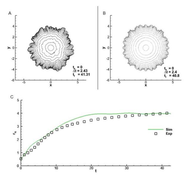
Figure 6-15. Temporal evolution of the front of a circular turbidity current: A) Exp 6-10; B) Sim 6-1. The contours are plotted from  $t=t_0$  to  $t=t_f$  by steps of  $\Delta t$ . C) Azimuthally averaged radial location of the front versus time for Exp 6-10 (symbols) and Sim 6-1 (solid line).
