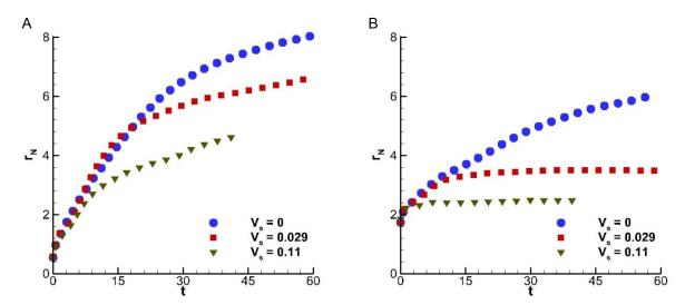
Figure 6-8. Front position versus time for currents of various settling velocity  $V_s$  along A) the minor x-axis and B) the major y-axis:  $\bullet$ ,  $V_s$ =0 (Exp 6-4);  $\blacksquare$ ,  $V_s$ =0.029 (Exp 6-3);  $\blacktriangledown$ ,  $V_s$ =0.11 (Exp 6-5).
