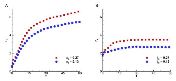
Figure 6-9. Front position versus time for various initial volume fraction  $\phi_0$  along A) the minor *x*-axis and B) the major *y*-axis:  $\bullet$ ,  $\phi_0 = 0.13$  (Exp 6-6);  $\blacksquare$ ,  $\phi_0 = 0.27$  (Exp 6-4).
