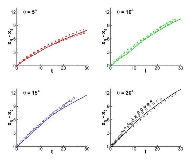
Figure 7-8. Front position as a function of time. The solid line is from the present simulations, and the symbols are from the experiments of Ross *et al.* (2002).
