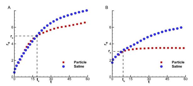
Figure 6-6. Front position  $r_N$  versus time for the RR-turbidity current (Exp 6-3, squares) and the RR-saline current (Exp 6-4, circles) along A) the minor x-axis and B) the major y-axis. The vertical (horizontal) dashed line corresponds to the critical time  $t_c$  (location  $r_c$ ) beyond which the saline front progressively deviates from the particle-laden front.
