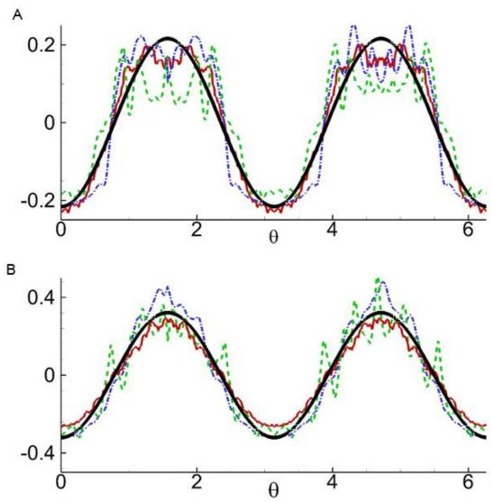
Figure 5-12. (Colour online) Azimuthal evolution at the final time of the scaled front location (red solid), speed (green dashed), and height (blue dash dot) from A) Sim 5-1 ( $\chi_0=3.8$  and B) Sim 5-3 ( $\chi_0=8$ ). The thick solid black line corresponds to  $f(\theta)$  from Eq. (5-22). The mean value is subtracted from each curve.
