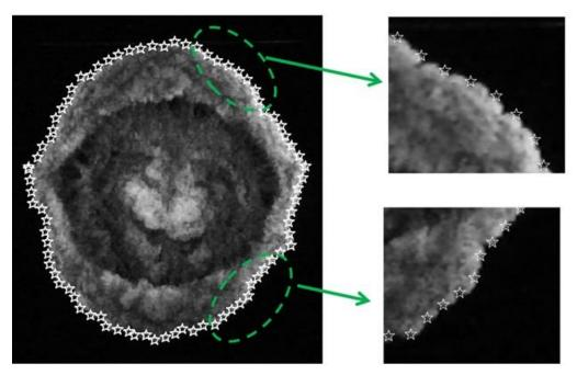
Figure 5-2. Example of front location detection from experiments. A plan view of the current (Exp 5-2 at t=5.9) is shown on the left along with the white star symbols corresponding to the extracted front location. A close up view on the right shows good agreement between the extracted and the actual front location.
