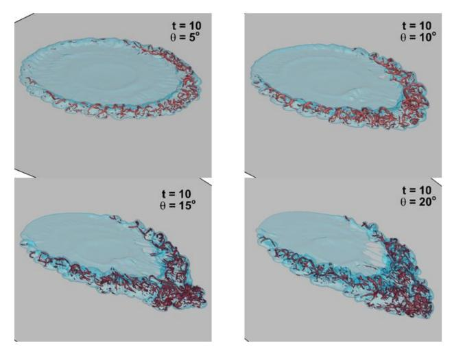
Figure 7-5. Snapshots of the current at t=10 for various slopes  $\theta=(5^\circ,10^\circ,15^\circ,20^\circ)$ . The current is visualized with a semi-transparent iso-sufaces of density with a value of  $\rho=0.05$ . The vortical structures in the interior of the current correspond to iso-surfaces of the swirling strength  $\lambda_{ci}=(3.5,3.5,4.5,5)$  for  $\theta=(5^\circ,10^\circ,15^\circ,20^\circ)$ , respectively.
