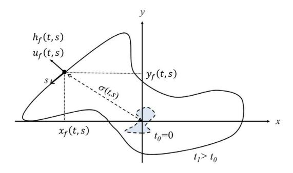
Figure 2-7. Schematic of extended box model.  $(x_f(s,t),y_f(s,t))$  denote the local position,  $h_f(s,t)$  the height,  $u_f(s,t)$  the outward normal velocity of the front and  $\sigma(s,t)$  the area per arc length. The independent variables s and t denote the distance measured along the circumference of the front and time, respectively.
