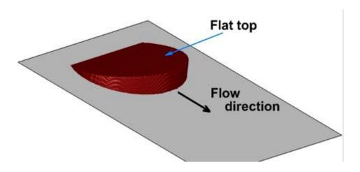
Figure 7-1. Schematic of the shallow water model of Webber et al. (1993).
