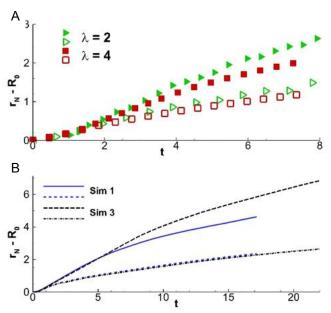
Figure 5-14. (Colour online) A) Time evolution of the fast front (solid symbols) and slow front (open symbols) of a RR release of initial vertical aspect ratio ( $\triangleright \triangleright$ )  $\lambda = 2$ , Exp 5-2 and ( $\square \triangleright$ )  $\lambda = 4$ . Exp 5-5. B) Time evolution of the fast and slow fronts of a RR release of initial horizontal aspect ratio (blue lines)  $\chi_0 = 3.8$ , Sim 5-1 and (black lines)  $\chi_0 = 8$ , Sim 5-3.
