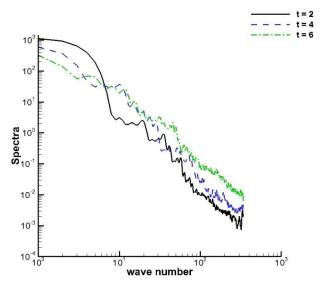
Figure 4-2. Density Spectra as a function of wavenumber along the x-direction for three different time instances at Re = 10000.
