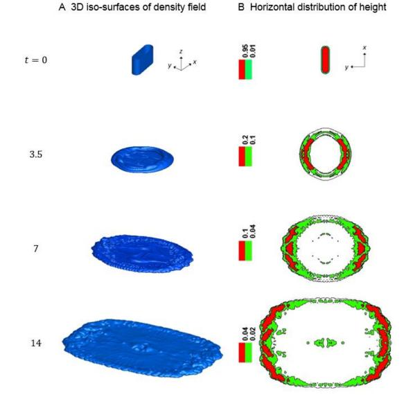
Figure 5-6. Height of the RR-gravity current (Sim 5-1). A) Iso-surfaces  $\rho=10^{-2}$ , B) Distribution of the height along the horizontal plane. Note that the local height strongly varies along the circumference of the current, being maximum along the y-direction.
