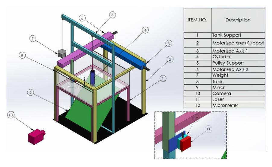
Figure 6-1. Isometric view of the experimental setup. Inset: close-up view of the apparatus used to measure the deposit height. Note that for clarity, the tank and the motorized axes support have been removed from the picture in the inset.
