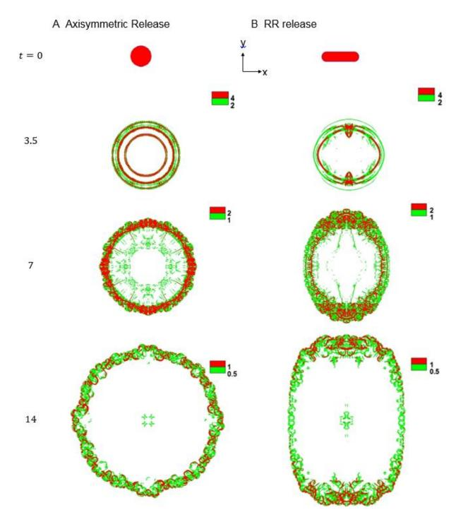
Figure 5-17. Vertically averaged  $\lambda_{ci}$  over the height of the current: A) axisymmetric release (Sim 5-2), B) RR release (Sim 5-1). The initial volume of the current is the same for both cases.
