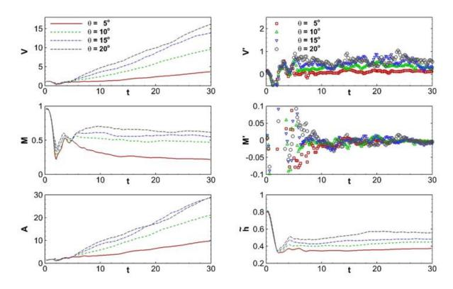
Figure 7-16. Temporal evolution of the volume V, mass M, wall-normal projected area A, mean height of the head  $\tilde{h}$ , and the time rates of change V' and M' of the volume and mass, respectively.
