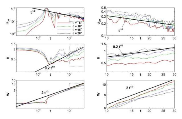
Figure 7-18. Log log plots of the speed of the center of mass  $(u_{CM})$ , maximum height (H), and maximum width (W) in the head as function of time for  $\theta=5^{\circ},10^{\circ},15^{\circ},20^{\circ}$ . A blown up view, corresponding to the dashed rectangle is shown on the right hand side.
