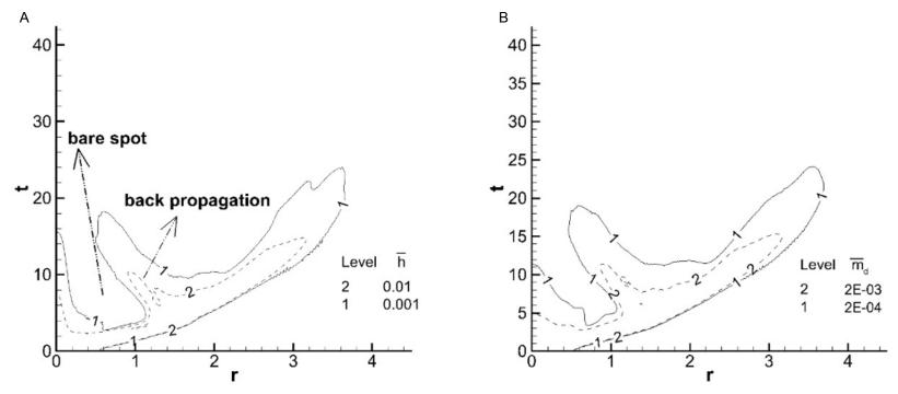
Figure 6-18. A) Contours in space and time of the azimuthally averaged height of the current for Sim 6-1. Flow reversal is observed around r=1.2 and t=4.5. B) Contours in space and time of the azimuthally averaged, instantaneous mass deposition rate of particles per unit area for Sim 6-1.
