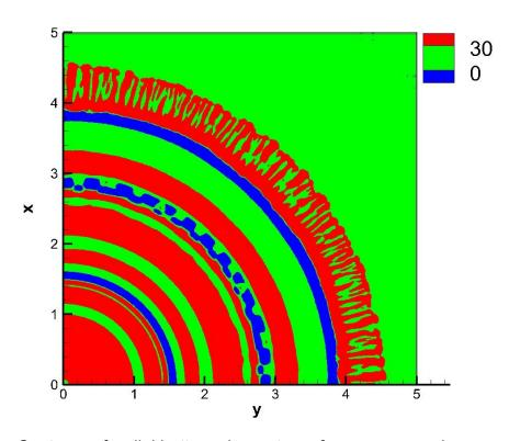
Figure 4-11. Contours of radial bottom shear stress for Re=10000 in one quadrant of the computational domain at t=6. The wall shear stress is strongly affected by the clockwise-rotating bottom vortex tubes shown in Figure 4-4.
