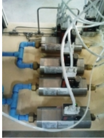
Figure 3.7: Photograph of the fluidisation and aeration mass flowmeters.
