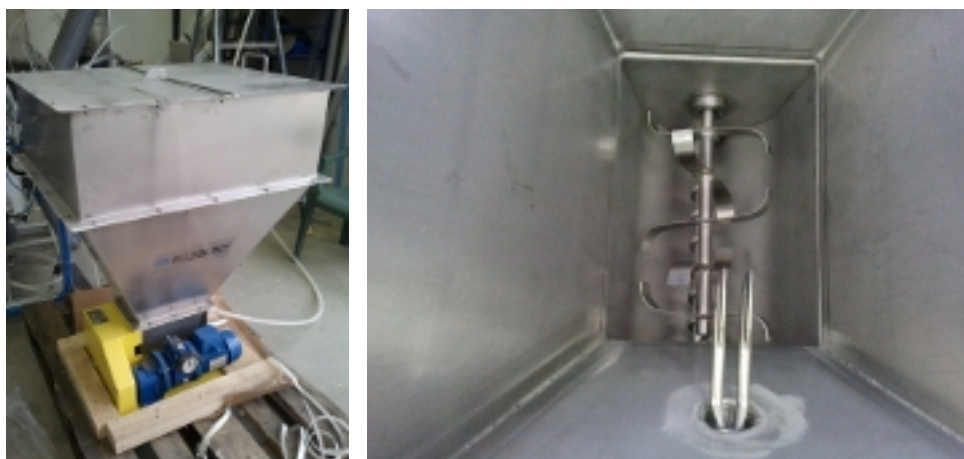
(a) Photograph of the hopper and its electric engine.
