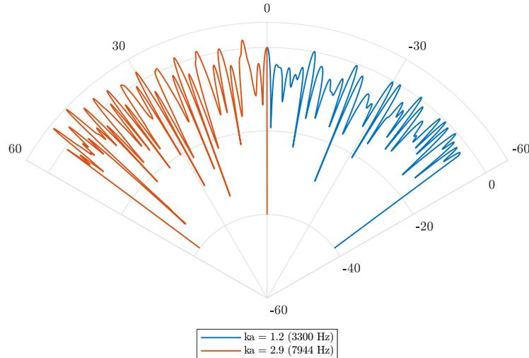
**Figure 6.6:** Point-source projected scattered pressure, as the result of the superposition and interference of  $N_{sl} = 15$  sources modelled as [Mellow and Kärkkäinen, 2011], with a source-to-source spacing of 0.08 m, and at a read-out distance of 1.66 m from the equivalent façade, as per anechoic measurements in §6.4.
