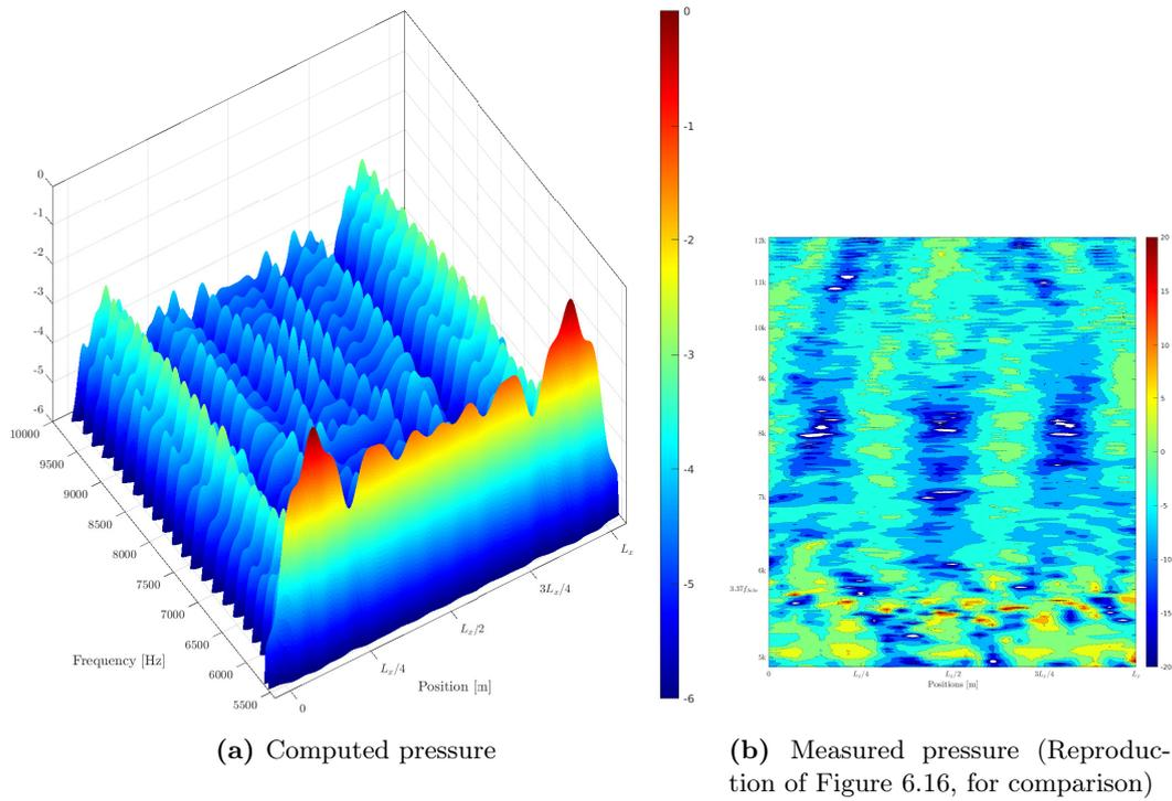
**Figure B.2:** Computed scattered pressure (normalized dB) in the range 5.5 kHz to 10 kHz as per [Mellow and Kärkkäinen, 2011] model, spanning the width the laboratory setup, with a grid spacing of 2 mm and a frequency bin of 2 Hz.
