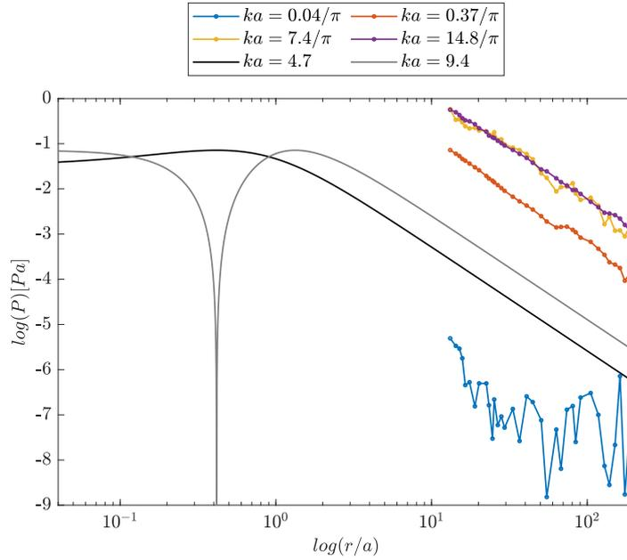
**Figure 5.7:** Pressure of the baffled speaker of radius  $a = 25.5$  mm as a function of the  $r/a$  distances for  $ka\pi = \{0.04, 0.37, 7.4, 14.8\}$ . Far-field approximation similarity of the measured piston-like radiator. Measured pressure at 1 m driving only the top speaker of the array. The solid black and gray lines are computed from theory for  $ka = 4.7$  and  $ka = 9.4$ .
