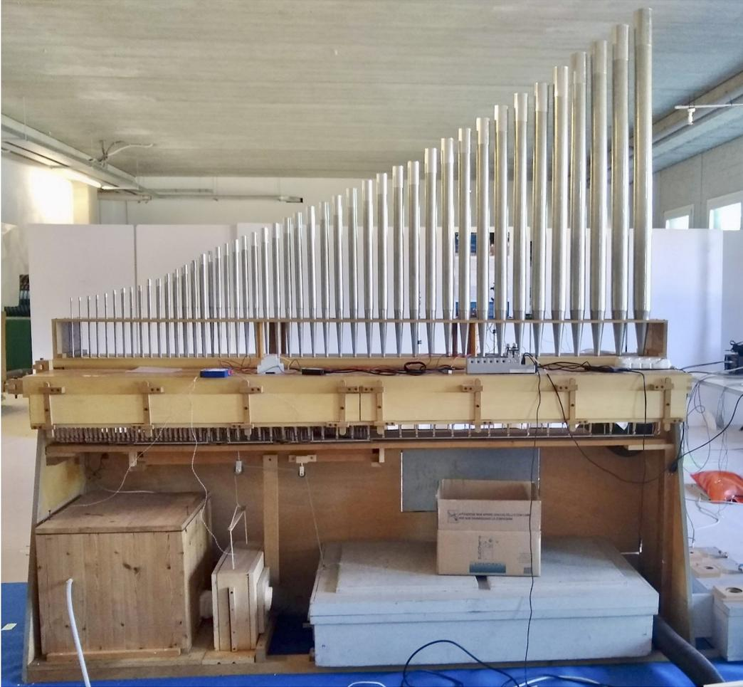
**Figure 3.7:** Measurement setup overview in the workshop organ as seen from the back. The keyboard is at the other side.
