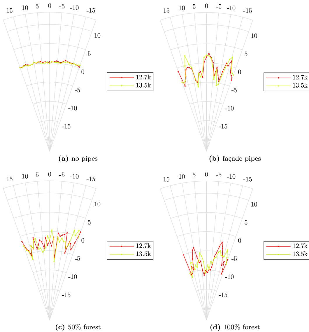
**Figure B.23:** 3-walled organ cavity at different densities of cylinders. Measured pressure, relative SPL dB rms normalized by free propagation reference at 2 m.
