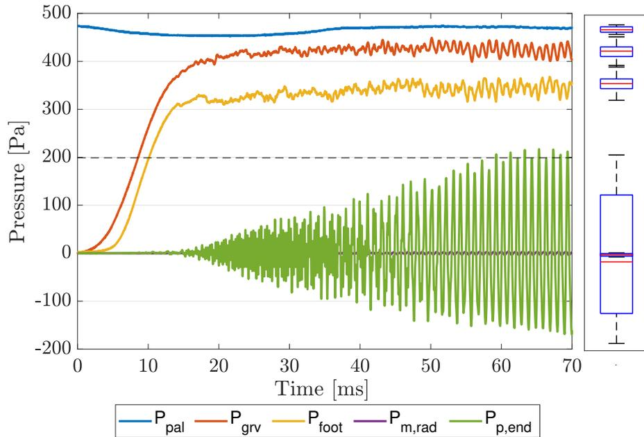
**Figure 3.3:** Left: overview of measured pressure time-series showing the transient build-up of Pipe 5, with geometry details in Table 3.1. The horizontal dashed line indicates the target pressure amplitude inside the resonator reached in SS. Right: data deviation, over 20 periods in SS.
