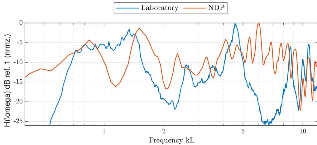
**Figure 6.22:** NDP buffet internal response as excited by a big balloon explosion compared with the internal response of the laboratory cavity. No pipes in the interior, and semi-open conditions (façade). The characteristic length is taken as  $L = \sqrt{L_x^2 + L_y^2 + L_z^2}$ , where for the NDP organ only the height of the first floor of windchests is considered ( $L_{y,NDP} = \sim 2$  m).
