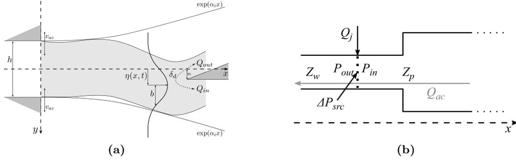
**Figure 4.2:** (a) Diagram of the mouth region and the associate geometrical and jet-related parameters (adapted from [Ernoul, 2016]). (b) One-dimensional impedance analogy of the flute-like instrument.
