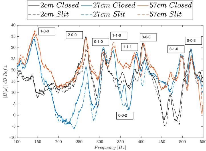
**Figure 6.12:** Measured internal pressure field for a cavity with no apertures and one aperture at different internal positions. Distances are referred over the  $\mathbf{X}$ -axis and away from the center of the front wall. The values for the modal frequencies annotated (closed cavity) may be found in Table 6.2.
