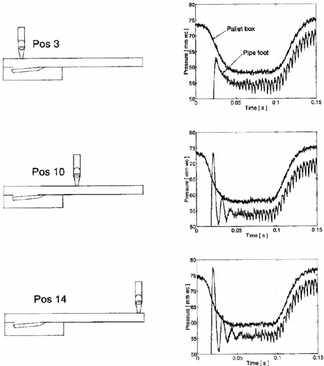
**Figure 3.16:** Different response amplitudes of the pipe foot pressure as a function of the distance to the opening valve. From [Carlsson, 2002]. Organ makers traditionally indicate blowing pressures in height water column. The target pressure of 75 mm water column corresponds to approximately 730 Pa.
