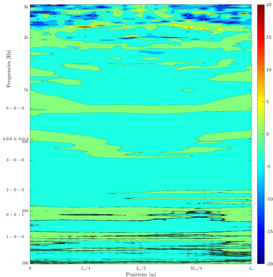
**Figure B.6:** Low frequencies of the measured facade pressure transfer function. Walls removed, only 16 cylinders at the front array. Measurement distance: 0.2 m from the front array. The effect of the reference field with no pipes and walls has been subtracted.
