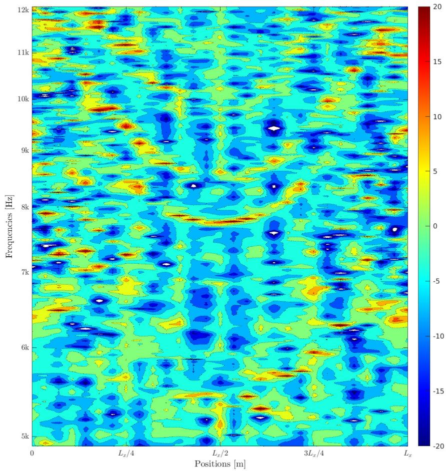
**Figure B.8:** High frequencies of the measured facade pressure transfer function. Walls removed, only 16 cylinders at the front array. Measurement distance: 0.2 m from the front array. The effect of the reference field with no pipes and walls has been subtracted.
