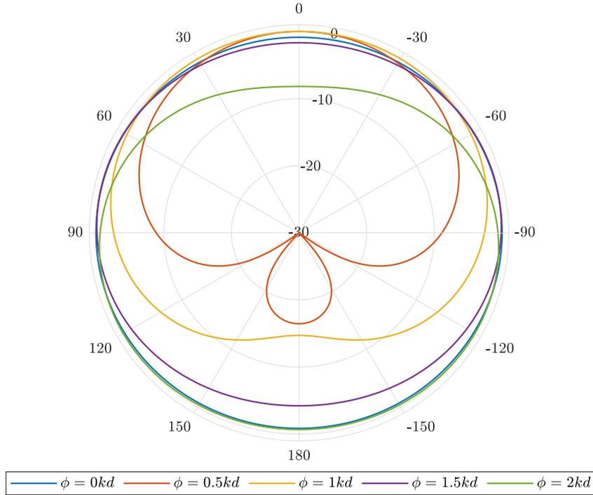
**Figure 6.4:** Following Rossi's model [Rossi, 1988], computation of radiated field by an array of equally distributed pulsating sources changing the  $\phi$  parameter for different values of  $kd$ , where  $d$  is the pipe-to-pipe separation and  $k$  the wavenumber.
