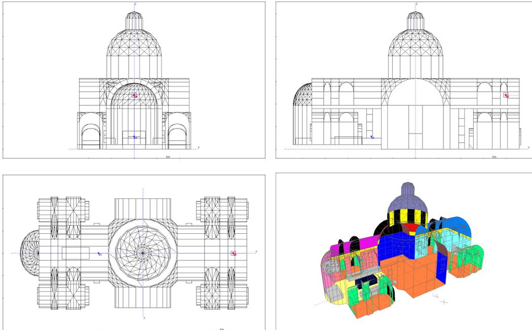
Figure 7.13: View of the GA model of Chapelle Sorbonne in CATT-Acoustic/TUCT.
