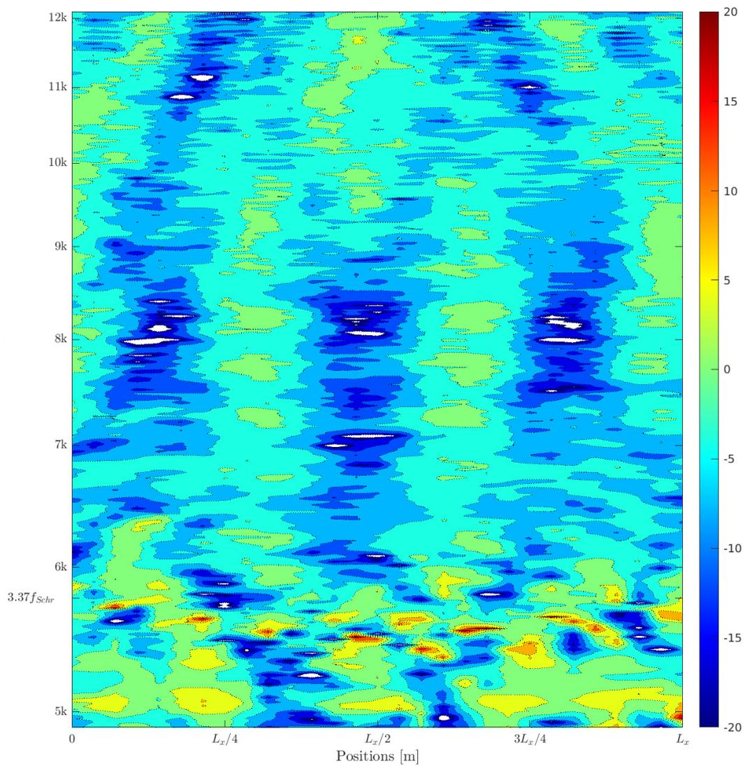
**Figure 6.16:** High frequencies of the façade response at 1.66 m away from the façade. No lateral or rear walls present and no other cylinders than the façade array. The effect of the source reference field with no pipes and walls has been subtracted.
