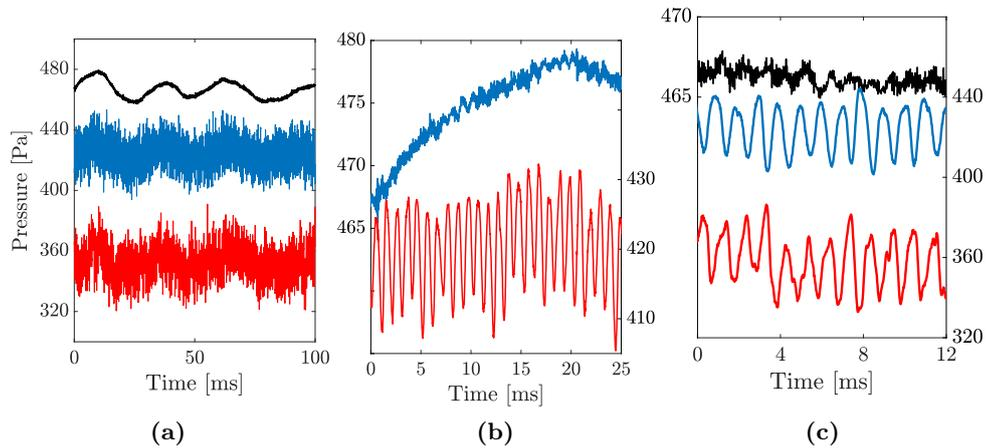
**Figure 3.11:** Measured pressure for  $p_{\text{pal}}$  (—),  $p_{\text{grv}}$  (—), and  $p_{\text{f}}$  (—) during steady-state segments with test pipe 5 in the workshop organ. (a) SS during 100 ms. (b) 12-period zoom segment from (a), where data for  $p_{\text{pal}}$  has been offset for visualization, and its axis appears at the top LHS.
