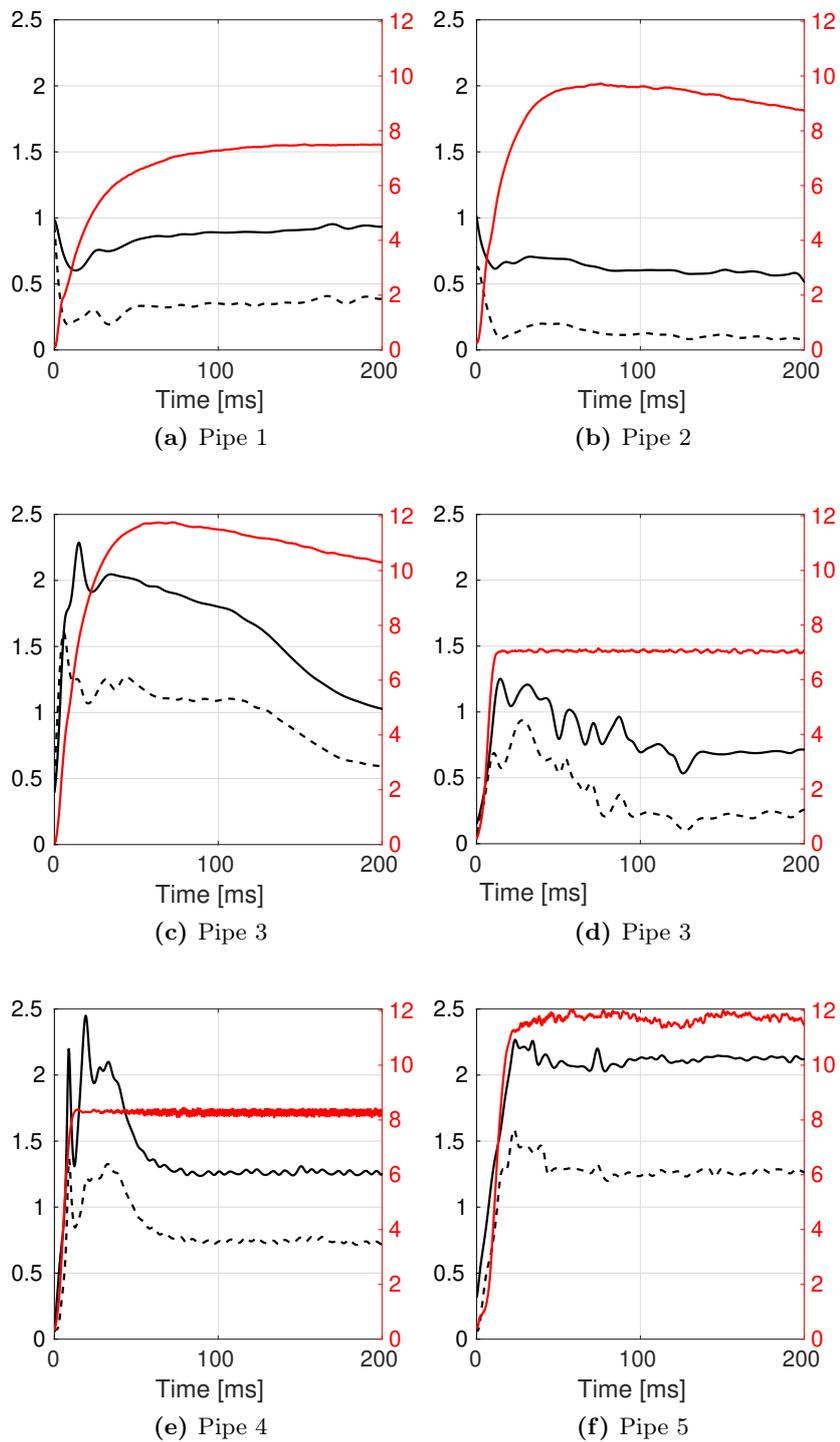
**Figure 3.9:** Ratio of second and third mode Fourier coefficients of the pipe's resonator internal pressure over the fundamental during the transient ( $a_2/a_1$  —,  $a_3/a_1$  ---, LHS numerical axes), overlaid with the reduced jet velocity ( $\theta$  —, RHS numerical axes). (a)-(c) Pipes 1-3 were measured in the experimental laboratory reservoir. (d)-(e) Pipes 3-4 were measured in the church organ. (f) Pipe 5 was measured in the workshop organ.
