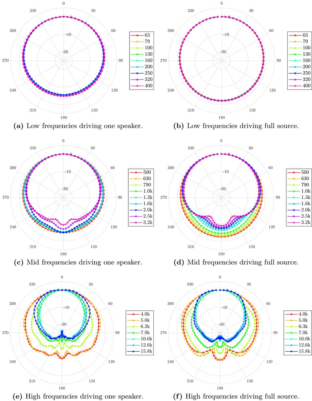
**Figure 5.3:** Measured directivity of the 1 m source at 0.2 m, analyzed in thirds of octave bands. Left: single speaker. Right: full array measured at half height. Normalized data at  $0^\circ$  per band.
