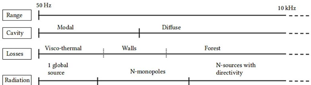
**Figure 6.1:** Organ radiation models per frequency ranges.
