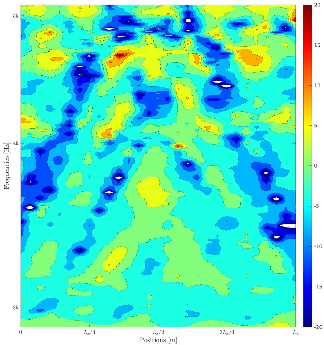
**Figure 6.15:** Mid-to-high frequencies of the façade response at 1.66 m away from the façade. No lateral or rear walls present and no other cylinders than the façade array. The effect of the source reference field with no pipes and walls has been subtracted.
