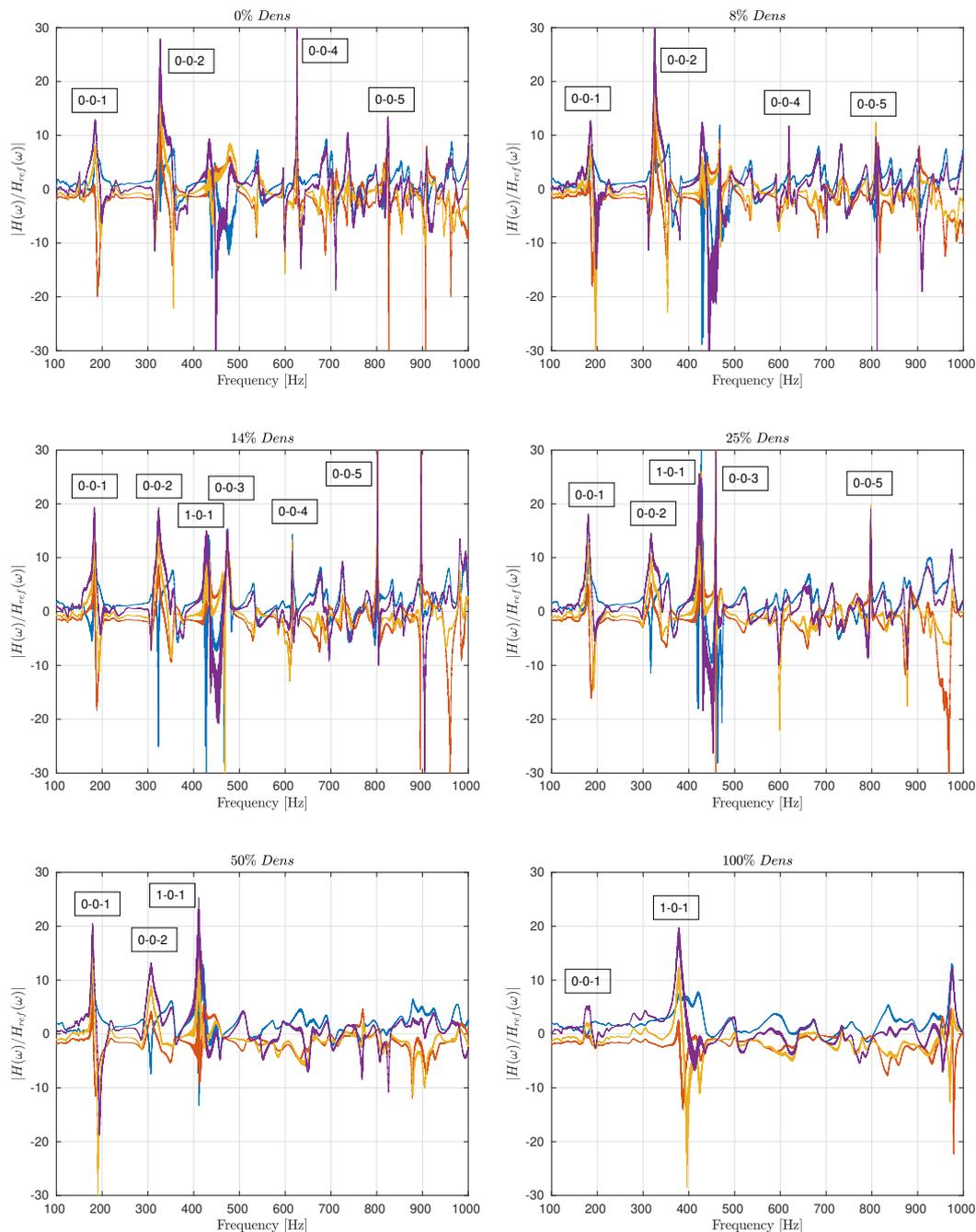
**Figure B.4:** Magnitudes of pressure at the slit for different vertical alignments. Bottom microphone to mid-low microphone: *Mic1/Mic2* —; mid-height to mid-low microphone: *Mic3/Mic2* —; mid-top to mid-low: *Mic4/Mic2* —; top microphone to mid-low: *Mic5/Mic2* —.
