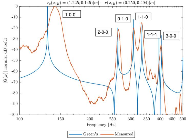
**Figure 6.11:** Measured spectra versus computed lossy Green's solution with wall impedance and losses of a single aperture as per Equations (6.17), (6.19) and (6.20). The source is located in a rear corner and the observation point in near the front panel, mid height (in the 3D measurement) and off the central node in the  $x$ -axis. The values for the modal frequencies annotated may be found in Table 6.2.
