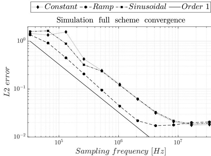
**Figure 4.4:** Convergence study of the full forward Euler scheme normalizing  $L_2$  errors by the reference numerical solution at  $\sim 67$  MHz, using 400 ms worth of steady-state mouth pressure signal. Slopes for the mid region of convergence are  $-0.95$ ,  $-1.09$ , and  $-0.9$ , respectively, for constant, ramp, and sinusoidal forcing terms.
