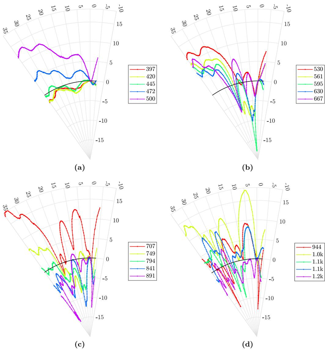
**Figure C.3:** Twelfth octave bands of relative SPL (dB) measured in empty tribune organ of NDP.
