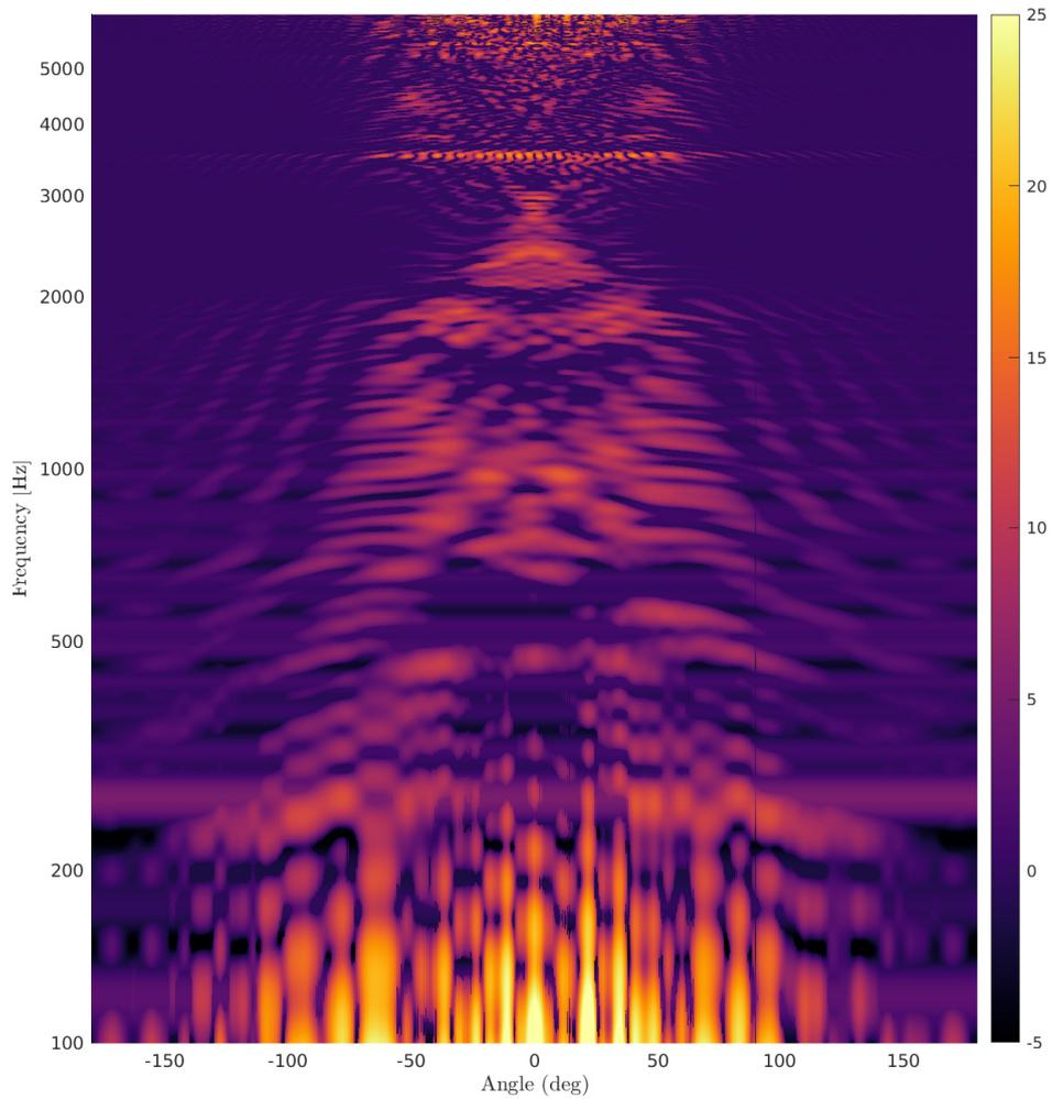
**Figure D.3:** Scattered pressure spectrum (dB) at the contour of 1.5 m around the organ-like system geometry. Sampling frequency 123.3 kHz, FFT size of  $2^{17}$  samples, window time 3000 time steps. The horizontal axis expresses the angle span around the coordinate center of the excitation injection point.
