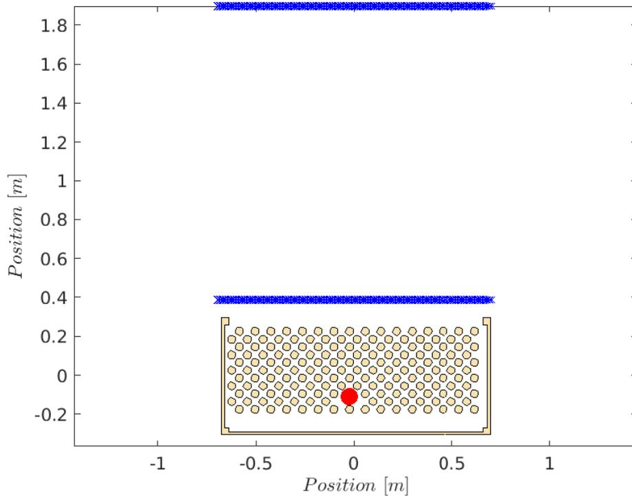
**Figure 6.25:** Meshed geometry for the 2D FVFDTD simulation of the scattering problem emulating the setup in laboratory condition. The red marker shows the position of excitation and the blue markers read-out locations.
