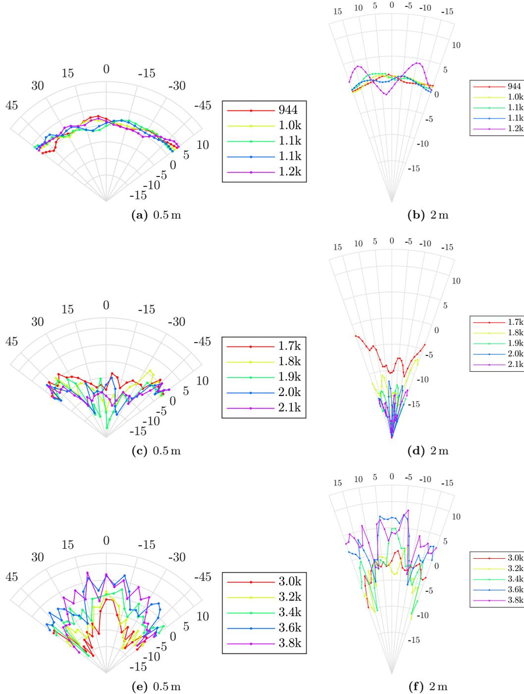
**Figure B.14:** Façade array of 16 equally distributed cylinders and 50% of the total forest cylinders in the cavity space ( $n_o = 134$ ), no walls of any sort. Measured pressure, relative SPL dB rms normalized by free propagation reference.
