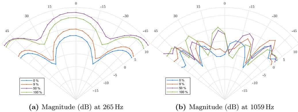
**Figure 6.19:** Relative SPL measured pressure (dB) at different densities near the semi-closed organ cavity (two lateral and one rear walls). Twelfth octave band analysis.
