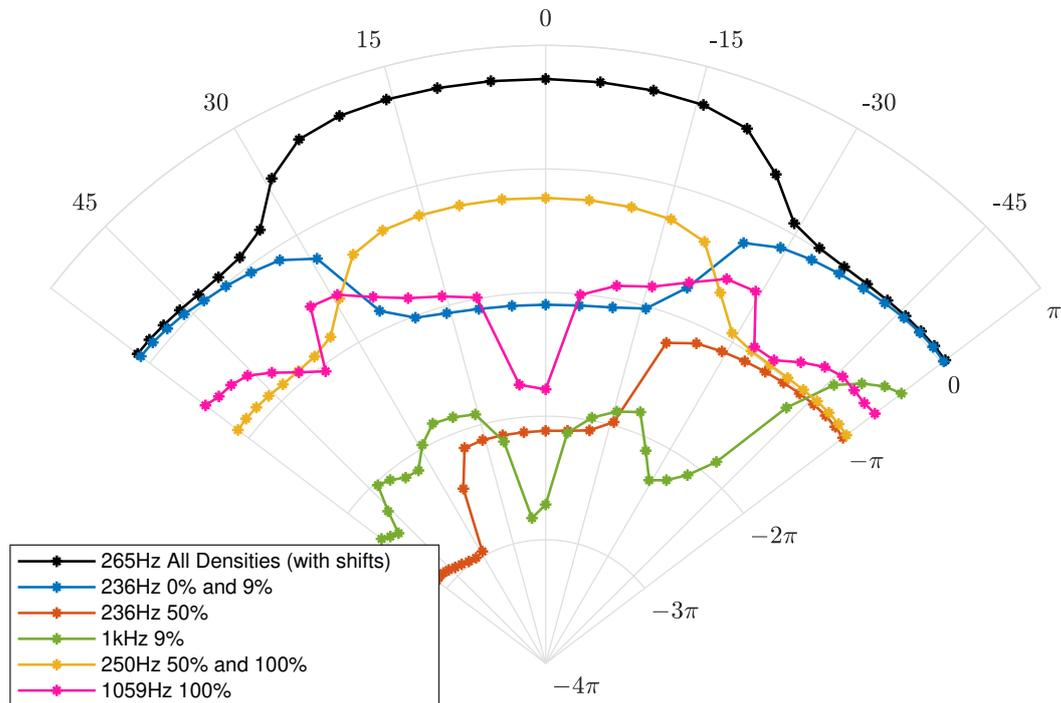
**Figure 6.20:** Measured pressure field phase (rad) at different densities of forest and different frequencies at 0.2 m of the semi-closed organ cavity (two lateral and one rear walls). Twelfth octave band analysis.
