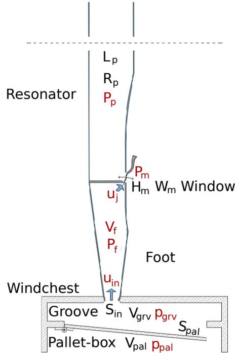
**Figure 3.1:** Diagram of reservoirs and organ pipe. In red, pressure and velocity variables; in black, geometry parameters. The size of the pallet valve has been increased for visualization purposes only.
