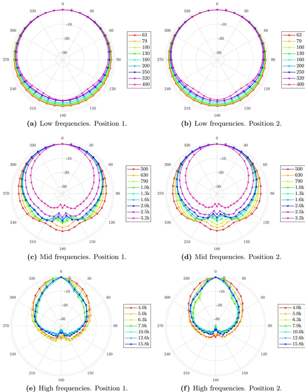
**Figure 5.9:** Directivity of the 2m source measured at 1 m. On the left: on axis with the membrane cone of the speaker immediately below half the height of the source. On the right: on axis with the membrane edge of the speaker immediately below half the height of the source.
