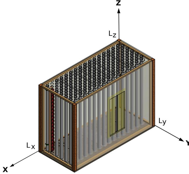
**Figure 6.2:** Diagram of the organ-like cavity, its internal elements, and cartesian  $\mathbf{X}-\mathbf{Y}-\mathbf{Z}$  coordinate system. Figure created by L. Quartier. Further details are provided in §6.4.1.
