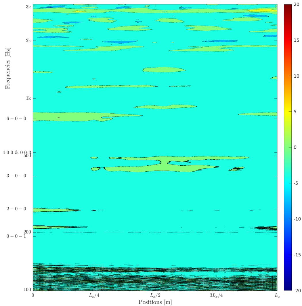
**Figure 6.14:** Low and mid frequencies of the façade transfer function at a distance of 1.66 m away from the façade. No lateral or rear walls present and no other cylinders than the façade array. The effect of the source reference field with no pipes and walls has been subtracted.
