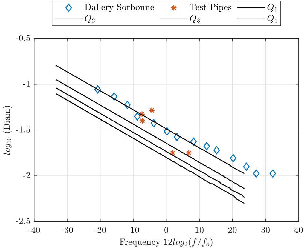
**Figure 3.4:** Pipe diameter ( $D$ ) scaling rules as a function of the resonator’s singing pitch (ref  $A_{440}$ ,  $f_o = 440$  Hz) and the stop typology to which they belong. Measured diameters from Prestant 4’ from Dallery organ in Chapelle Sorbonne ( $\diamond$ ), test Pipes 1-5 ( $\star$ ),  $Q_{n,max}$  models for  $n = \{2, 3, 4\}$  (-  $\bullet$  -, ---, and —, respectively).
