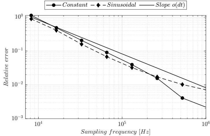
**Figure 4.3:** Convergence study of the resonator scheme ( $\delta_{tt}$ ,  $\delta_{t-}$ ,  $\delta_{t-}$ ) with constant and sinusoidal driving inputs. Numerical error is computed with respect to analytical solutions in Equation (4.15) and Equation (4.17).
