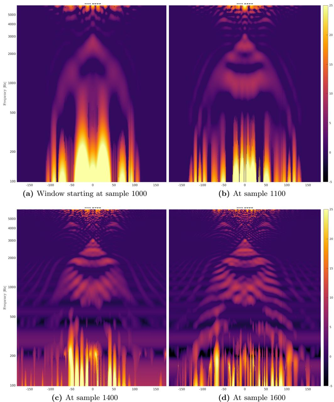
**Figure D.4:** Simulated scattered pressure read at the 4.5 m contour from the origin at different initial window times using a window length of 800 samples, an FFT size of  $2^{15}$ , and a time sampling frequency of 123.3 kHz. The axes span the same angle and frequency domain as in Figure D.3.
