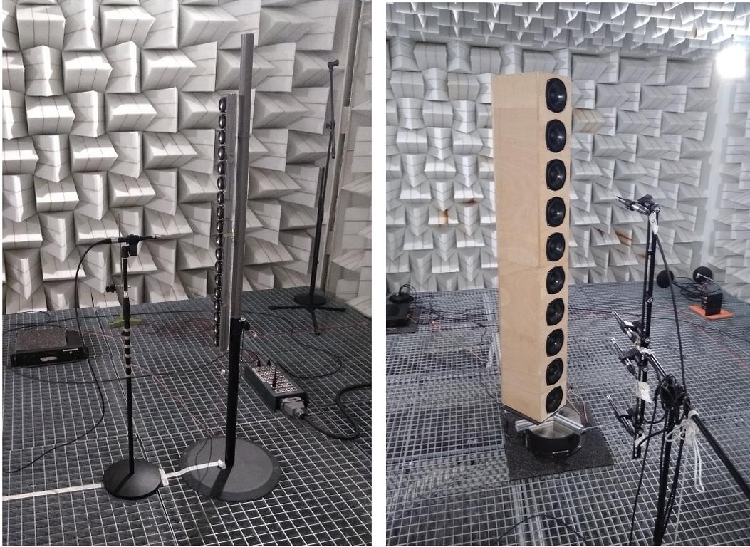
(a) The 1 m source measurements driving 18 speakers
