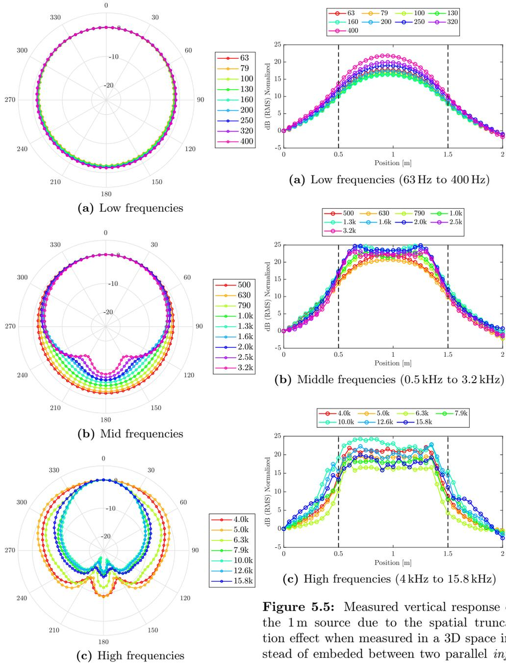
**Figure 5.4:** Directivity of the 1m source full array measured at 4m, analyzed per thirds of octave band.
