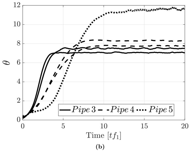
**Figure 3.8:** Reduced jet velocity  $\theta = u_j/W_m f_1$  over non-dimensional time  $t f_1$  (multiple measurements). (a) Pipes 1-3 (having foot volumes 0.150 L, 0.120 L, and 0.084 L, respectively) in the laboratory experimental reservoir driven by a fast-opening valve and reaching  $\sim 500$  Pa in SS. (b) Pipes 3-4 measured in the church organ and Pipe 5 in the workshop organ (having foot volumes 0.084 L, 0.020 L, and 0.021 L, respectively).
