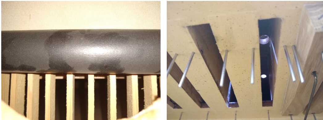
(a) Curtain regulating system between the blower and the parallel reservoir box.
