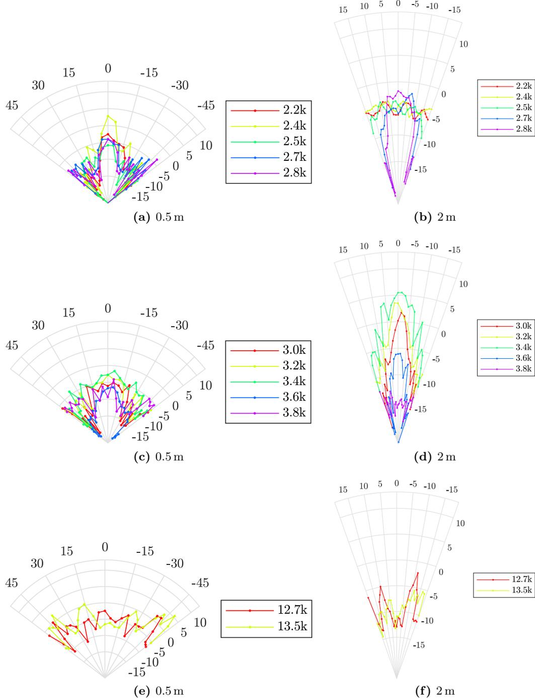
**Figure B.16:** Façade array of 16 equally distributed cylinders and 100% of the total forest cylinders in the cavity space ( $n_o = 244$ ), no walls of any sort. Measured pressure, relative SPL dB rms normalized by free propagation reference.
