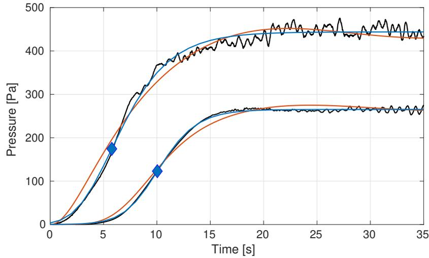
**Figure 3.12:** Measured pressure transient overlaid with time-stepping numerical solution of Equation (3.3) and the fitted model for  $p_{grv}$  and  $p_f$ . Markers indicate the maximum growth rate. Measured pressure (—), physical model (—), fitted model (—).
