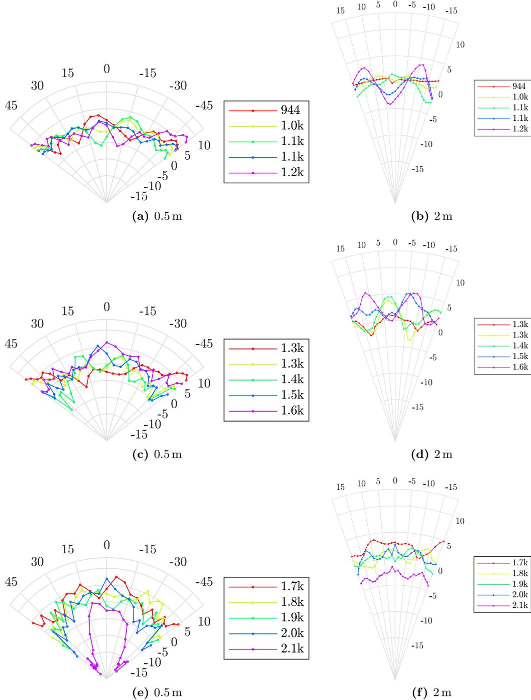
**Figure B.15:** Façade array of 16 equally distributed cylinders and 100% of the total forest cylinders in the cavity space ( $n_o = 134$ ), no walls of any sort. Measured pressure, relative SPL dB rms normalized by free propagation reference.
