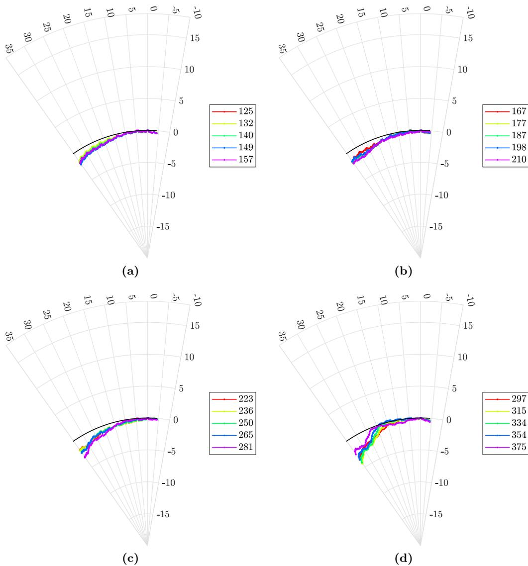
**Figure C.2:** Twelfth octave bands of relative SPL (dB) measured in the empty tribune organ of NDP.
