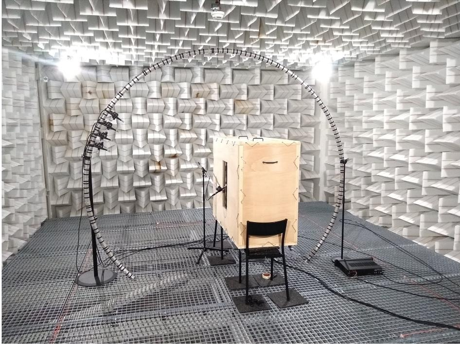
**Figure 6.28:** Laboratory measurement setup of the vertical directivity of the single slit at 1.3 m from the source (2D, inside) for 0% and 100% cylinder density conditions with the same protocol as in §6.4.1.
