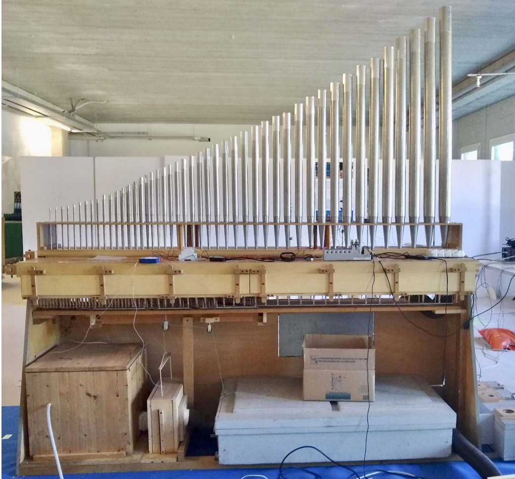
Figure 3.7: Measurement setup overview in the workshop organ as seen from the back. The keyboard is at the other side.
