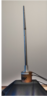
(a) Test pipe installed in the impedance measurement device
