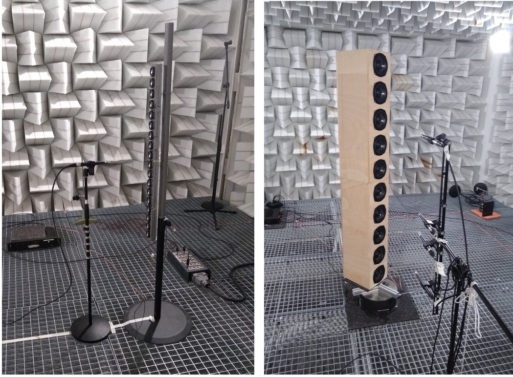
(a) The 1 m source measurements driving 18 speakers
