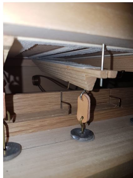
(b) Pallet valve in the workshop wind-chest.
