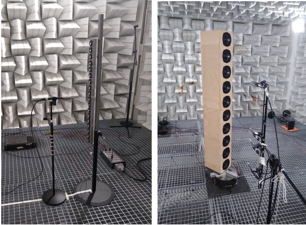
(a) The 1 m source measurements driving 18 speakers (b) The 2 m source during directivity measurements at a distance of 1 m at four different vertical alignments
