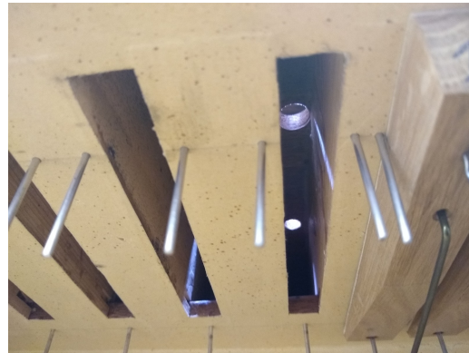
(b) Interior of a pallet-box and grooves with the sliders open and pipes removed. While Figure 3.1 shows a lateral view of the wind-chest and the pallet valve open, this frontal image offers the view from below the slot to which the pallet valve gives access.
