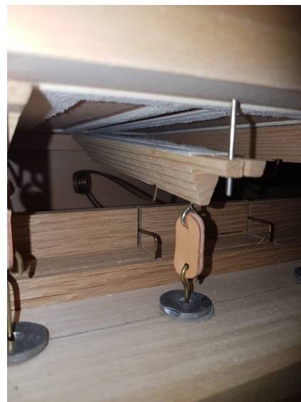
(b) Pallet valve in the workshop wind-chest.
