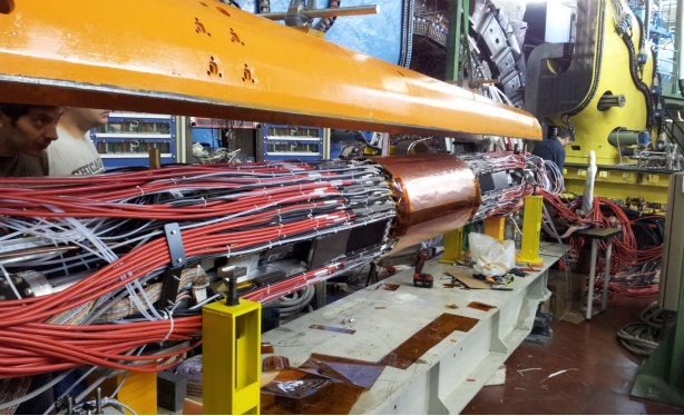
Figure 2.1: Photo taken before the insertion of the central assembly inside the detector. The orange cover on top is used for the support during installation. Accelerator components are hidden under the wires on each side of the inner tracker (copper colored in the middle). (Courtesy of Luigi Pellegrino, 2023)
