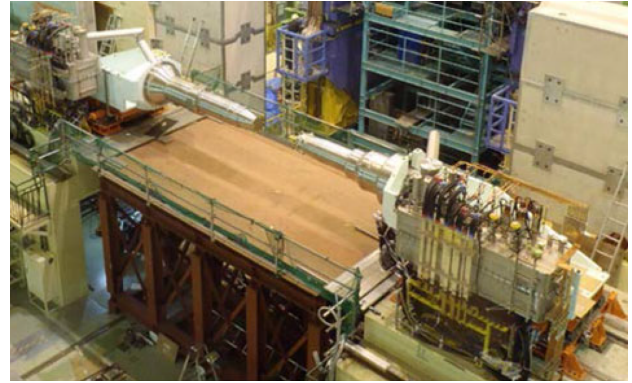
Figure 2.5: Picture of the MDI of SuperKEKB, the detector being in the maintenance position. The asymmetric cryostats (shining metallic part) can be seen in their cantilever configuration at the center of the picture (cf. [3]).
