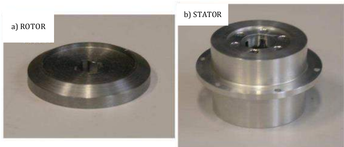
Fig. 2.15 The actuator parts: a) rotor, b) stator [72]
