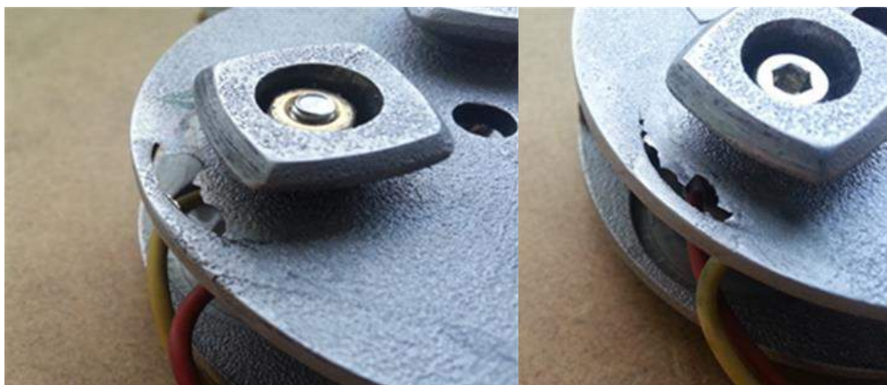
Fig. 7.3 The cracks caused by the vibration on the counter-mass
