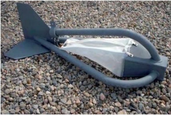
Figure 1.9 : Helley-Smith sampler (HS) (Malavoi et al., 2012)
