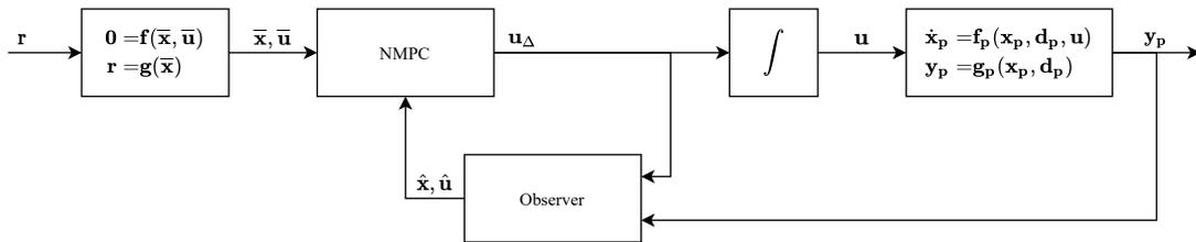
Figure 2.29 – NMPC block diagram for offset-free control.
