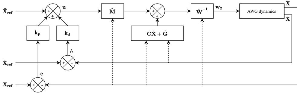
Figure 2.9 – Computed torque control block diagram.
