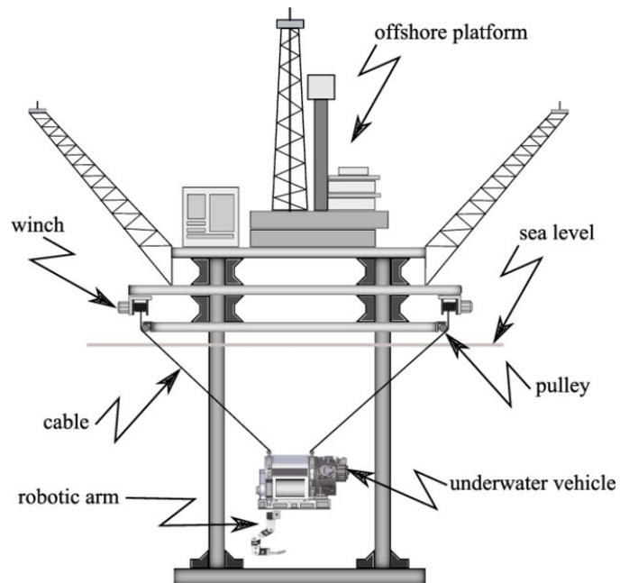
Figure 1.7 – HCT-a-UVMS (figure from (El-Ghazaly et al., 2015)).
