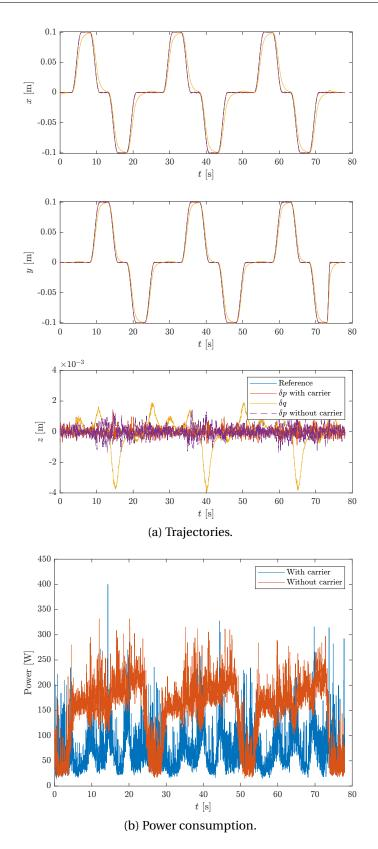
Figure 3.8 – AWG power consumption comparison with and without the CDPR carrier.
