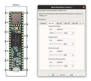
Figure B.1 – Teensyshot Simulink block.
