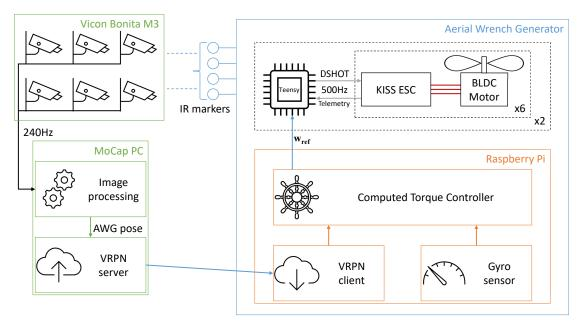
Figure 2.8 – AWG electronic architecture for CTC experiments.
