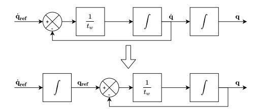
Figure 3.10 – Equivalent delta-input formulation of the carrier dynamics.
