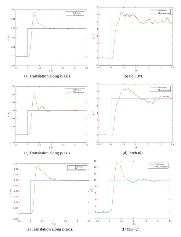
Figure 2.16 – Position (left) and orientation (right) step responses.
