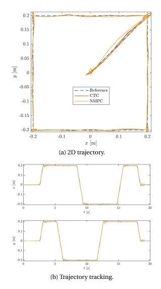
Figure 2.27 – 2D trajectory tracking by the AWG with NMPC and CTC.
