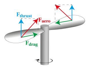
Figure 2.2 – Forces on propellers.
