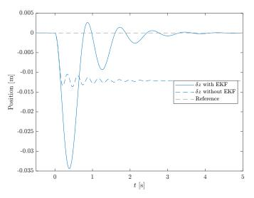
Figure 3.12 – Response of the NMPC to a step disturbance.
