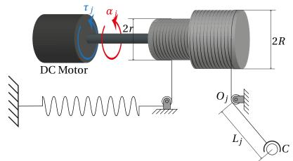
Figure 3.2 – CDPR actuated winch parameters.
