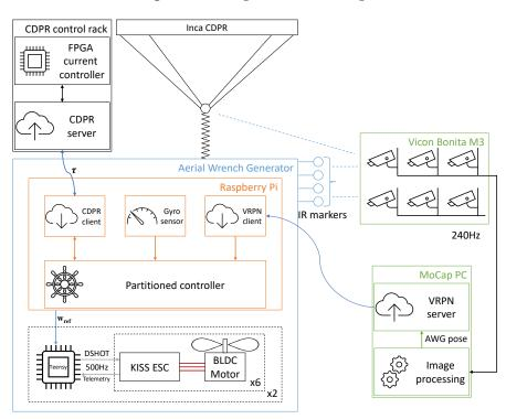
Figure 3.4 – Electronic architecture of the AMES.
