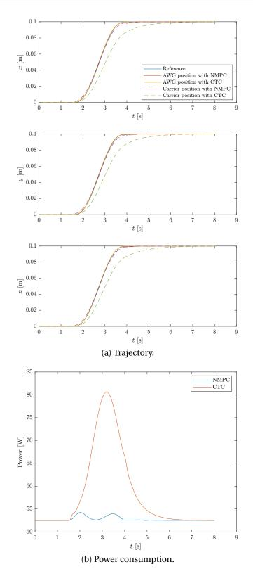
Figure 3.13 – AWG power consumption comparison with NMPC and partitioned controller.
