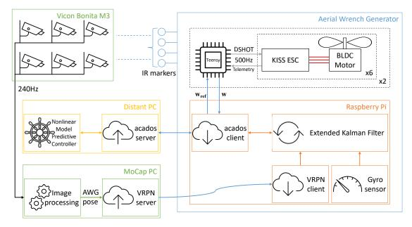
Figure 2.23 – AWG NMPC architecture.
