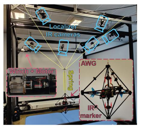
Figure 3.3 – Experimental setup.
