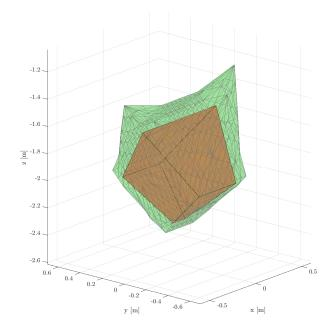
Figure 2.14 – Total orientation workspace of the AWG.
