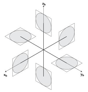
Figure 2.4 – Propeller configuration (figure inspired by (Brescianini & D'Andrea, 2018)).
