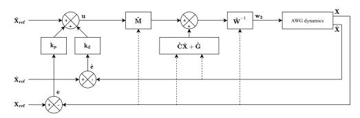
Figure 2.9 – Computed torque control block diagram.
