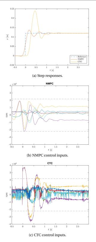
Figure 2.26 – Responses for a position step and control inputs (dashed lines are actuator saturation).
