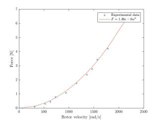
Figure 2.13 – Thrust coefficient identification.
