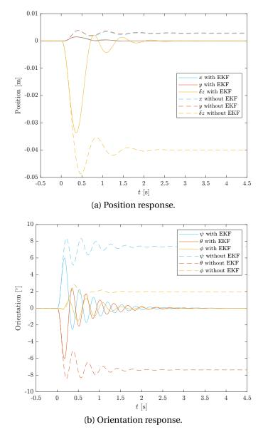
Figure 2.30 – Response to a disturbance step with and without EKF.
