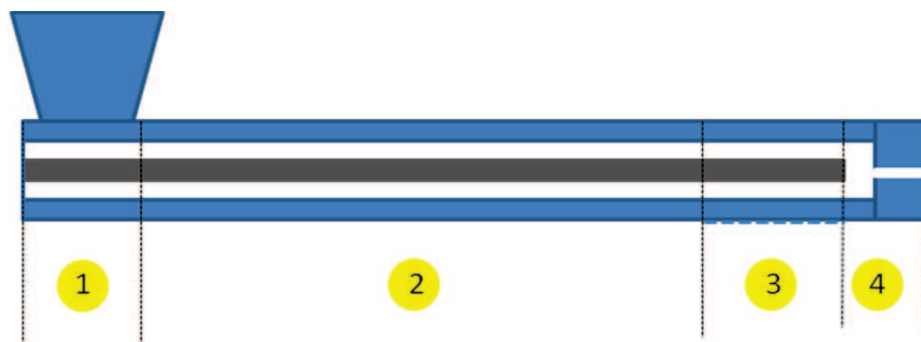
Figure 19: Functional zones of pressing (single-screw extruder OMEGA 20)
