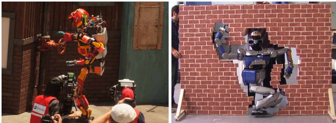
Figure 1.1: Motion planning for humanoid robots is computationally hard, but could enable breakthrough technologies and could provide us with a deeper algorithmic understanding of intelligent behavior. Left: Robot at the DARPA robotics challenge manipulating a valve. Right: Robot HRP-2 walking through a wall. Orthey, Andreas. 2015.
