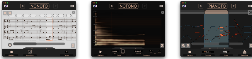
Figure 1.1: The three music creation interfaces I developed as part of this PhD: NONOTO , for sheet music composition, NOTONO for visually-grounded sound creation and PIANOTO , for expressive piano performance creation. Each of these interfaces enables local re-generation of portions of the represented musical material, assisted by a backend AI model.
