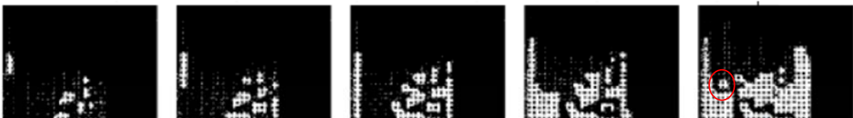
Hydrophilic (20140313 EXP 6), Condensation process of a hydrophilic situation Time, 0.38 1.454.36 days. the area percent : 0.030, 0.067, 0.136.
