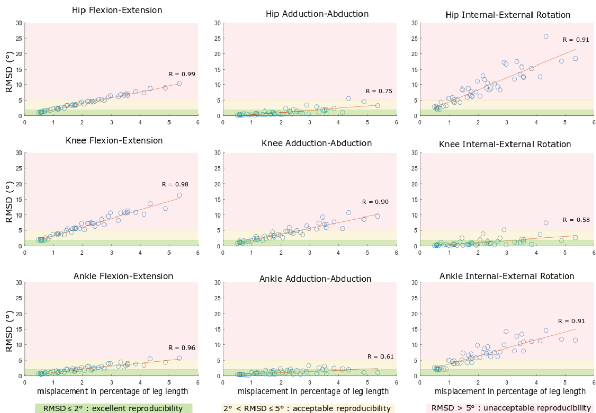
Figure 20. Correlation between RMSD and magnitude of misplacement in percentage of leg length. Scatter plot representing RMSD for all tested magnitudes to misplacement of the KNE marker on the AP direction considering the CP population. R (correlation coefficient).
