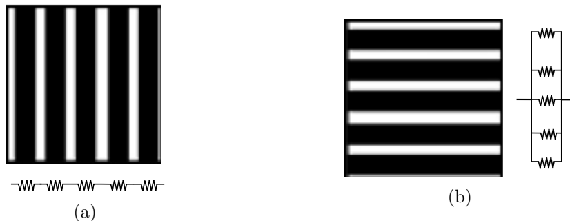
Figure 2.20: Equivalent medium as a network of electrical resistors (a) Parallel model (b) Series model.
