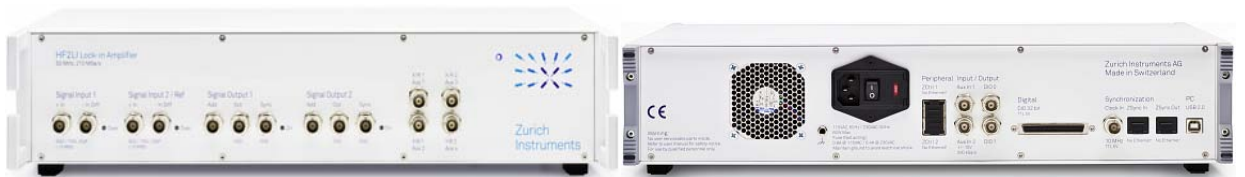
Figure 4.13: Lockin amplifier HF2LI MF by Zurich instruments used in the experiments.
