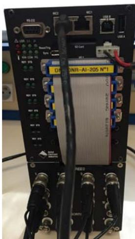
FIGURE A.6 – Centrale d'acquisition UEIDAQ.
