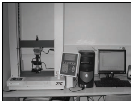
Figure 3.17: H25KS Brazilian testing equipment.
