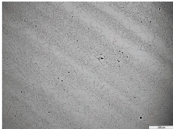
**Fig. 3.2** OM image of A600 heat WL344 (Imphy) in its as received material state. The small black spots seen in the image are chromium carbide ( $\text{Cr}_x\text{C}_y$ ) precipitates and the larger more angular black structures have been identified as TiCN by SEM-EDS analysis.
