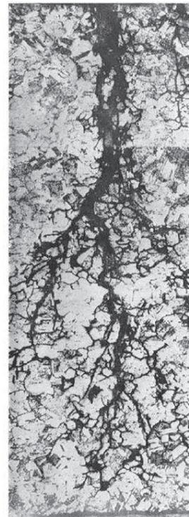
**Fig. 2.1** Stress corrosion crack in Ni base alloy 600 after exposure in high temperature water [2].
