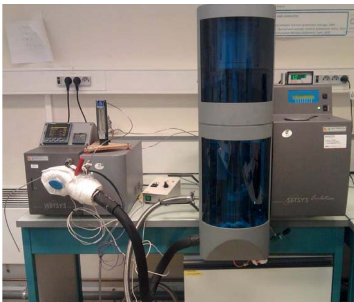
Figure 44. ATG (right of the picture) coupled to a wet gas generator (left of the picture)
