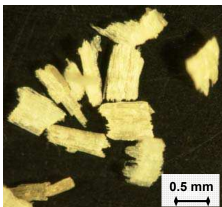
Figure 38. Microscopic view of wood particles from the 0.35 mm sample
