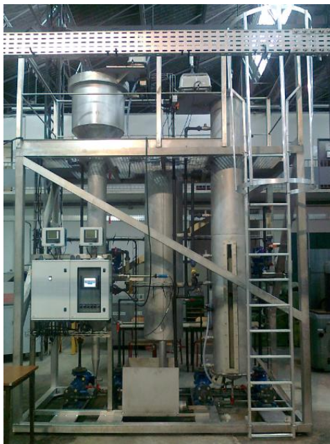
Figure VI. 1: GSBR (right) and crystallizer (left) pilots for real wastewater treatment coming from the cheese industry.
