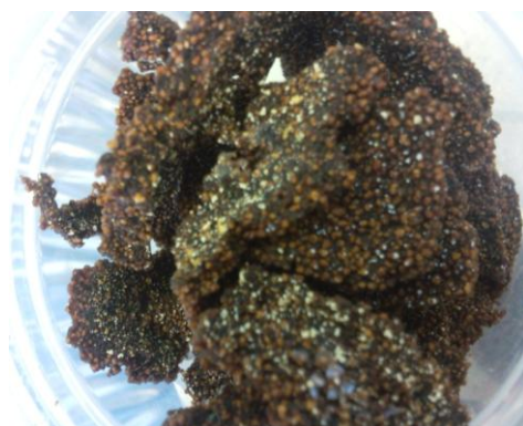
Figure VI. 2: Air-Dried granular sludge purged from GSB1.
