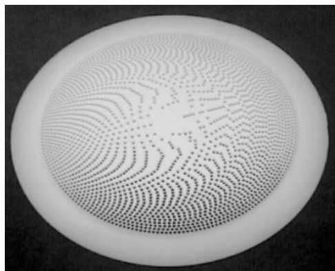
Figure 1.32 – Luneburg lens realized by hole drilling method [57]
