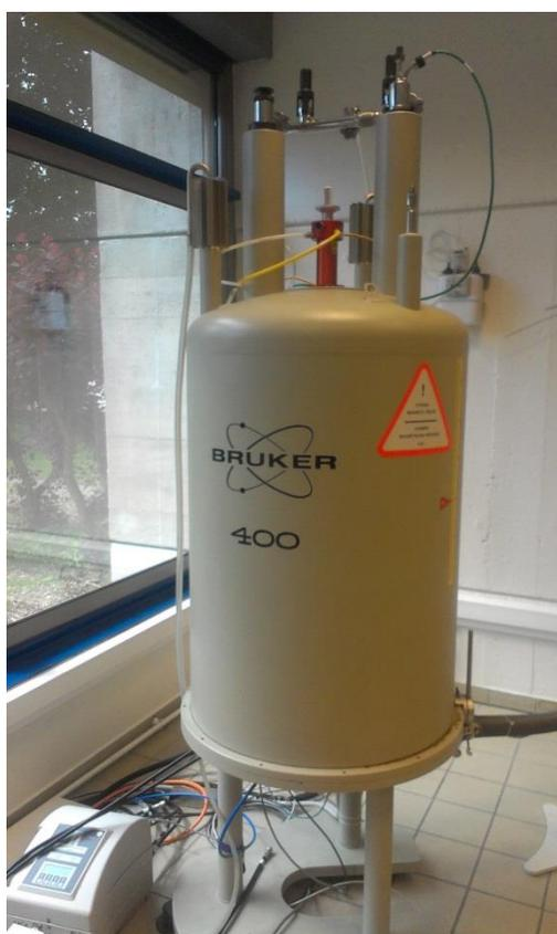
**Fig. 41. Solid-state NMR device.**
