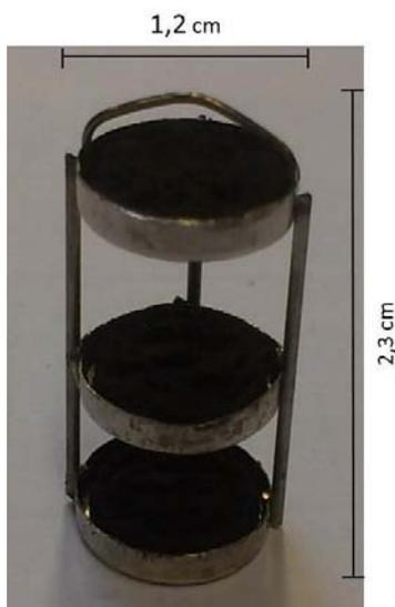
**Fig. 34. Three-staged crucible for TGA torrefaction.**
