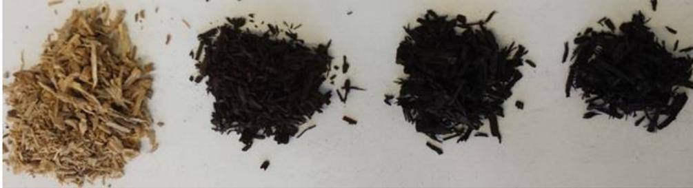
**Fig. 17. Evolution of an ash-wood sample during torrefaction. From left to right: raw biomass, and biomass torrefied at 250, 280 and 300°C under the same conditions (Lê Thành et al., 2015).**
