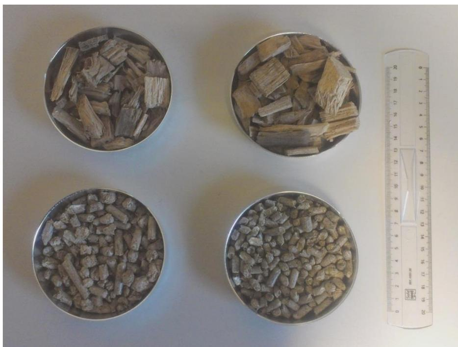
**Fig. 30. The four biomasses: pine chips on the top left; ash-wood chips on the top right; miscanthus pellets on the bottom left; and wheat straw pellets on the bottom right.**
