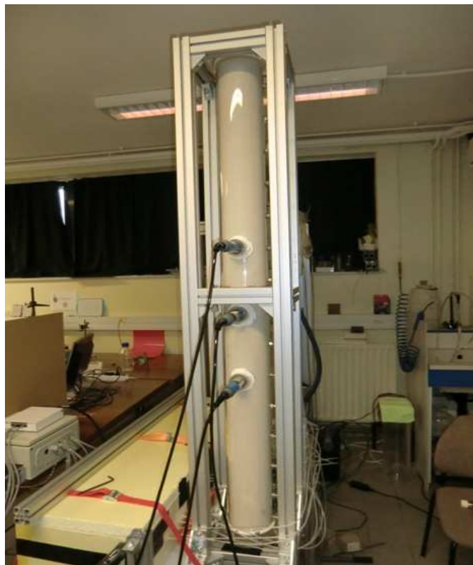
Fig. 5.16: The sand column at the end of the filling process.
