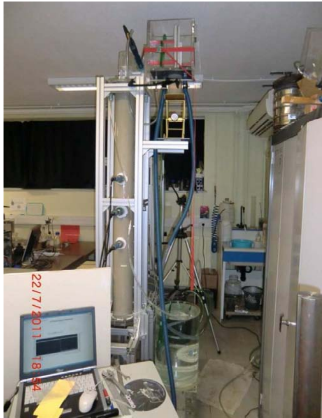
Fig. 5.19: Constant head permeability test conducted on the sand column to measure the saturated hydraulic conductivity. Two overflow tanks are attached at the top and bottom of the column
