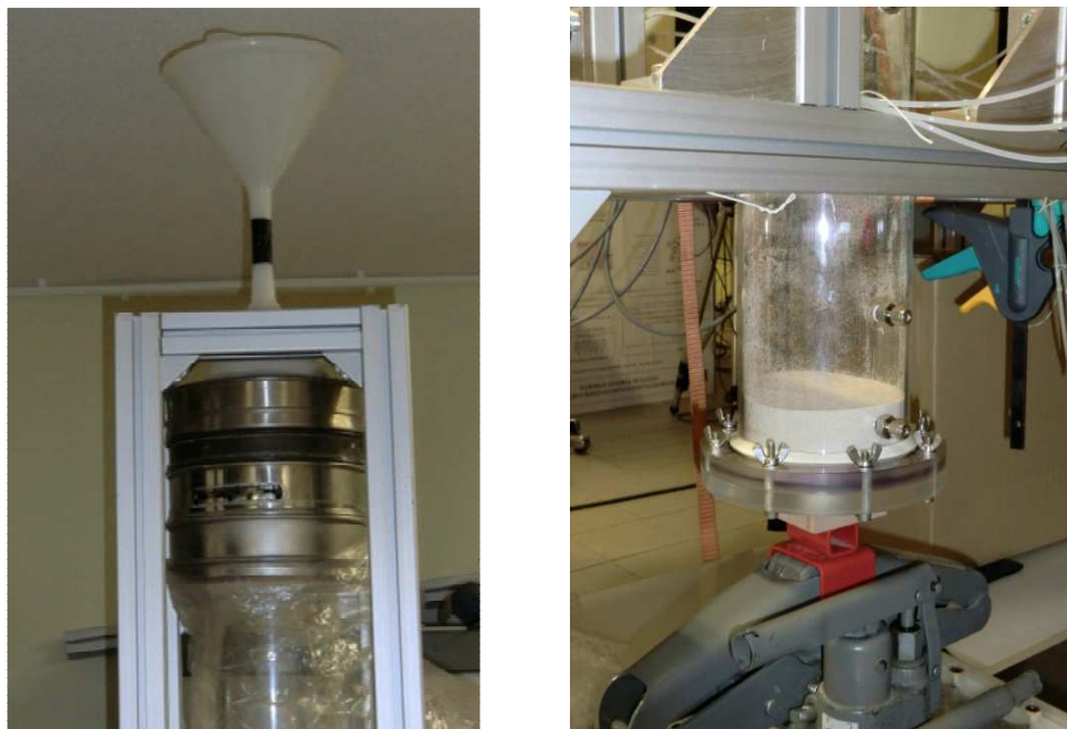
Fig. 5.15: Left: Photos of sand raining method used to fill the 1D sand column with four sieves and a funnel. Right: photo of the column bottom during the early stage of the filling process.
