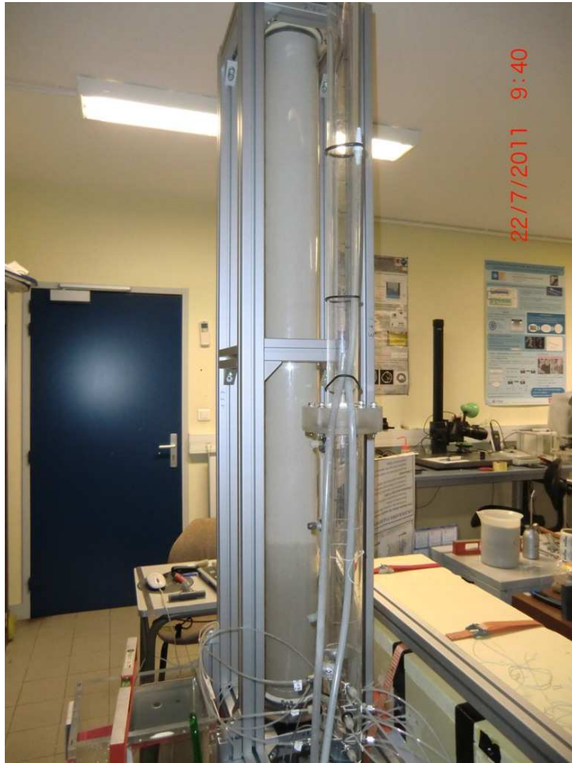
Fig. 5.20: Photo of the sand column at the end of the imbibitions step (the imposed water table height is Z_{S_{Applied}} = 5\text{mm} measured from the bottom of the sand). This photo corresponds to a steady state conditions.
