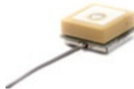
FIGURE 2.19 – Patch céramique GPS du commerce.
