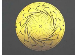
FIGURE 2.28 – Antenne Novatel sans son radôme.
