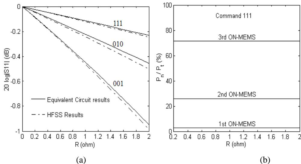
**Figure 3.2:** (a) Results obtained by equivalent circuit and HFSS under single MEMS case (a) Comparison between power loss results obtained by HFSS and the equivalent circuit for the unit cell as a whole (b) Power dissipated within the ON-MEMS individually ( $P_n$  represents the individual power of an ON-MEMS,  $n$  denotes the number of the ON-MEMS,  $P_t$  denotes the total power dissipated within the unit cell).
