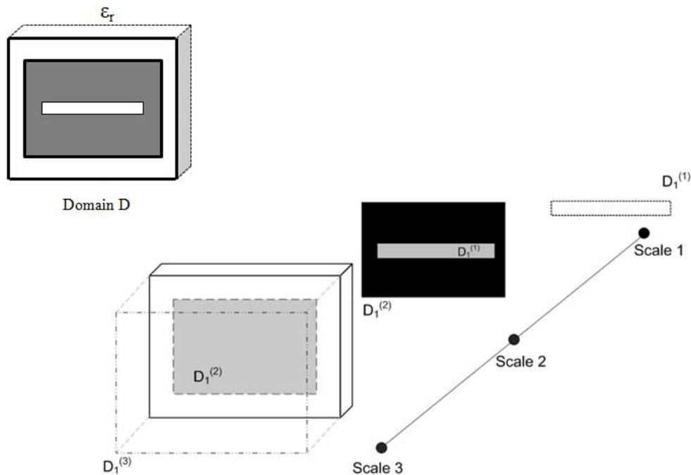
**Figure 5.2:** Partitioning the discontinuity plane  $D$  of the planar reflector in its constituent domains and sub-domains at three scales, white portions represent dielectric, black represents metal and grey parts are mere projections of the immediate sub-domains.
