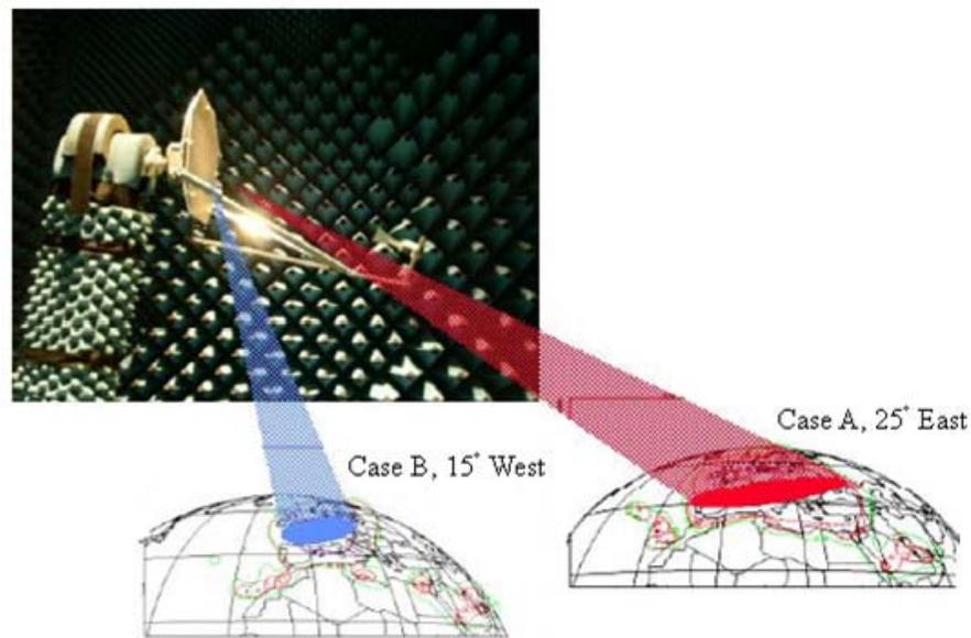
**Figure 1.3:** Depiction of an electronically reconfigurable reflectarray antenna [2]
