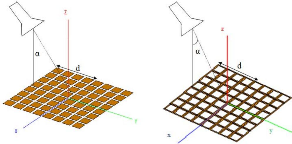
**Figure 6.18:** Basic configuration of free-standing planar structures with feed horn (a) metallic patch structure: patch dims 13.5x13, unit-cell dims 16.8x16.8 (b) metal grid structure: aperture dims 13.5 x 13, unit- cell dims 16.8 x 16.8 (all dimensions are in mm).
