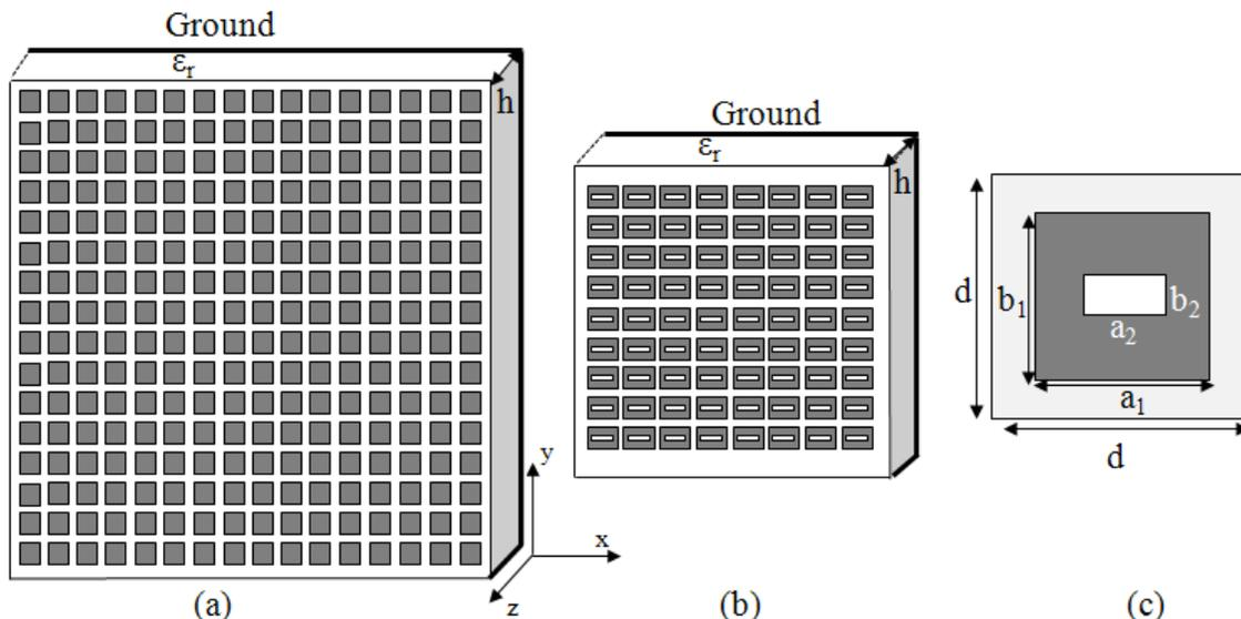
**Figure 6.11:** (a) A 256-cell ( $16 \times 16$ ) reflectarray geometry, unit cell and patch dimensions are the same as given in (c). (b) A 64-cell ( $8 \times 8$ ) reflectarray geometry with  $h=3.175\text{mm}$ ,  $\epsilon_r=2.17$ . (c) An enlarged unit cell with  $d=16.8\text{mm}$ ,  $a_1=13.5\text{mm}$ ,  $b_1=13\text{mm}$ ,  $a_2=9\text{mm}$  and  $b_2=6\text{mm}$ .
