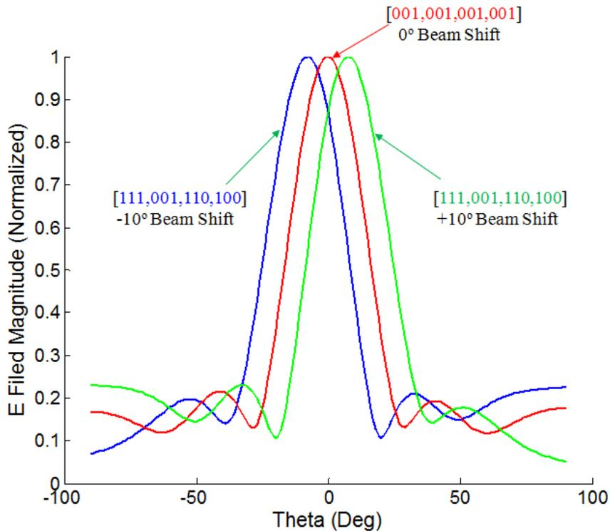
**Figure 6.27:** Normalized SCT results of  $4 \times 1$  uniform reflectarray of Figure 18, the electronic configurations (i.e., the switching states (ON/OFF) for all the three types are shown in the Figure.
