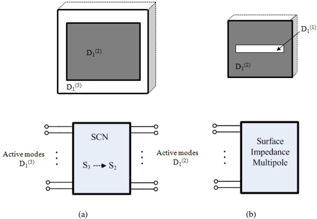
**Figure 5.4:** Decomposition of the problem in two sub-problems. (a) SCN is computed from the structure shown above (b) Surface Impedance Multipole is computed from the problem involving patch and slot domain only.
