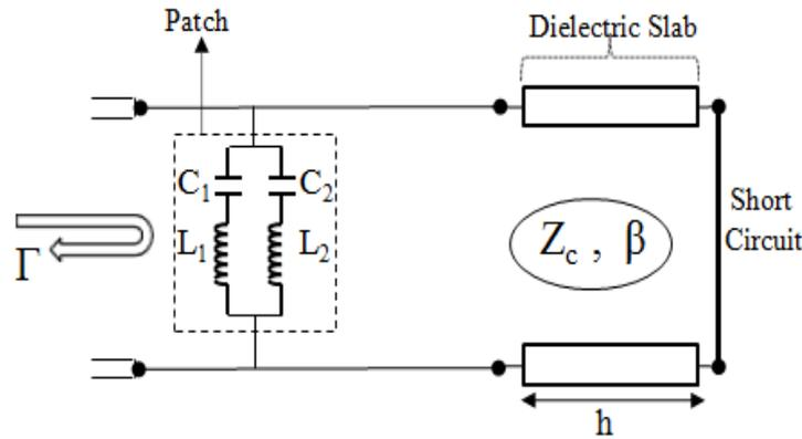
**Figure 2.5:** Equivalent electrical circuit model for microstrip patch
