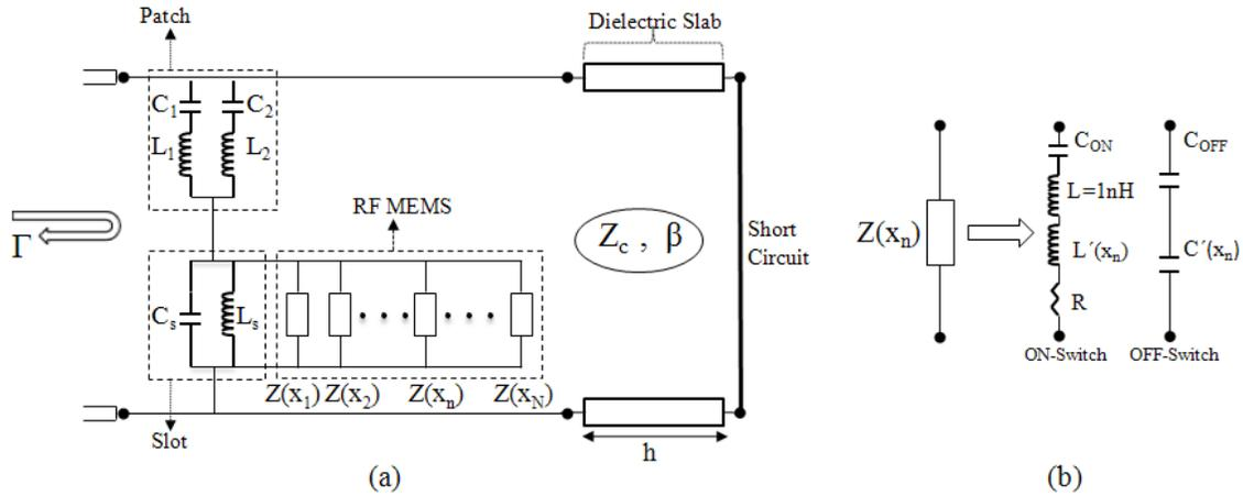
**Figure 3.1:** (a) Equivalent electrical circuit for the MEMS-controlled phase-shifter cell; (b) Equivalent circuit model of the  $n^{\text{th}}$  MEMS switch within the slot (the equivalent impedance  $Z$  depends on the ON/OFF state of the switch as well as its coordinate  $x_n$  inside the slot).
