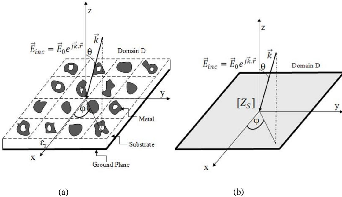
**Figure 6.7:** (a) An  $N \times N$  microstrip reflectarray of arbitrary cells under arbitrary plane wave incidence. (b) The surface impedance matrix  $[Z_S]$  modeling the domain  $D$ , this matrix is derived from the cascade of scale changing networks as shown in Figure 6.9.
