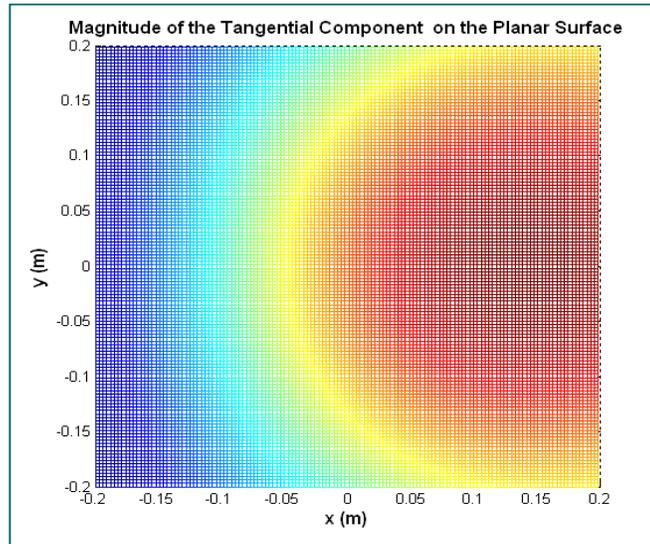
**Figure B.5:** Tangential field pattern of a horn antenna placed at an offset of 200mm from the center of the surface with an angle of inclination equal to  $30^\circ$ .  $d=660\text{mm}$
