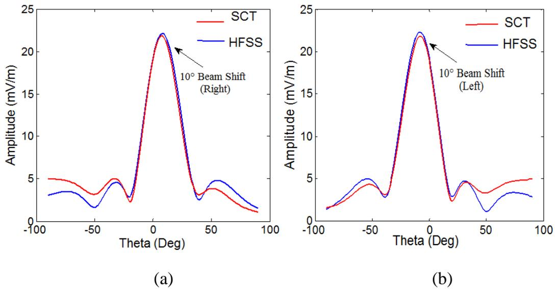
**Figure 6.26:** Radiation patterns of  $4 \times 1$  uniform reflectarray of Figure 18, the electronic configuration (i.e., the switching states (ON/OFF) for the twelve RF-MEMS switches of four phase shifter cells) of the four phase shifter cells are non-identical and hence obtaining H plane patterns asymmetrical (a) H-plane pattern with electronic configuration of the four elements as  $[111\ 001\ 110\ 100]$  (b) H-plane pattern with electronic configuration as  $[100\ 110\ 001\ 111]$ .
