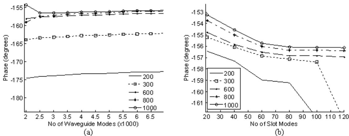
**Figure 5.8:** Convergence study of the phase of reflection coefficient for configuration 3 ( $L_p, W_s$ )  $\Rightarrow$  (8, 8), frequency 12.1GHz: (a) Convergence with respect to the number of modes in the periodic waveguide (legend indicates number of patch modes); (b) Convergence with respect to number of modes in the slot (legend indicates number of patch modes).
