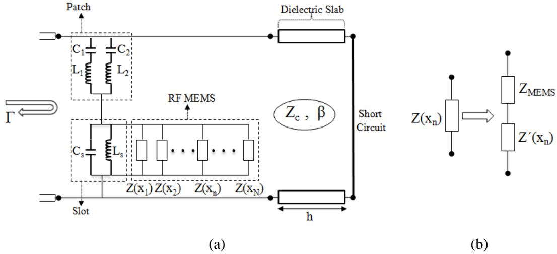
**Figure 2.12:** (a) Equivalent electrical circuit for a phase-shifter cell comprising of  $N$  MEMS; (b) Equivalent circuit model of the  $n^{\text{th}}$  MEMS within the slot (the total impedance  $Z_{\text{MEMS}}+Z'$  depends on the ON/OFF state of the switch as well as its coordinate  $x_n$  inside the slot).
