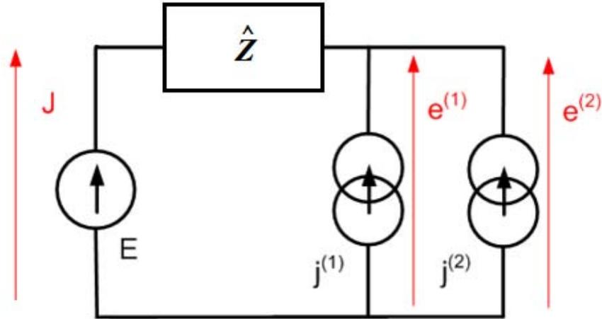
**Figure 6.3:** Simplified Equivalent circuit. Virtual source and the scale-changing source of each branch (when defined in the same domain and using same orthogonal modal-basis) can be replaced by a single current source.
