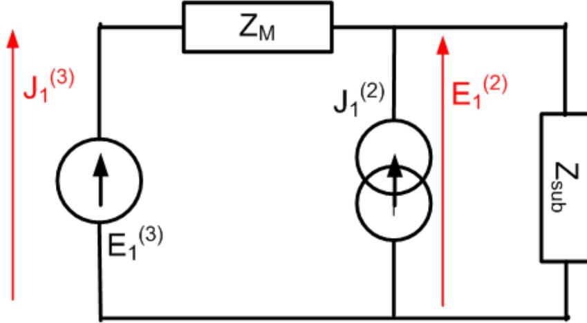
**Figure 5.7:** Simplified equivalent circuit of Figure 5.6.
