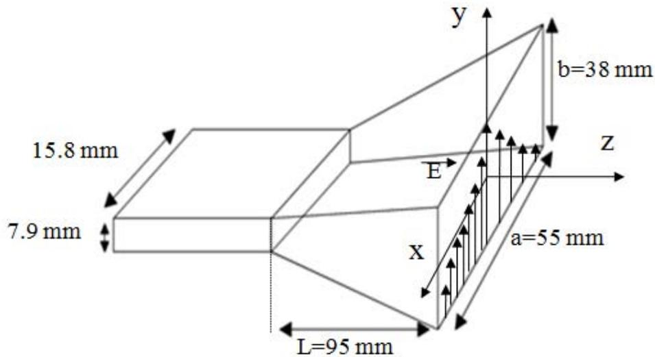
**Figure 6.16:** Dimension of the pyramidal horn along with its aperture field distribution (TE<sub>10</sub> mode)
