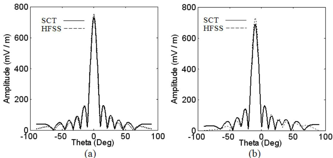
**Figure 6.13:** (a) E- plane radiation patterns of a  $8 \times 8$  uniform reflectarray of identical patches under normal plane wave incidence, both patterns are symmetrical (b) H-plane pattern of the same reflectarray under oblique incidence ( $\theta=10^\circ$ ), E-plane pattern is similar as shown in (a).
