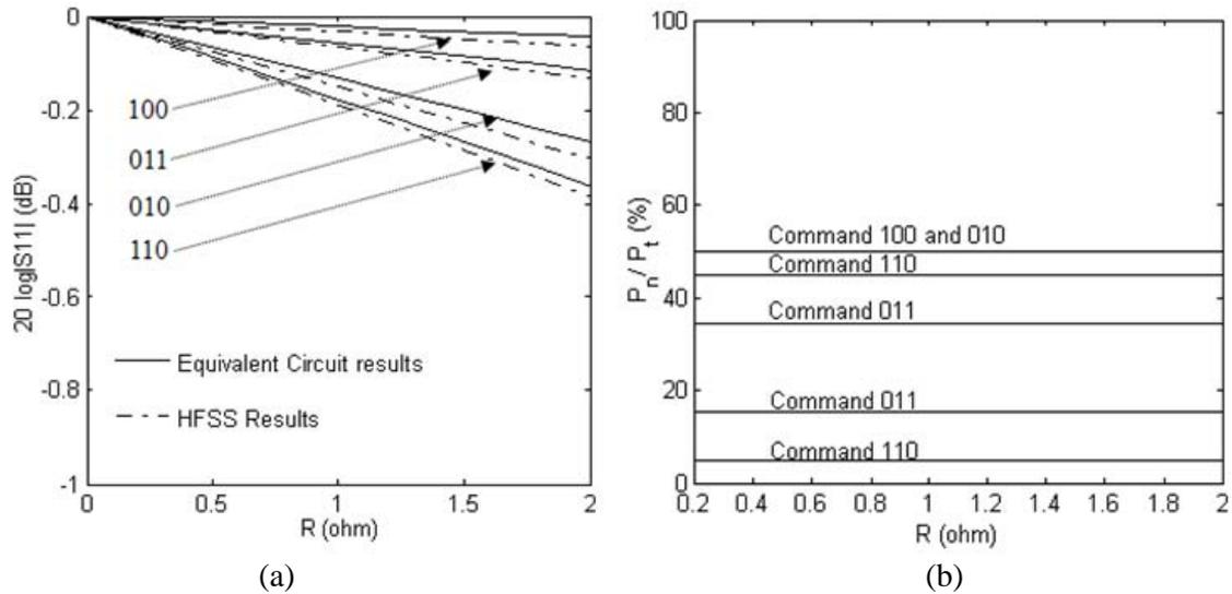
**Figure 3.3:** (a) Results obtained by the equivalent circuit and HFSS under double MEMS case (a) Comparison between Power loss results obtained by HFSS and equivalent circuit for the unit cell as a whole (b) Power dissipated within the ON-MEMS individually.
