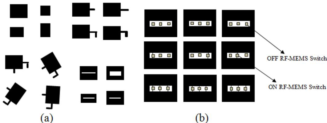
**Figure 1.4:** (a) Various approaches for phase tuning of the reflectarray. (b) Reflectarray implementation with RF-MEMS switches as phase tuning elements (all the reflectarray elements have similar physical structure and orientation)
