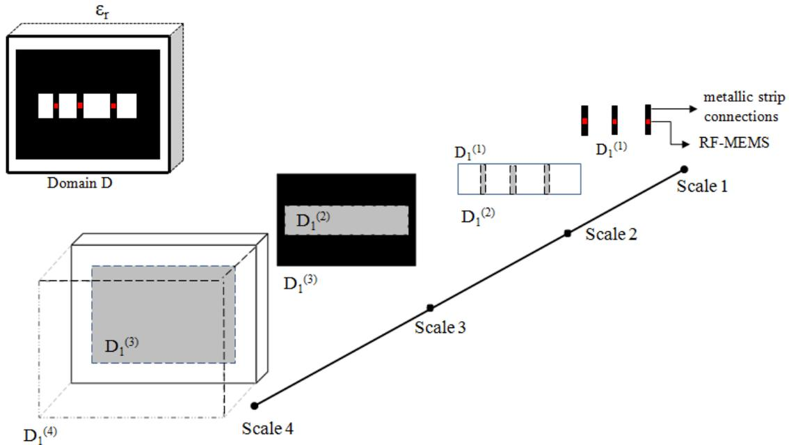
**Figure 6.24:** Partitioning of the discontinuity plane  $D$  of the active phase shifter cell in its constituent domains and sub-domains in four scales, white portions represent dielectric, black represents metal, grey parts represent un-partitioned sub-domains and red represents the RF- MEMS switch.
