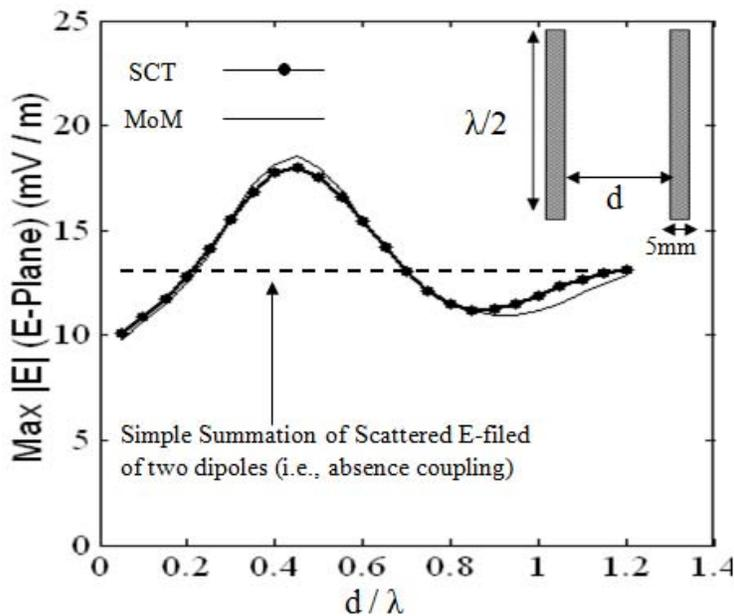
**Figure 6.5:** Characterization of mutual coupling for two dipole strips at 12.5GHz: E-plane backscattered electric field in the normal direction by two coupled half-wave printed dipoles with respect to the normalized separation between the dipoles when illuminating by a normally incident plane wave (polarized along the dipoles axis) at 12.5GHz.
