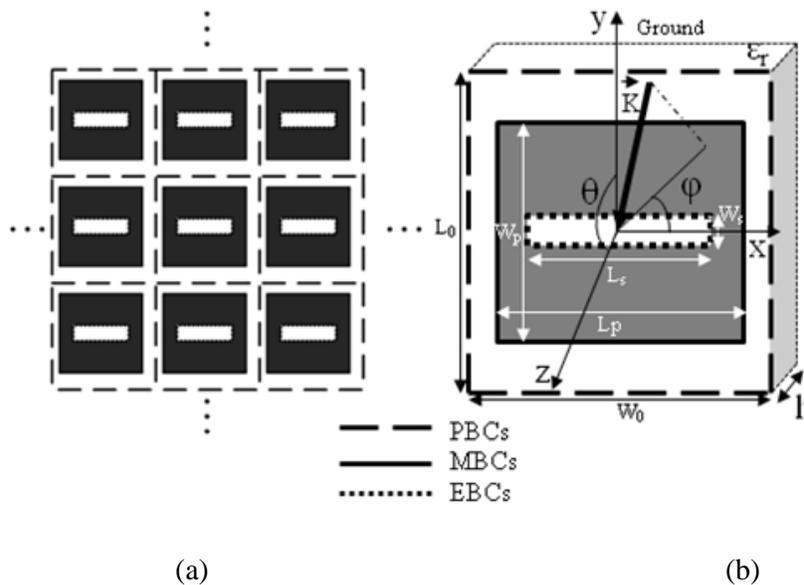
**Figure 5.1:** (a) A two dimensional periodic reflectarray (b) Enlarged unit-cell of the array with dimensions:  $L_0=W_0=15\text{mm}$ ,  $W_p=12\text{mm}$ ,  $L_s=1\text{mm}$ ,  $W_p$  and  $L_s$  are variable. Substrate thickness  $h=2.17\text{mm}$  ( $\epsilon_r=3.38$ ), PBCs, MBCs and EBCs stand for periodic, magnetic and electric boundary conditions respectively.
