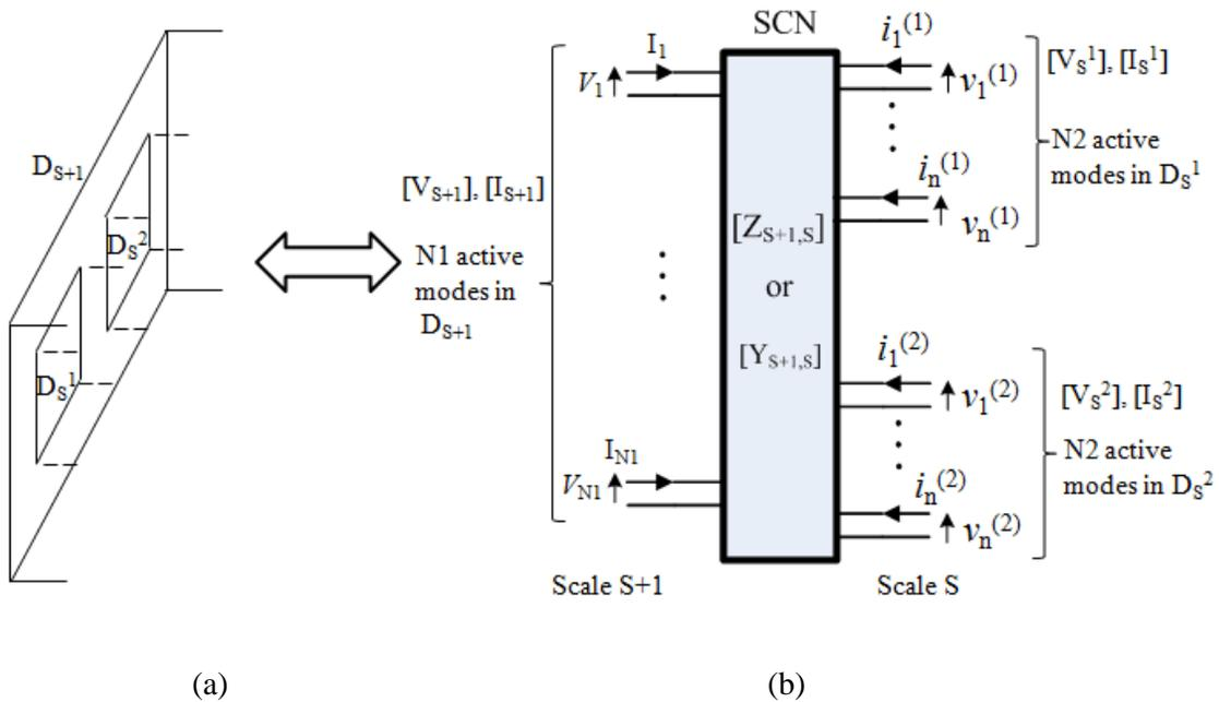
**Figure 6.1:** (a) Electromagnetic coupling between two adjacent unit-cell domains  $D_S^1$  and  $D_S^2$  modeled by a bifurcated waveguide. (b) Inter-modal coupling between parent domain  $D_{S+1}$  and daughter domains  $D_S^1$  and  $D_S^2$  can be represented by a bifurcation scale-changing network (SCN).
