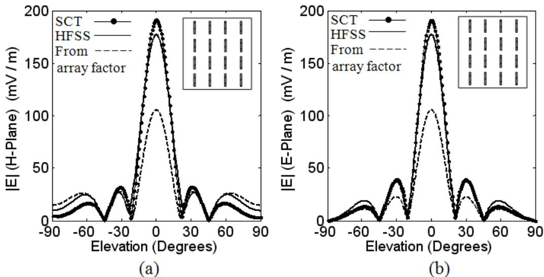
**Figure 6.6:** Far-field radiation pattern of a simple 4x4 dipole array in(a) H-plane and (b) E-plane when illuminating by a normally incident plane wave (polarized along the dipoles axis) at 12.5GHz.
