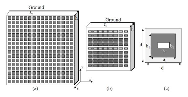
**Figure 6.11:** (a) A 256-cell (16 ×16) reflectarray geometry, unit cell and patch dimensions are the same as given in (c). (b) A 64-cell (8×8) reflectarray geometry with h=3.175mm,  $\epsilon_r$ =2.17. (c) An enlarged unit cell with d=16.8mm, a<sub>1</sub>=13.5mm, b<sub>1</sub>=13mm, a<sub>2</sub>=9mm and b<sub>2</sub>=6mm.
