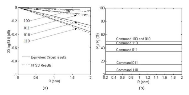
**Figure 3.3:** (a) Results obtained by the equivalent circuit and HFSS under double MEMS case (a) Comparison between Power loss results obtained by HFSS and equivalent circuit for the unit cell as a whole (b) Power dissipated within the ON-MEMS individually.
