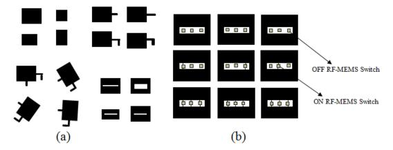
**Figure 1.4:** (a) Various approaches for phase tuning of the reflectarray. (b) Reflectarray implementation with RF-MEMS switches as phase tuning elements (all the reflectarray elements have similar physical structure and orientation)
