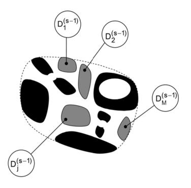
**Figure 4.2:** The i<sup>th</sup> generic domain resulting from the partition process at scale level S (black is metal, white is dielectric and grey indicates the location of sub-domains  $D_j^{(s-1)}$  (with j = 1, 2, ... M) [35].
