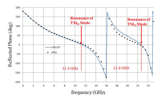
Figure 2.6: Comparison between the phases of the reflection coefficient obtained by equivalent circuit and HFSS
