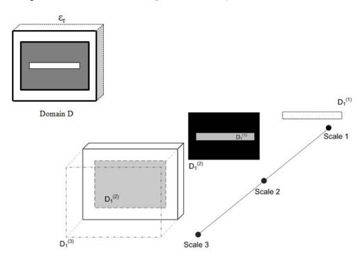
**Figure 5.2:** Partitioning the discontinuity plane D of the planar reflector in its constituent domains and sub-domains at three scales, white portions represent dielectric, black represents metal and grey parts are mere projections of the immediate sub-domains.
