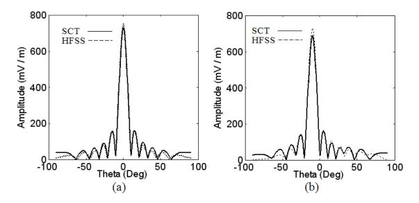
**Figure 6.13**: (a) E- plane radiation patterns of a  $8 \times 8$  uniform reflectarray of identical patches under normal plane wave incidence, both patterns are symmetrical (b) H-plane pattern of the same reflectarray under oblique incidence ( $\theta$ =10°), E-plane pattern is similar as shown in (a).
