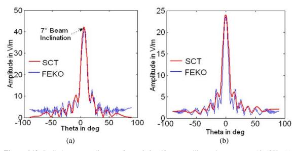
**Figure 6.19:** Radiation pattern diagrams for an 8x8 uniform metallic patch structure at 12.5GHz (a) E-Plane pattern (b) H-Plane pattern
