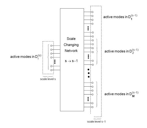
**Figure 4.3:** The Scale Changing Network coupling the active modes in the domain  $D_i^{(s)}$  (scale level s) and its constitutive sub-domains  $D_j^{(s-1)}$  (scale level s–1) [35].
