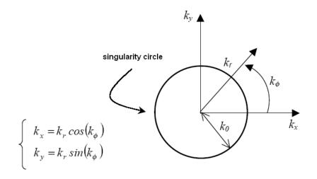
Figure 6.8: Wave-vector transformation from Cartesian to polar co-ordinates.
