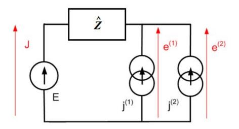
**Figure 6.3:** Simplified Equivalent circuit. Virtual source and the scale-changing source of each branch (when defined in the same domain and using same orthogonal modal-basis) can be replaced by a single current source.
