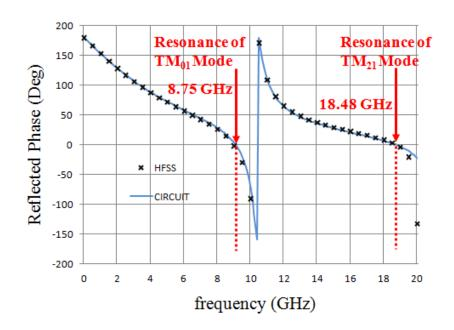
**Figure 2.8:** Comparison between the phases of the reflection coefficient obtained by equivalent circuit model of Figure 2.7(b) and HFSS
