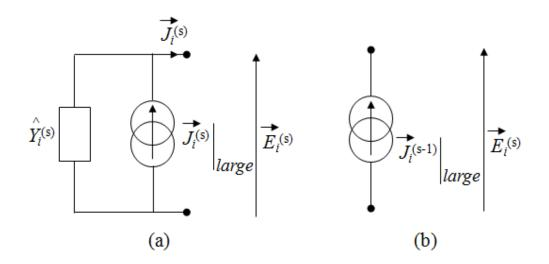
**Figure 4.6:** Symbolic representations of the current Scale Changing Sources: (a) In the domain  $D_i^{(s)}$  (scale level *S*); (b) In the sub-domain  $D_j^{(s-1)}$  (Scale level S-1). These sources allow deriving impedance matrix characterizing the Scale-Changing Network that models the electromagnetic coupling between the scale S and the scale S-1.
