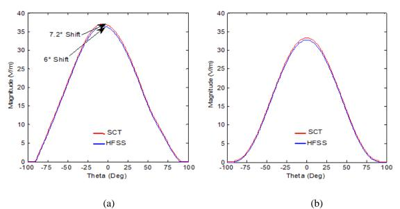
**Figure 5.10:** Scattered Electric Field in the far-field zone obtained from the SCT and HFSS under oblique incidence ( $\theta$ =20°,  $\varphi$ =0°) at 12.1 GHz (a) E-Plane (b) H-Plane
