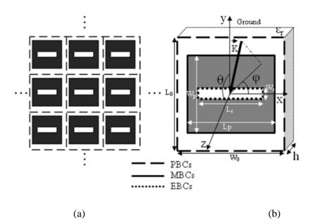
**Figure 5.1:** (a) A two dimensional periodic reflectarray (b) Enlarged unit-cell of the array with dimensions:  $L_0=W_0=15$ mm,  $W_p=12$ mm,  $L_s=1$ mm,  $W_p$  and  $L_s$  are variable. Substrate thickness h=2.17mm ( $\epsilon$ r=3.38), PBCs, MBCs and EBCs stand for periodic, magnetic and electric boundary conditions respectively.
