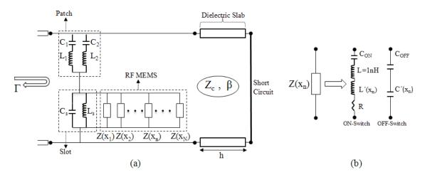
**Figure 3.1:** (a) Equivalent electrical circuit for the MEMS-controlled phase-shifter cell; (b) Equivalent circuit model of the  $n^{th}$  MEMS switch within the slot (the equivalent impedance Z depends on the ON/OFF state of the switch as well as its coordinate  $x_n$  inside the slot).
