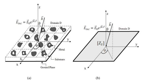
**Figure 6.7:** (a) An  $N \times N$  microstrip reflectarray of arbitrary cells under arbitrary plane wave incidence. (b) The surface impedance matrix  $[\mathbf{Z}_{S}]$  modeling the domain  $\mathbf{D}$ , this matrix is derived from the cascade of scale changing networks as shown in Figure 6.9.
