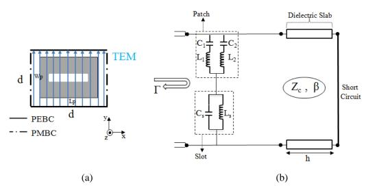
**Figure 2.7:** (a) Metallic Patch loaded with slot in  $d \times d$  waveguide excited by TEM wave (b) Its equivalent electrical circuit model.
