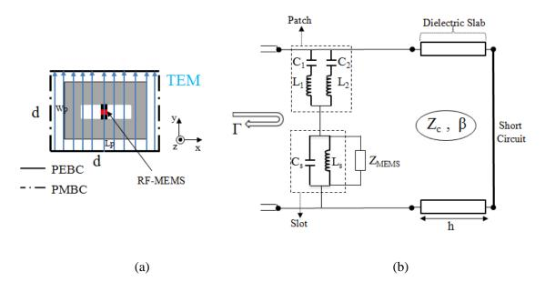
Section I: Chapter 2: Extraction of Equivalent Electrical Circuit Model for Reflectarray Phase Shifters
