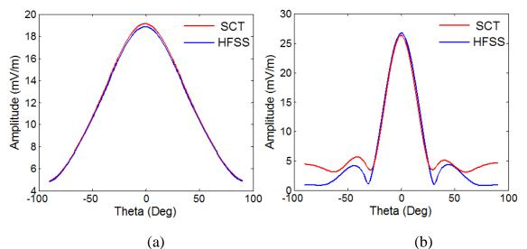
**Figure 6.25:** Radiation patterns of  $4\times1$  uniform reflectarray of Figure 18 keeping the electronic configuration (i.e., the switching states (ON/OFF) for the twelve RF-MEMS switches of four phase shifter cells) of the four phase shifter cells identical and hence obtaining both E and H plane patterns symmetrical (a) E- plane pattern (b) H-plane pattern
