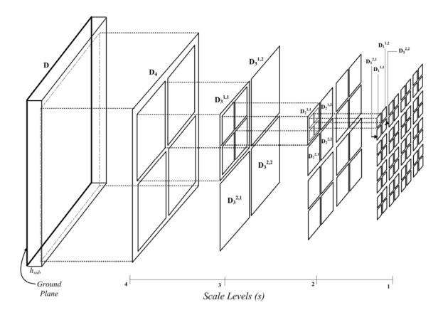
**Figure 6.9:** Partitioning of 64-cell array  $(8 \times 8)$ ; such hierarchical domain-decomposition allows defining the constitutive scale-levels and focusing rapidly on increasing fine details in the array.
