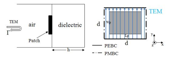
Figure 2.3: Simple Metallic Patch in d×d waveguide excited by TEM wave
