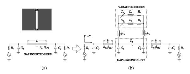
**Figure 2.1:** Equivalent circuit for predicting reflectarray cell scattering (a) Standard microstrip patch (b) Microstrip patch with varactor diode and discontinuities [10]
