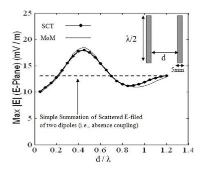
**Figure 6.5:** Characterization of mutual coupling for two dipole strips at 12.5GHz: E-plane backscattered electric field in the normal direction by two coupled half-wave printed dipoles with respect to the normalized separation between the dipoles when illuminating by a normally incident plane wave (polarized along the dipoles axis) at 12.5GHz.
