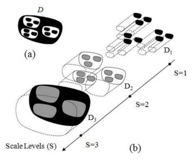
**Figure 4.1:** (a) An example of discontinuity plane presenting 3 scale-levels (black is metal and white is dielectric) (b) The scattered view of the various sub-domains at different scale levels generated by the partitioning process [35].
