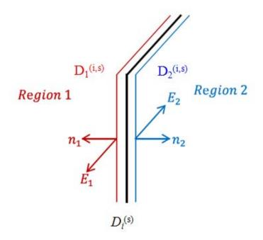
**Figure 4.5:** The discontinuity plane  $D_i^{(s)}$  along with two infinitely close parallel side-planes  $D_{\alpha}^{(i,s)}$  with  $\alpha = 1,2$  representing the two half-regions.
