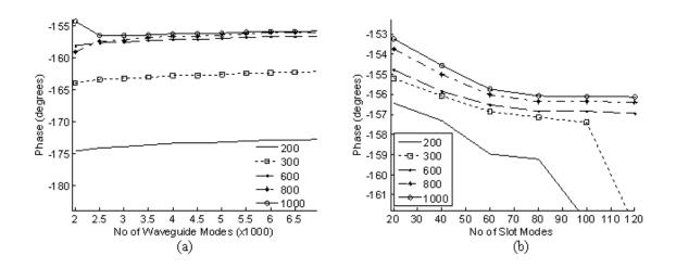
**Figure 5.8:** Convergence study of the phase of reflection coefficient for configuration 3 (Lp, Ws) => (8, 8), frequency 12.1GHz: (a) Convergence with respect to the number of modes in the periodic waveguide (legend indicates number of patch modes); (b) Convergence with respect to number of modes in the slot (legend indicates number of patch modes).
