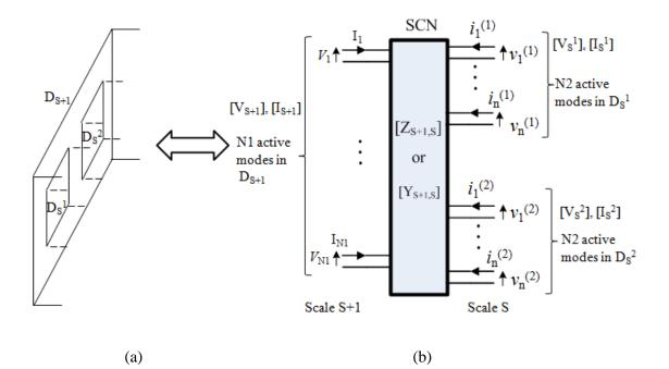
**Figure 6.1:** (a) Electromagnetic coupling between two adjacent unit-cell domains  $D_S^1$  and  $D_S^2$  modeled by a bifurcated waveguide. (b) Inter-modal coupling between parent domain  $D_{S+1}$  and daughter domains  $D_S^1$  and  $D_S^2$  can be represented by a bifurcation scale-changing network (SCN).
