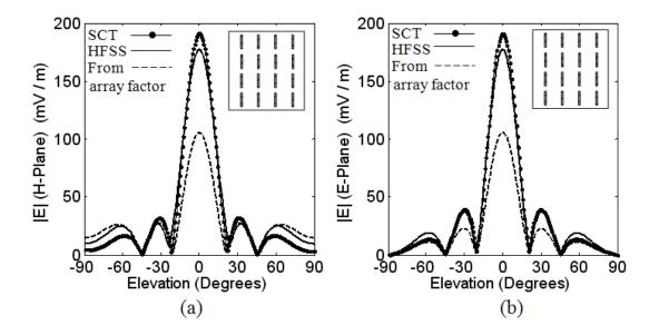
**Figure 6.6:** Far-field radiation pattern of a simple  $4 \times 4$  dipole array in(a) H-plane and (b) E-plane when illuminating by a normally incident plane wave (polarized along the dipoles axis) at 12.5GHz.
