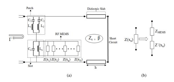
**Figure 2.12:** (a) Equivalent electrical circuit for a phase-shifter cell comprising of N MEMS; (b) Equivalent circuit model of the n<sup>th</sup> MEMS within the slot (the total impedance  $Z_{MEMS}+Z'$  depends on the ON/OFF state of the switch as well as its coordinate  $x_n$  inside the slot).
