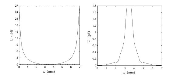
Figure 2.11: Variations of (a) inductance L' and (b) capacitance C' versus position of a single MEMS switch in the slot.
