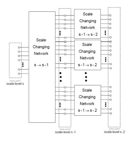
**Figure 4.4:** The cascade of Scale Changing Networks allows relating the transverse electromagnetic field at scale level S to that of at scale level S–2 [35].
