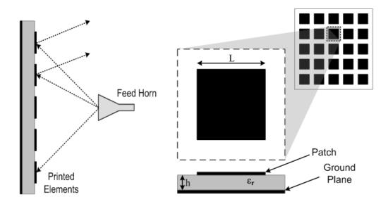
Figure 1.2: A standard microstrip reflectarray antenna
