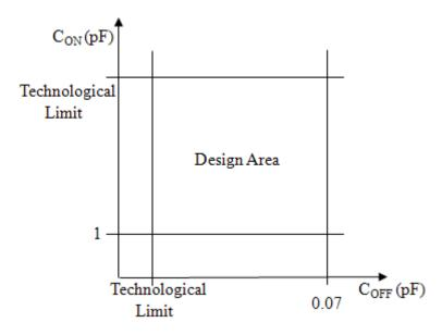
Figure 3.5: Graph for the phase shifter cell showing the design limits on the basis of C<sub>ON</sub> and C<sub>OFF</sub>.
