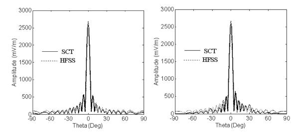
**Figure 6.12**: (a) E- plane and (b) H-plane radiation patterns of a 16×16 uniform patch-slot reflectarray (see caption of Figure 6.10(c) for the dimensions of the structure)
