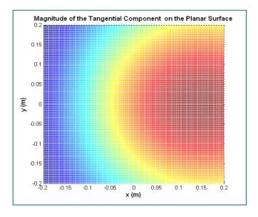
**Figure B.5:** Tangential field pattern of a horn antenna placed at an offset of 200mm from the center of the surface with an angle of inclination equal to 30°. d=660mm
