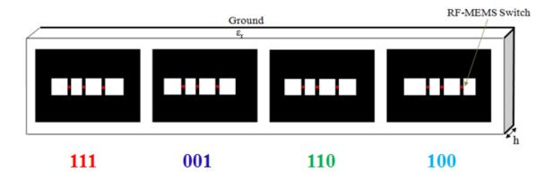
**Figure 6.23:** A 4-cell (4x1) reconfigurable reflectarray, all the dimensions are the same as given in Figure 1 of Chapter 2.
