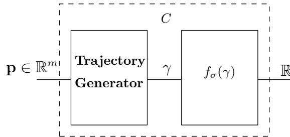
Fig. 3.2: The mapping to approximate. The Trajectory Generator takes in input a vector of parameters defining a step, and must return a *unique* trajectory. The value returned by the mapping is positive if the trajectory is acceptable (feasible), negative otherwise.
