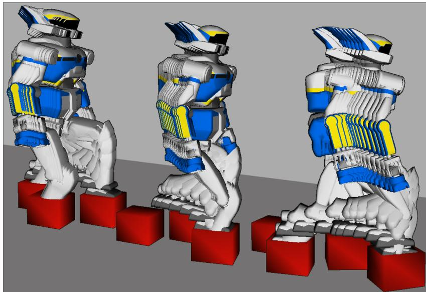
Fig. 6.14: A sequence of (raw) steps performed by HRP-2, with the corresponding configurations of the lower boxes. The feet of the robot always leave and enter the rectangular boxes from above, not from the sides. Thus, for all the obstacles whose height is less than  $h_m$ , the lower boxes can be used for conservative collision checks.
