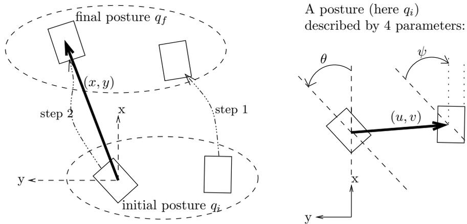
Fig. 2.2: (Left) The sequence of two steps from posture  $q_i$  to  $q_f$ , with translation parameters  $(x, y)$ . (Right) A posture is fully described by the absolute orientation of the left foot, and the relative position and orientation of the right foot.
