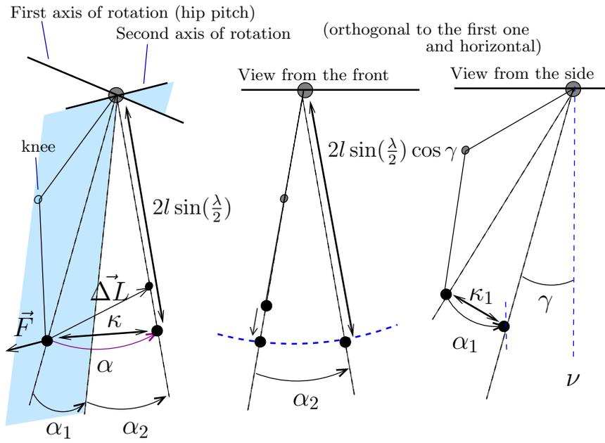
Fig. E.1: The two first rotations, to obtain the correct *hip joint - ankle joint* axis. Here “front” means that we watch the leg so that the hip, knee and ankle are aligned; the “view from the side” is orthogonal to the view from the front.
