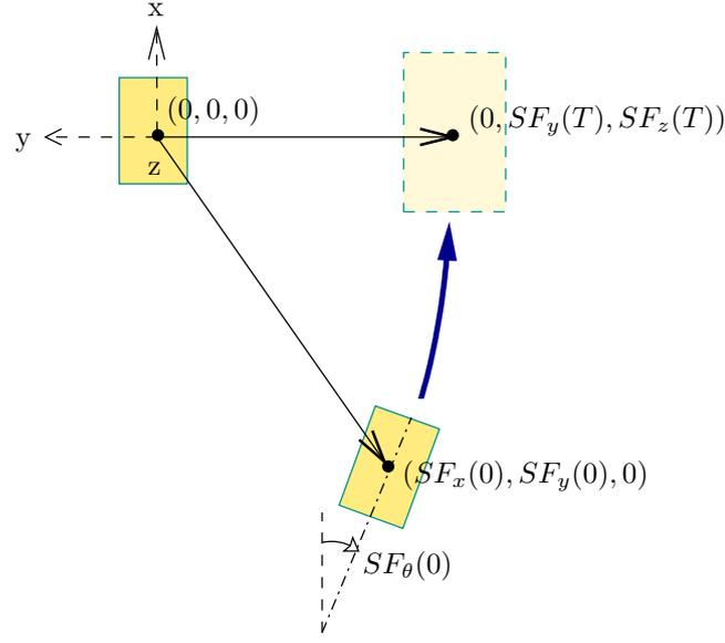
Fig. 4.1: Here we show an upward half-step from above. It is fully determined by the 5 parameters  $SF_x(0)$ ,  $SF_y(0)$ ,  $SF_\theta(0)$ ,  $SF_y(T)$  and  $SF_z(T)$ . A downward half-step is also fully determined by 5 parameters.
