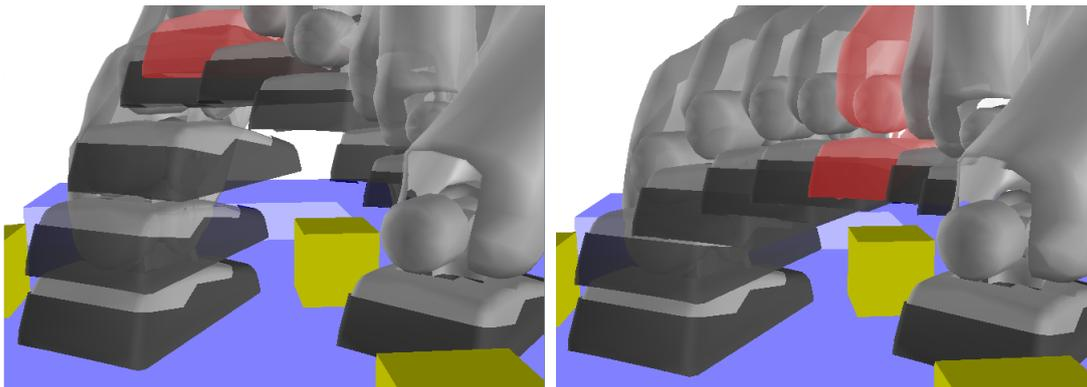
Fig. 4.6: *On the left*: a raw sequence of two half-steps avoiding a box on the ground. We can see that the swing foot reaches an unnecessarily high position. After smoothing (*on the right*), the trajectory has been modified so that the foot moves very close to the obstacle.
