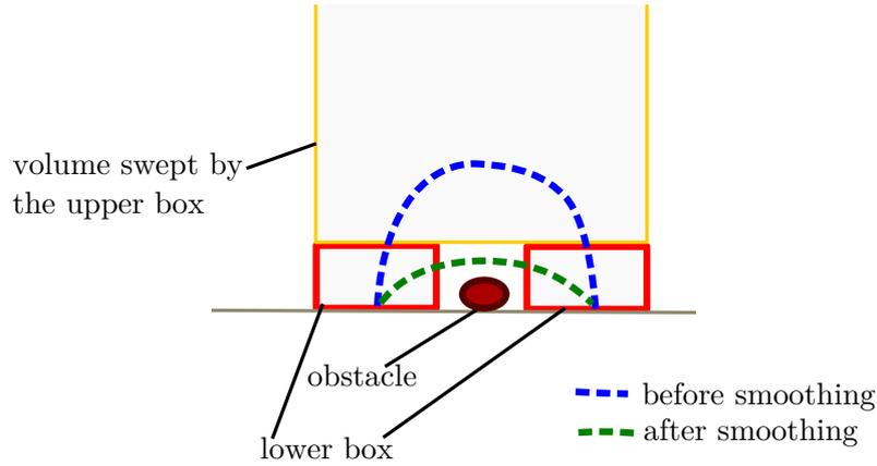
Fig. 6.15: Swing foot trajectory before and after smoothing. We can see that after the smoothing the robot trajectory is not necessarily contained in the boxes anymore.
