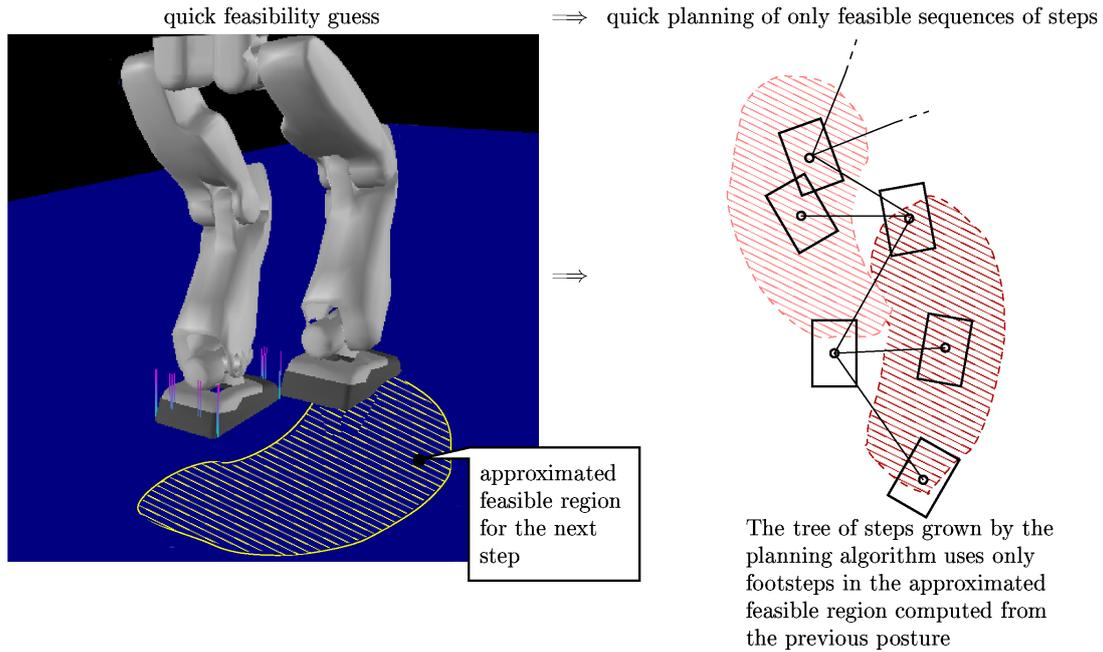
Fig. 3.1: From quick feasibility guess to fast and safe footsteps planning.
