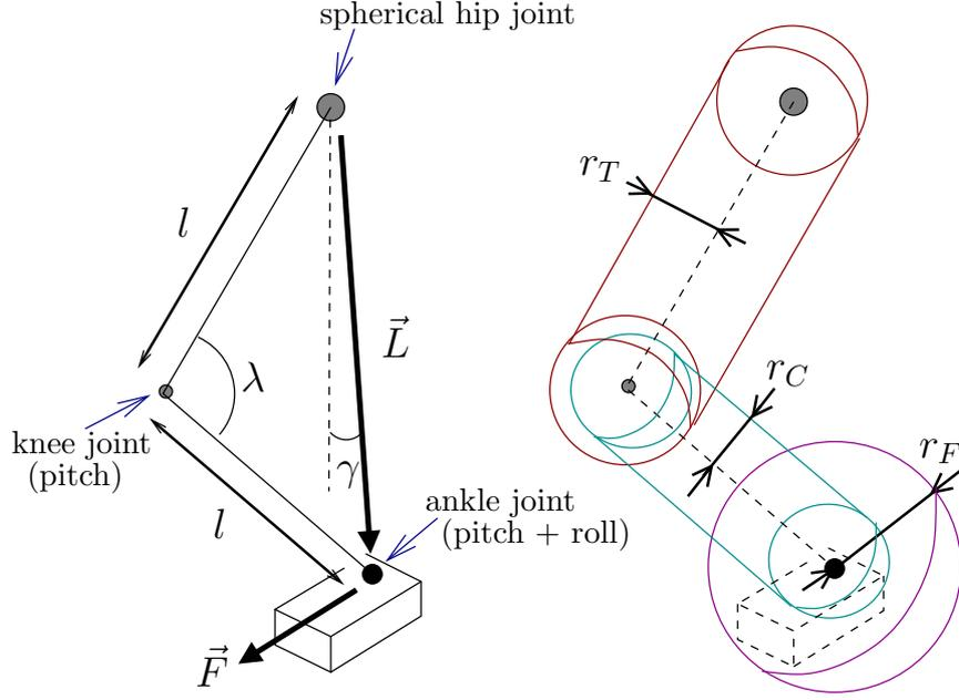
Fig. 4.8: A simple 6-DOF robot leg.
