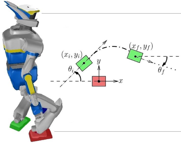
Fig. 3.5: Parameterization of a step for the humanoid robot HRP-2. The right foot defines the origin of the coordinate frame, and the left foot moves from  $(x_i, y_i, \theta_i)$  to  $(x_f, y_f, \theta_f)$ . The robot has 36 degree of freedom. 6 for the waist position and orientation (the “free-flyer”), and 30 revolute joints.
