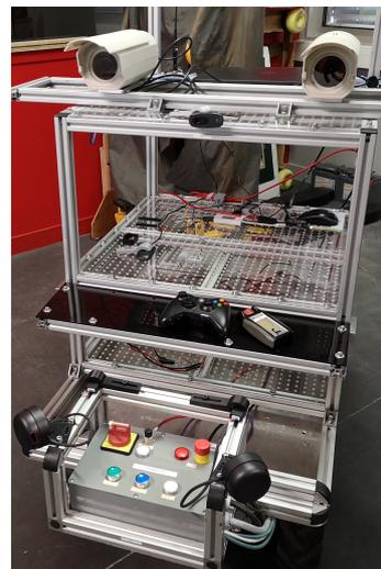
Figure 3.17: Robotic mobile driving platform with two stereoscopic event-based cameras mounted on top.
