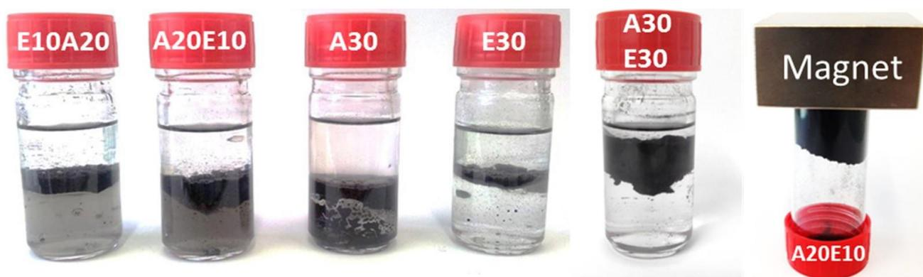
**Figure 6.4:** Photographs of water/toluene biphasic systems with **E30**, **A30**, **A20E10**, **E10A20**, and a physical mixture of **A30** (50%, w/w) and **E30** (50%, w/w); and magnetic amphiphilic **A20E10** powder.
