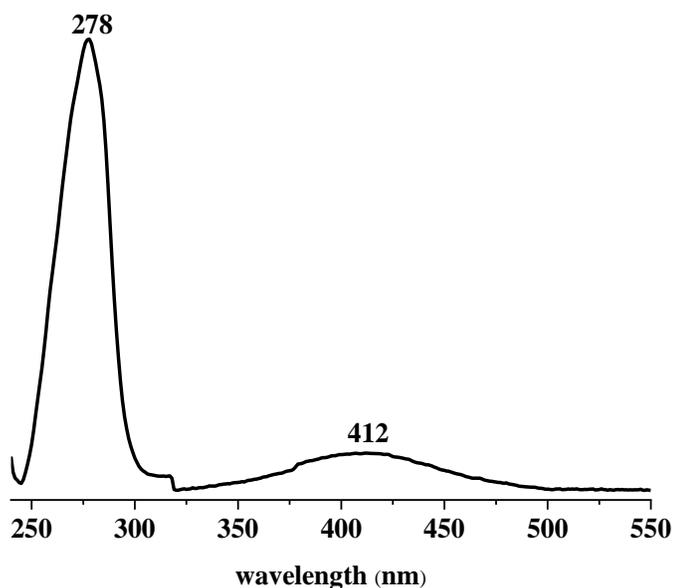
**Fig. 4.24:** UV/vis spectrum of labeled complex I E108C<sup>M</sup> variant. The peak at 278 nm is assigned to complex I, the one at 412 nm belongs to the released TNB<sup>-</sup> which is produced after treating complex I with KCN.
