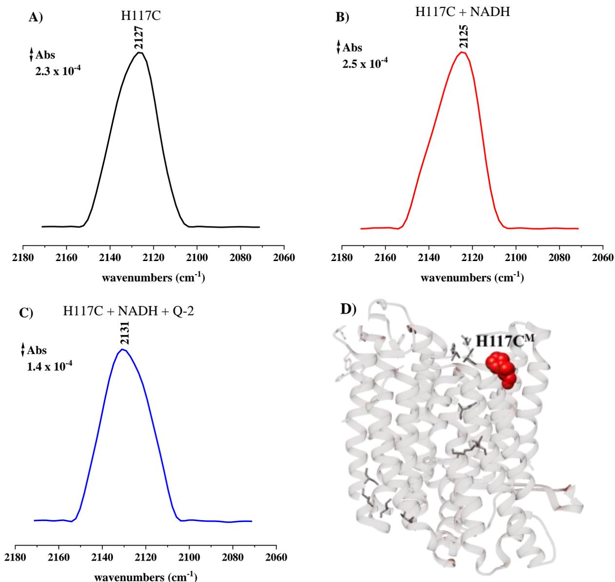
**Figure 4.38:** Spectra of the SCN bands of oxidized H117C<sup>M</sup> (A, black), after reduction with 100 μM NADH (B, red) and re-oxidation with 150 μM Q-2 (C, blue). D) Position of the H117C<sup>M</sup> residue in the NuO<sub>M</sub> structure.
