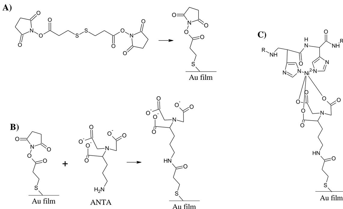
**Figure 4.27: Reactions to build the Ni-NTA-SAM surface.** A) Self-assembly of TSP on the gold monolayer; B) reaction of ANTA with TSP on the gold layer; C) complexation of Ni<sup>2+</sup> on ANTA-TSP gold layer [263].
