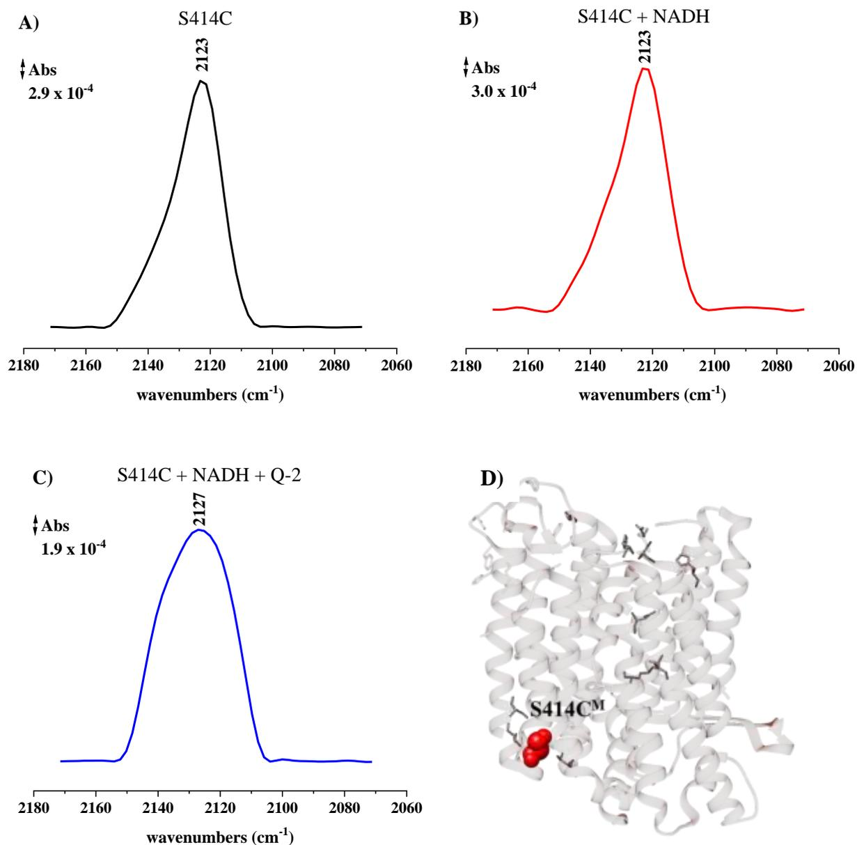
**Figure 4.44:** Spectra of the SCN bands of oxidized S414C<sup>M</sup> (A, black), after reduction with 100  $\mu$ M NADH (B, red) and re-oxidization with 150  $\mu$ M Q<sub>2</sub> (C, blue). D) Position of the S414C<sup>M</sup> residue in the NuoM structure.
