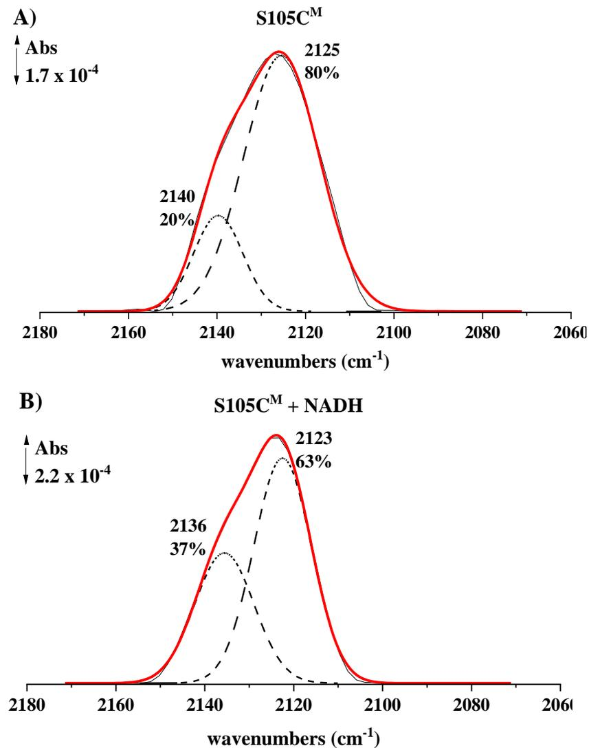
**Figure 4.35:** Deconvolution of the nitrile band obtained for the NuoM S105C<sup>M</sup> variant (A); after reduction by NADH (B).
