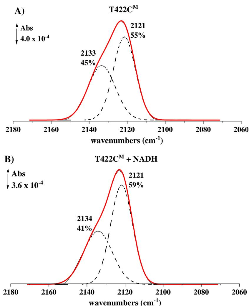
Figure 4.47: Deconvolution of the nitrile band T422C<sup>M</sup> variant (A) and after reduction with NADH (B).
