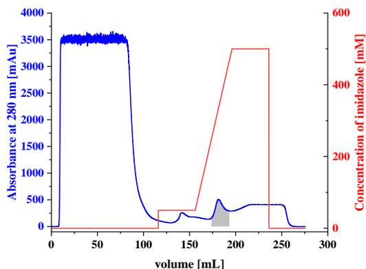
**Figure 4.65: Elution profile of HisTrap affinity chromatography to purify the E107D<sup>A</sup> variant.** Absorbance at 280 nm is shown in blue, concentration of imidazole in red. The fractions that normally include the oxidase are shown in grey area.
