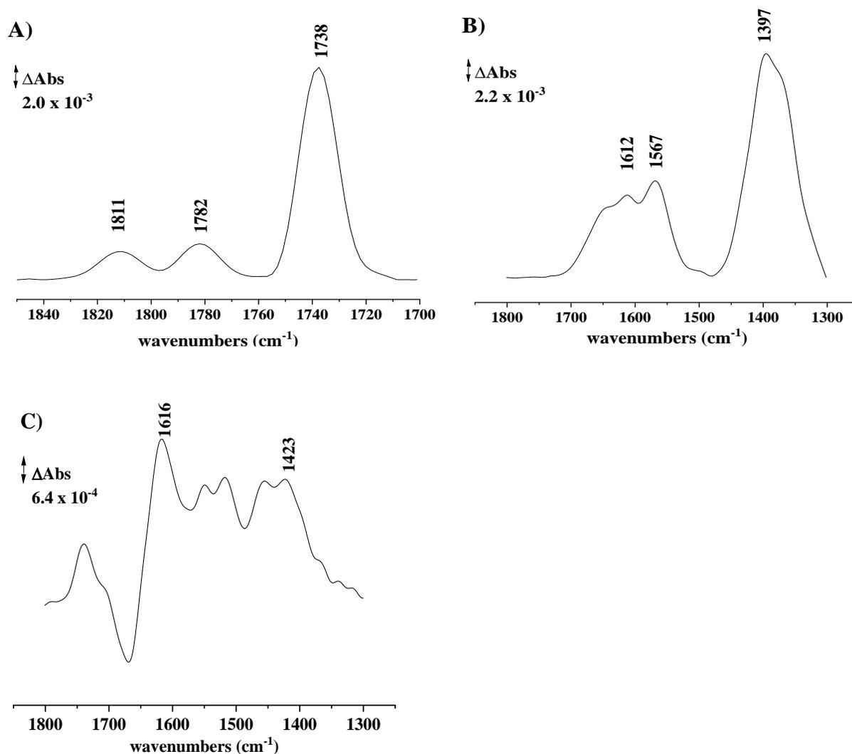
**Figure 4.28: ATR-FTIR spectra following of the crystal surface modification steps.** A) Self-assembly of the TSP monolayer on the bare Au surface (reference spectrum: gold layer covered with DMSO), B) cross-linking of ANTA with TSP monolayer (reference spectrum: DTSP SAM in water), C) complexation of  $\text{Ni}^{2+}$  by NTA (TSP-NTA SAM covered with water).
