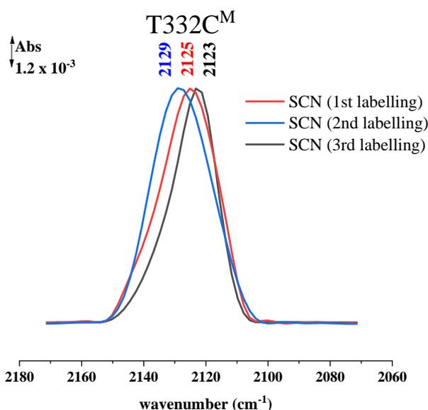
**Figure 4.33: Position of the thiocyanate band after labelling the T332C<sup>M</sup> variant several times.** 1<sup>st</sup> labelling (red), 2<sup>nd</sup> labelling (blue), 3<sup>rd</sup> labelling (black).
