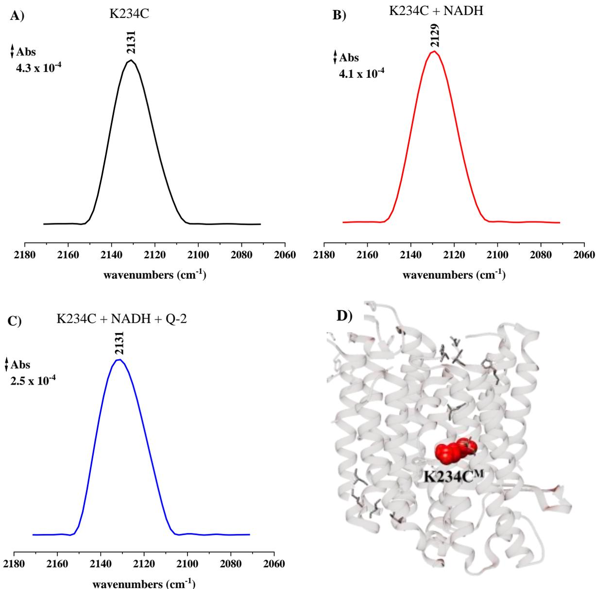
**Figure 4.51: Spectra of the SCN bands of oxidized K234C<sup>M</sup> (A, black), after reduction with 100  $\mu$ M NADH (B, red) and re-oxidation with 150  $\mu$ M Q-2 (C, blue). D) Position of the K234C<sup>M</sup> residue in the NuO structure.**
