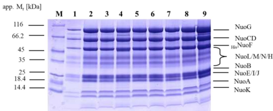
**Figure 4.13: SDS-PAGE of preparations of complex I and its variants.** The lane M belongs to the *unstained protein marker* (Thermo Fischer Scientific). Lanes are assigned as follows: complex I (1), NuoM S105C (2), NuoM H117C (3), NuoM T422C (4), NuoM S425C (5), NuoM T178C (6), NuoM K234C (7) and NuoM D258C (8), complex I (9, in higher concentration).
