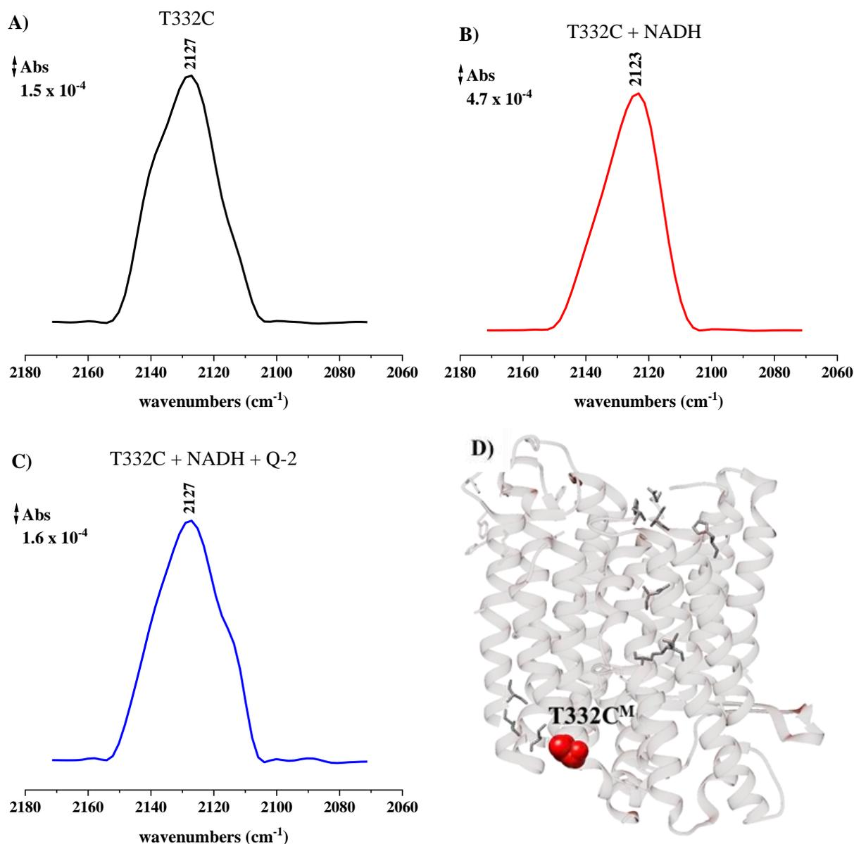
**Figure 4.42:** Spectra of the SCN bands of oxidized T332C<sup>M</sup> (A, black), after reduction with 100 μM NADH (B, red) and after re-oxidation with 150 μM Q-2 (C, blue). D) Position of the T332C<sup>M</sup> residue in the NuoM structure.
