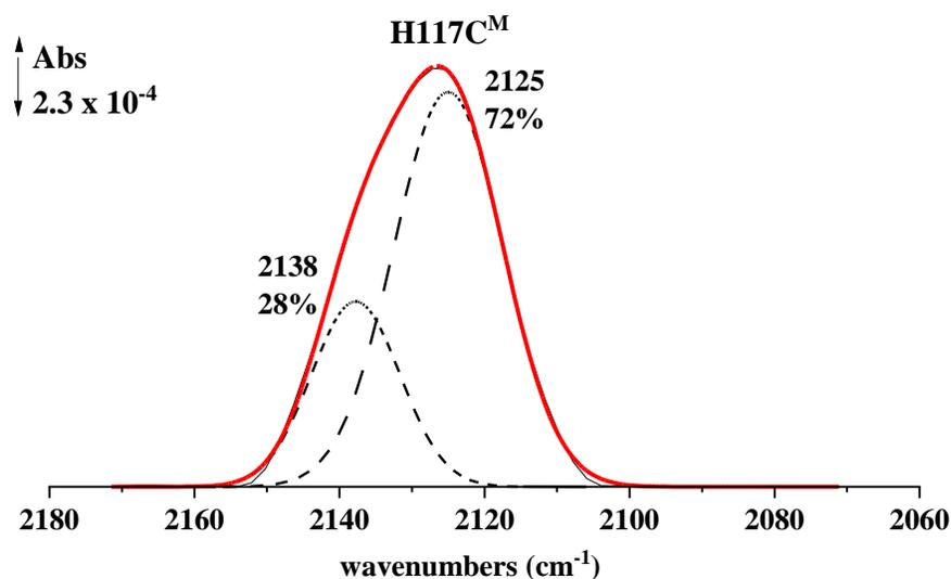
**Figure 4.39: Deconvolution of the nitrile band of the H117C<sup>M</sup> variant.**
