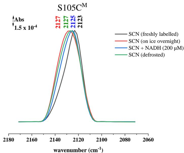
**Figure 4.31:** Position of the nitrile band observed with the S105C<sup>M</sup> variant after immediate labelling (black); after leaving the labelled sample overnight (red), after freezing and thawing the sample (green), and after addition of a higher substrate concentration (blue).
