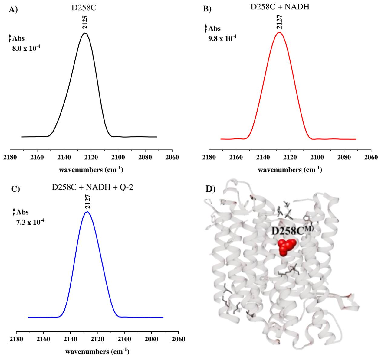
**Figure 4.52:** Spectra of the SCN bands of the oxidized D258C<sup>M</sup> (A, black), after reduction with 100  $\mu$ M NADH (B, red) and re-oxidation with 150  $\mu$ M Q-2 (C, blue). D) Position of the D258C<sup>M</sup> residue in the Nuom structure.
