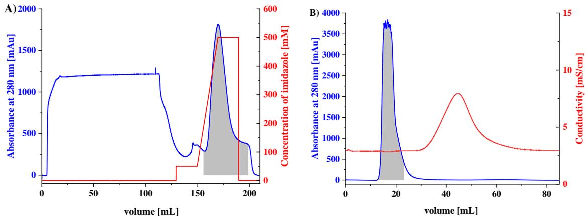
**Figure 4.63: Elution profile of HisTrap affinity chromatography (A) and HiTrap Desalting column (B).** A) Absorbance at 280 nm is shown in blue, concentration of imidazole in red. B) Absorbance at 280 nm is depicted in blue, conductivity is shown in red. The pooled fractions are indicated by the grey area.
