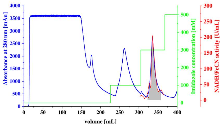
**Figure 4.10: Elution profile of the Ni<sup>2+</sup> affinity chromatography.** The absorbance at 280 nm is shown in blue; the imidazole concentration in green. The NADH/ferricyanide activity is shown in red. Fractions that were pooled and concentrated are shown in grey.
