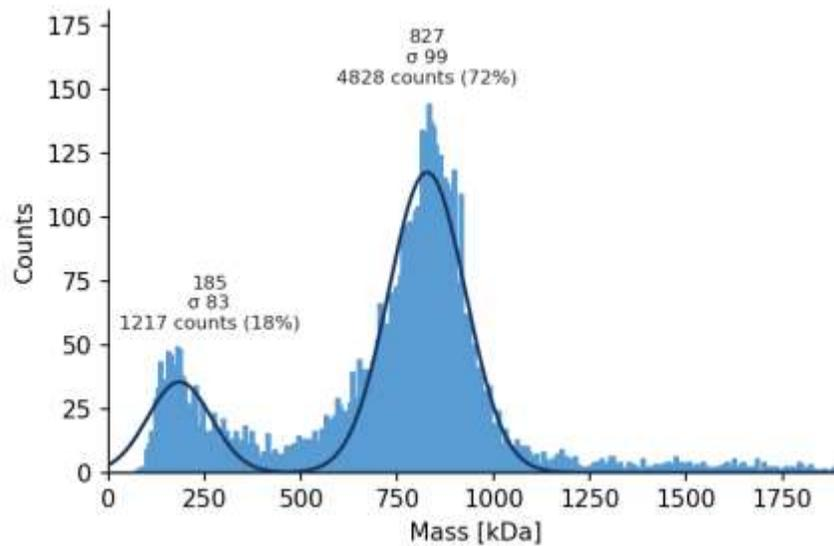
**Figure 4.15: Mass distribution of the T332C<sup>M</sup> variant.** Scatter plots of the binding events with corresponding Gaussian adjustments are shown. The protein sample was diluted to 50 nM. The mass is given in kDa, binding events and percentages are given.
