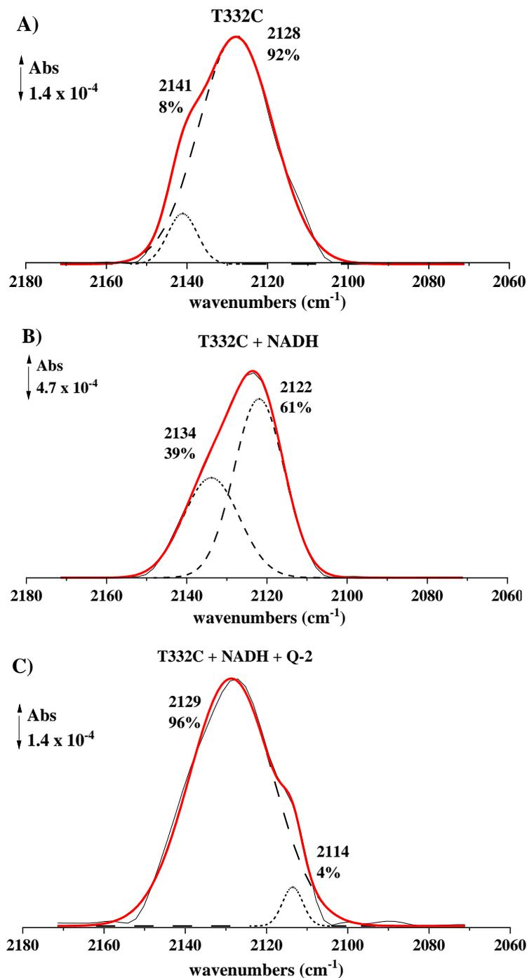
**Figure 4.43: Deconvolution of the nitrile band of the T332C<sup>M</sup> variant (A), after reduction by NADH (B) and after re-oxidation by Q-2 (C).**
