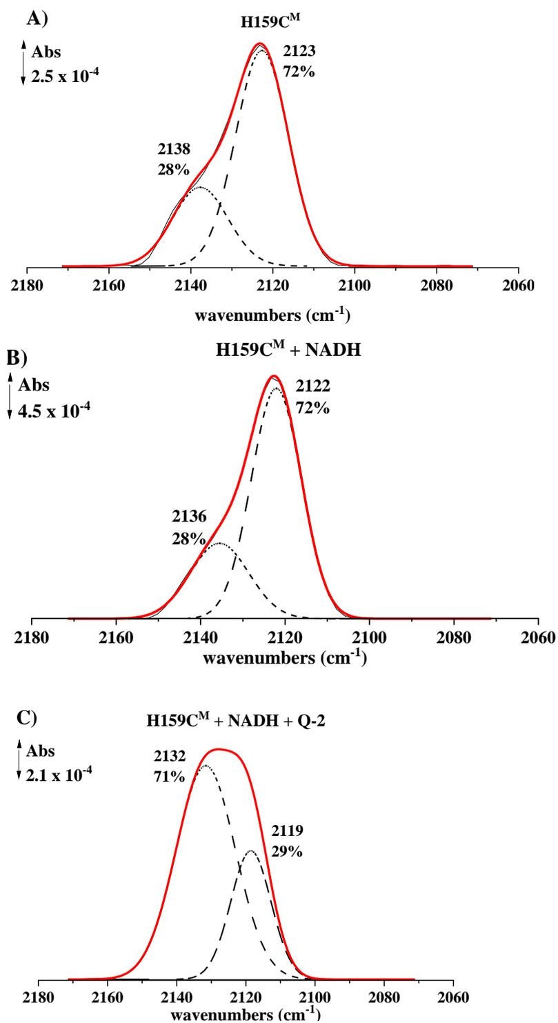
Figure 4.41: Deconvolution of the nitrile band of the H159C<sup>M</sup> variant (A), after reduction with NADH (B) and after re-oxidation with Q-2 (C).
