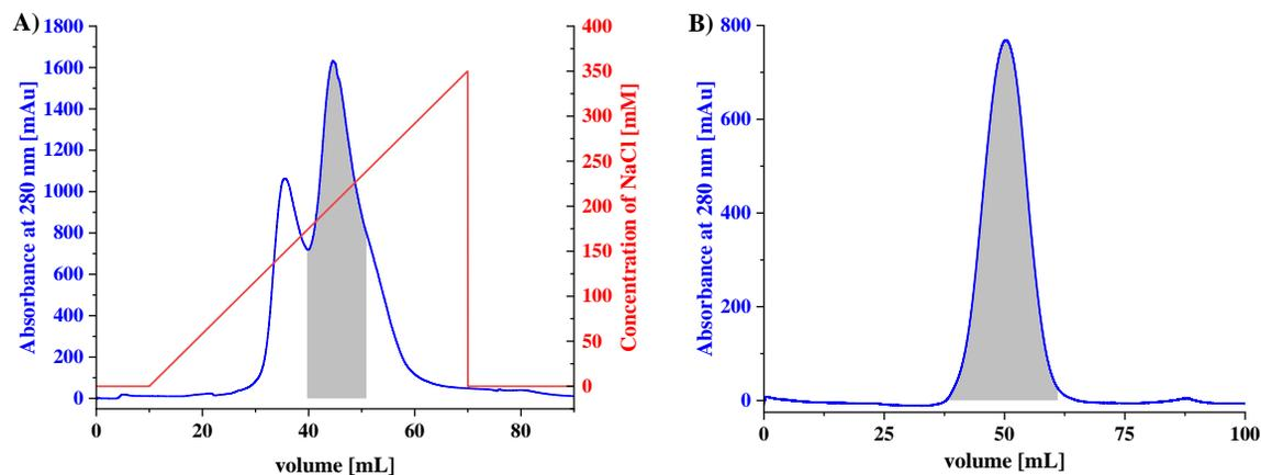
**Figure 4.64: Elution profile of MonoQion exchange chromatography (A) and S300 size exclusion column (B).** A) Absorbance at 280 nm is shown in blue, concentration of NaCl in red. B) Absorbance at 280 nm [mAu] is depicted in blue. The pooled fractions are indicated by the grey area.
