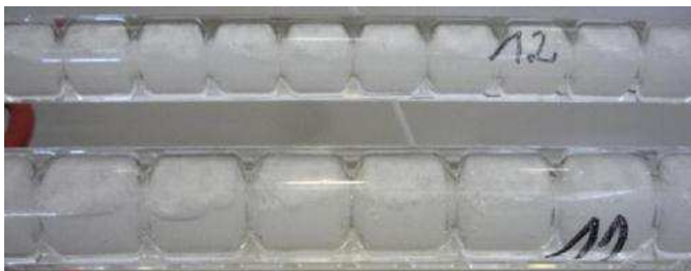
Figure VI- 11 : zoom on two sections – observation of the encrusting
