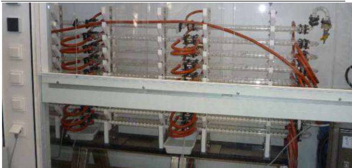
Figure IV- 31 : Continuous oscillatory baffle reactor COBR , general configuration
