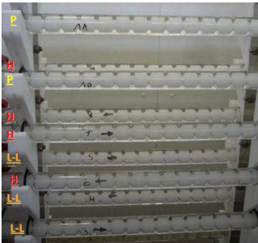
Figure VI- 10 : overview of the column in course of polymerization, L-L means liquid-liquid dispersion, H corresponds to the start of the reaction (heating zone) and P at the polymerization continuation
