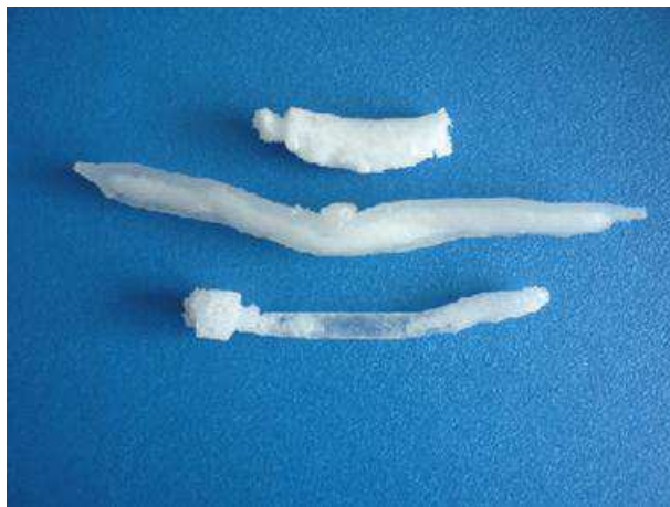
Figure VI- 4: polymer block resulting from the encrusting of the COBR
