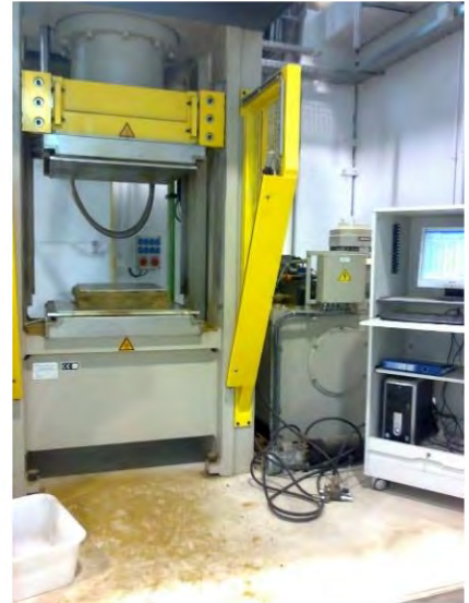
Figure A.VI-1 : Thermopresse hydraulique PEI 400T
