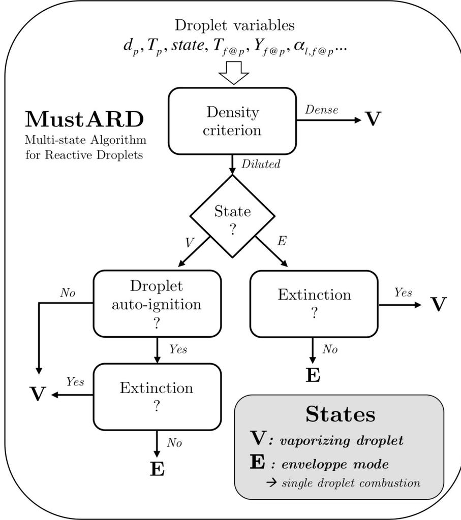
**Figure 8.14** : Scheme of the proposed multi-state droplet combustion algorithm, *MuStARD*.
