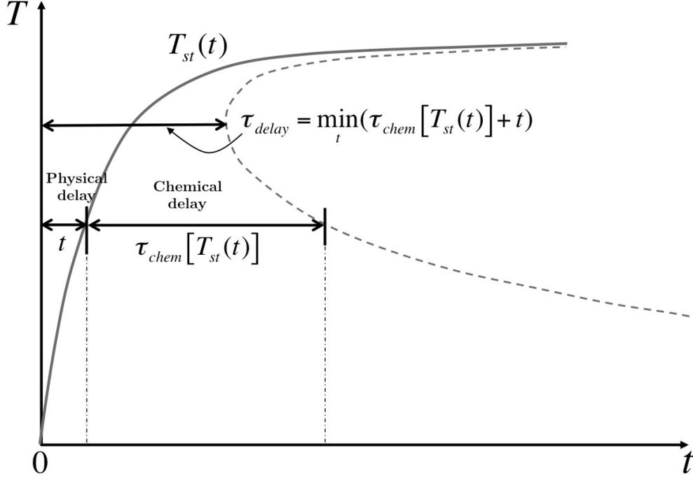
**Figure 8.17** : Evolution of the temperature at the stoichiometric point, for a droplet in a steady environment. The auto-ignition delay of the stoichiometric mixture  $\tau_{chem}$  is computed for each  $T_{st}(t)$ . the auto-ignition delay of the droplet corresponds to the minimum of  $t + \tau_{chem}(T_{st}(t))$ .
