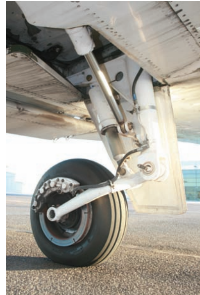
Figure 2.1: Main landing gear of a Cessna 404 Titan.
