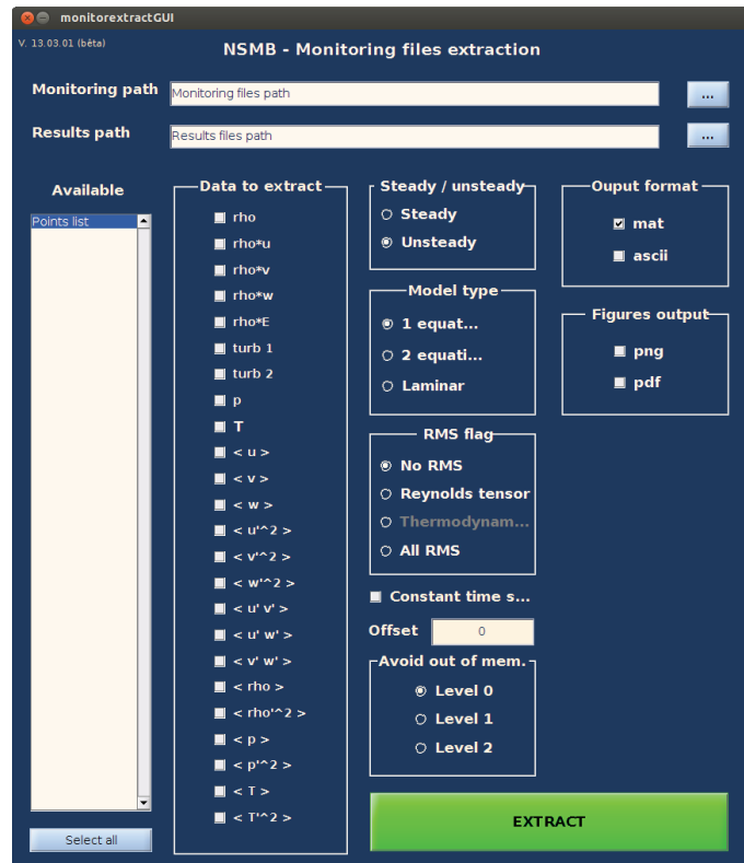
Figure D.1: Matlab graphical user interface of the programme to extract data from NSMB monitoring files.
