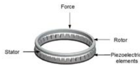
(a) Inchworm motor principle [23] (b) Ultrasonic rotary motor [27] (c) Inertial type stick and slip motor [3]
