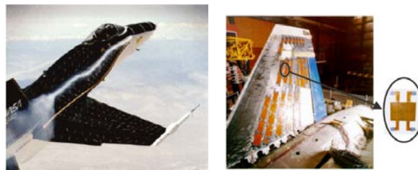
(a) F/A-18 with vortices generated at high angles of attack (b) piezoelectric actuators placed on the fin of a F/A-18
