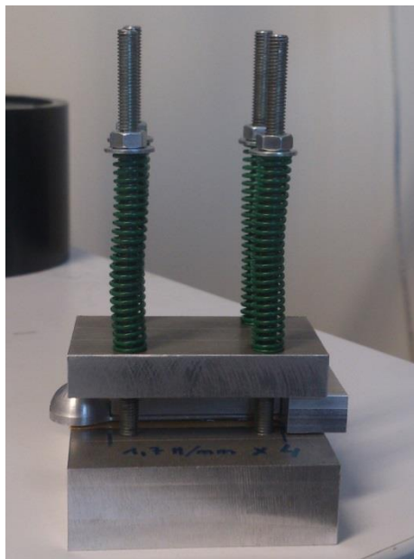
Figure 3.15 Application of evenly distributed pressure during the gluing process of the active and passive layers
