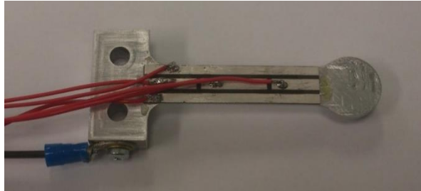
Figure 3.16 Completed prototype unimorph transducer “II”
