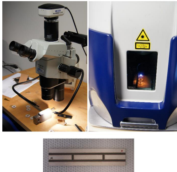
Figure 3.13 Sectorization process: upper right – laser cutting system; upper left – inspection of the depth of the cut; lower – sectorized ceramic
