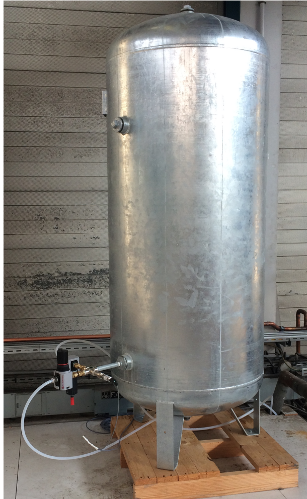
Figure 2.9: Buffer tank used at the inlet of the turbulent tuning gas line
