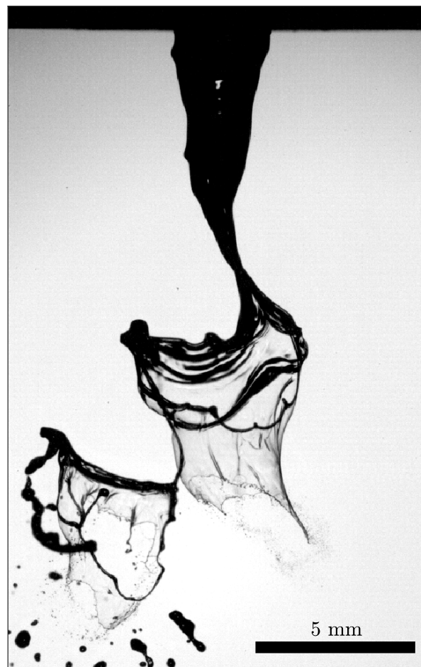
Figure 2.11: Snapshot of the atomization process captured using back-lit imaging, U_l = 0.41 m/s, U_g = 30 m/s, Re_l = 770 and We_g = 27 .
