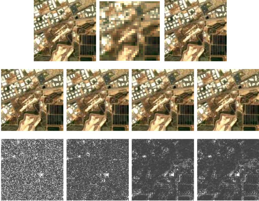
Figure B.1: Fusion results. (Top 1) Reference image. (Top 2) HS image. (Top 3) MS image. (Middle 1) MAP [HEW04]. (Middle 2) Wavelet MAP [ZDBS09]. (Middle 3) MCMC with known  $\mathbf{R}$ . (Middle 4) MCMC with unknown  $\mathbf{R}$ . (Bottom 1-4) The corresponding RMSE maps.
