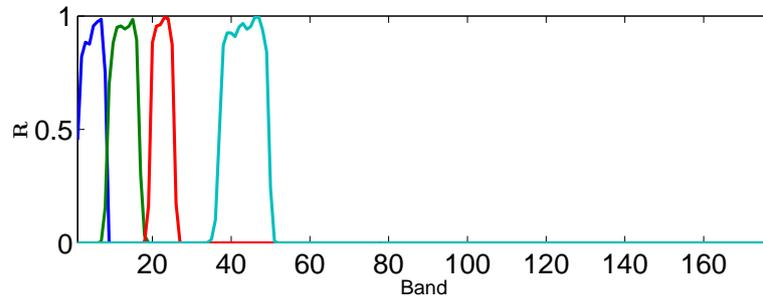
Figure 2.9: LANDSAT-like spectral responses (4 bands in MS image).
