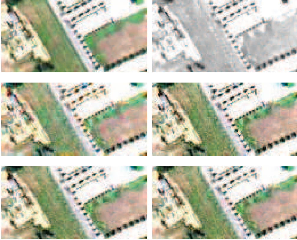
Figure 1.7: ROSIS dataset: (Top left) Reference image. (Top right) PAN image. (Middle left) Adaptive IHS [RSM + 10]. (Middle right) MAP [HEW04]. (Bottom left) Wavelet MAP [ZDBS09]. (Bottom right) MCMC.
