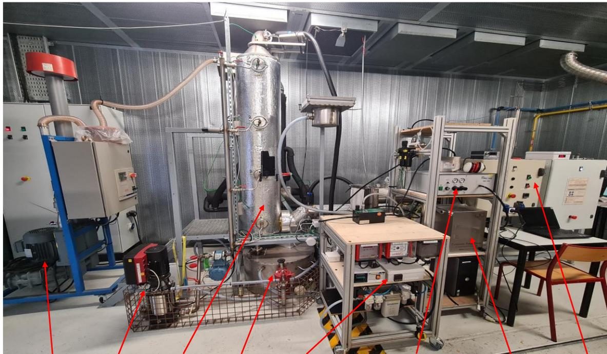
Centrifugal fan    Water pump    Spray scrubber    Water tank    Dilution system    Particle generator (DNP 2000 – Palas)    Particle counter (SMPS)    Heating system
