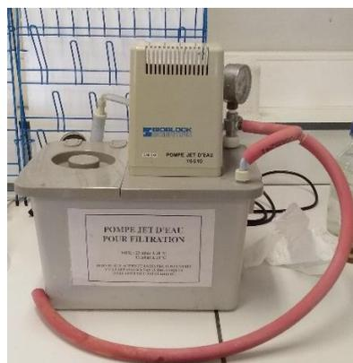
*Figure 33 Particle/liquid vacuum filtration apparatus*
