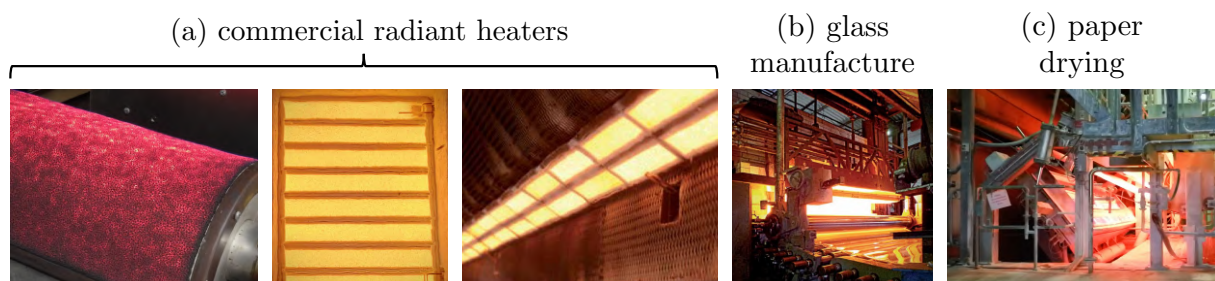
Figure 1.7. – From [59–61]: examples of commercial and industrial solutions based upon porous media combustion.
